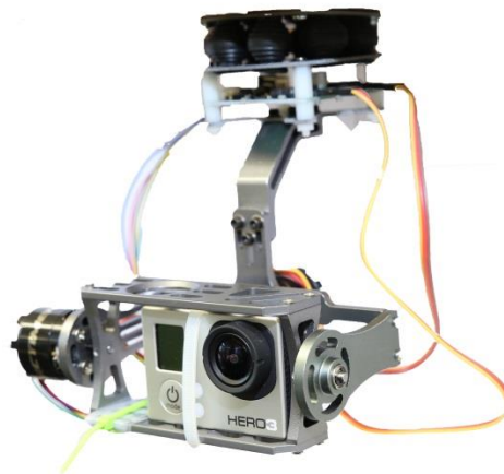
Figure 4-2: 2-Axis Gimbal with the recording unit.
