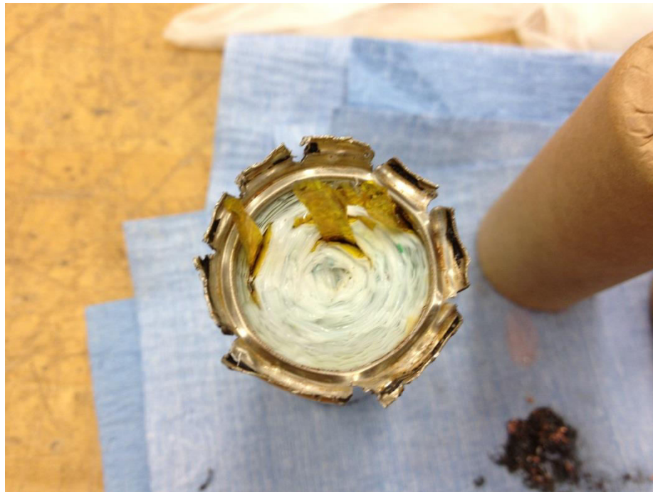
Figure 2-1 Top view cutout of a typical Li-ion cylindrical cell
