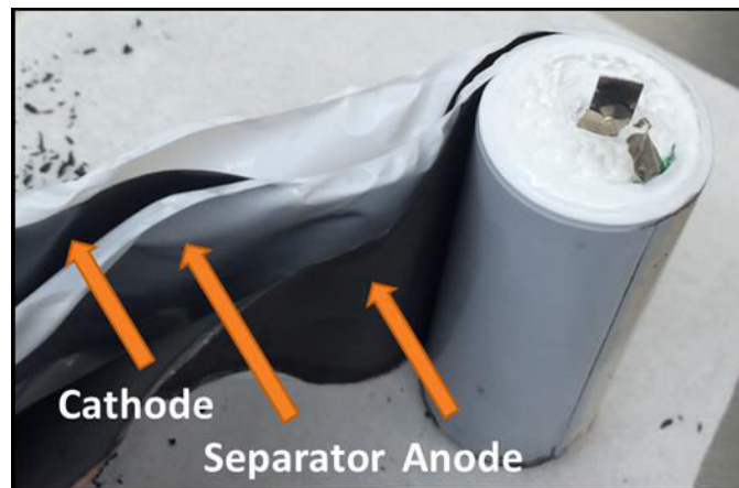
Figure 1-3 Disassembled 26650 to visualize internal material layers
