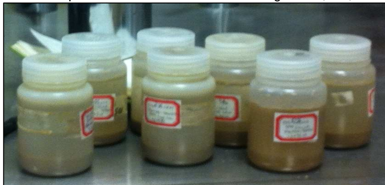
Figure 3.5 Lime-treated soil Sample for pH Test
