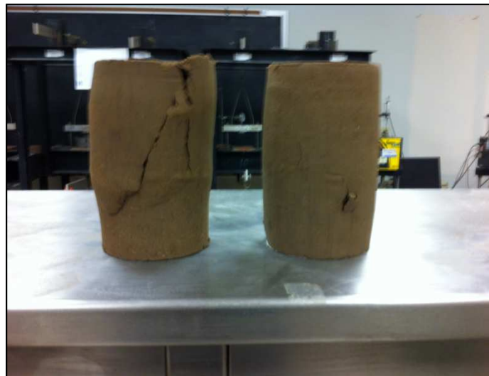
Figure 3.9 Failed Soil Specimens
