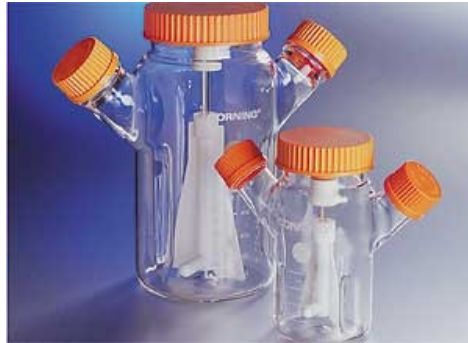
Fig. 3.1- ProCulture® Glass Spinner Reactor with Angled Side Arms
