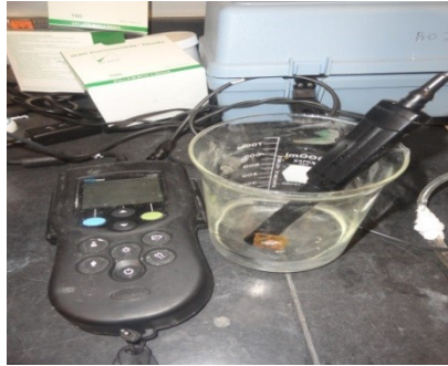
Fig. 3.14 – Probe to measure TDS and Conductivity
