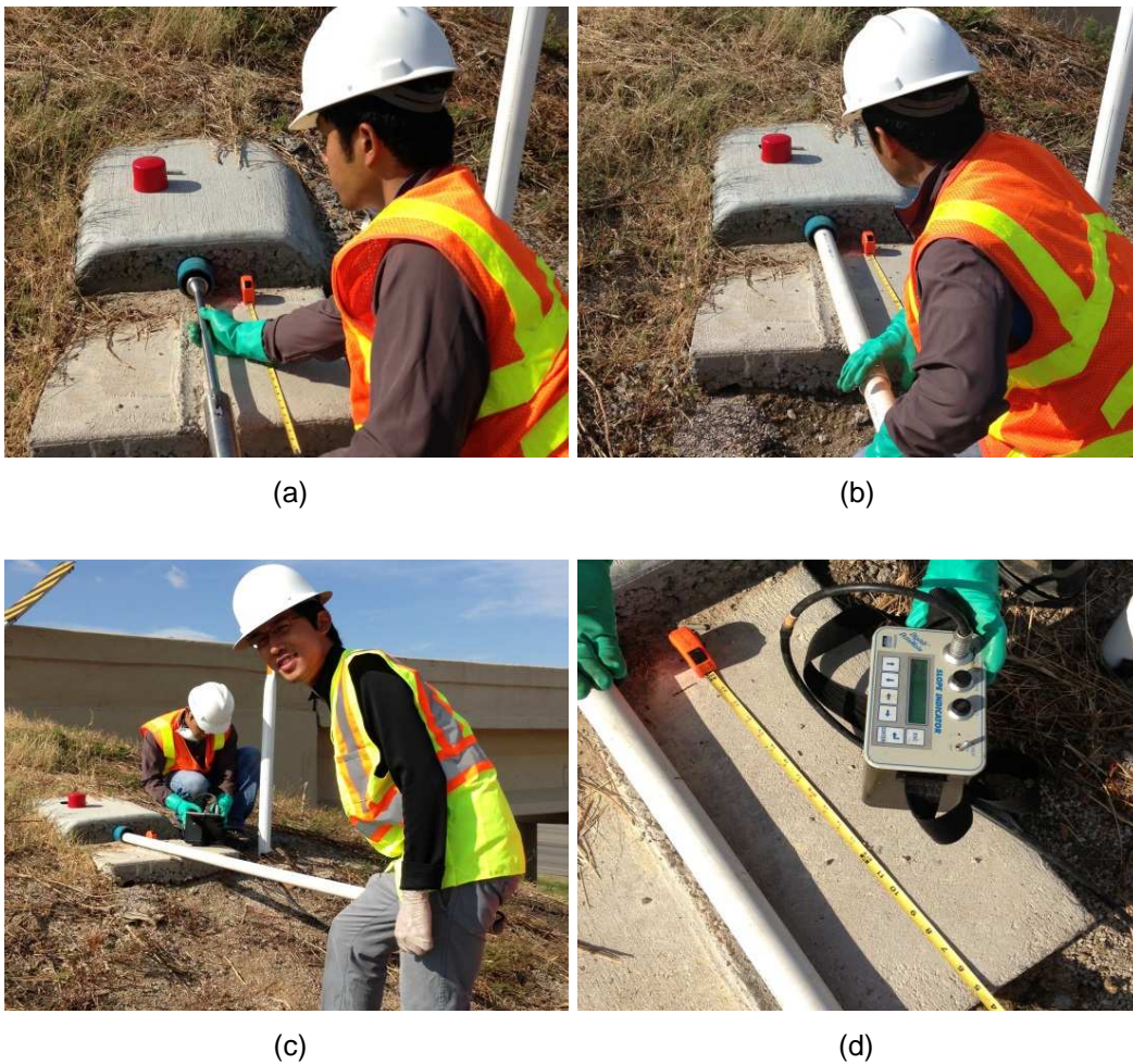
Figure 4.17 Process of an inclinometer survey: (a), (b), and (c) the process of passing horizontal probe into a casing; and (d) Digitilt DataMate used to record the readings
