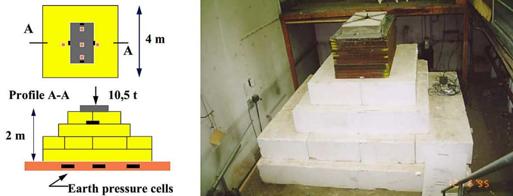
Figure 2.36 EPS test fill at the Norwegian Road Research Laboratory (Frydenlund and Aaboe, 2001)
