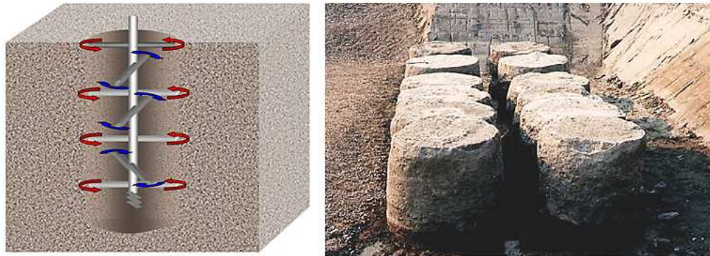
Figure 2.18 Deep soil mixing (DSM) operation and extruded DSM columns (Archeewa, 2010)
