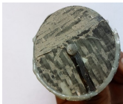
(e) Mixed failure mode in sample 5
