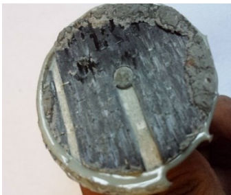
(g) Failure Modes F in sample 7
