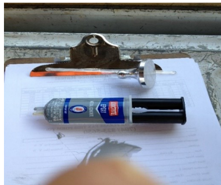
Figure 4-5 Epoxy used for bonding test dollies
