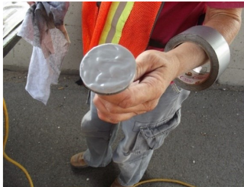
Figure 4-7 Epoxy applied to testing dollies
