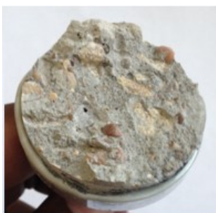
(b) Failure Mode G in sample 2
