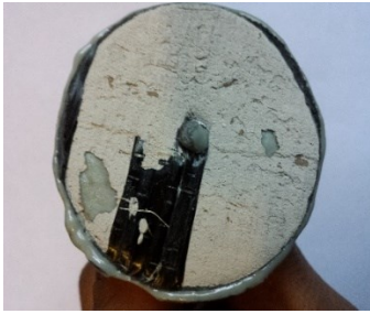
(a) Mixed failure Mode B in sample 1
