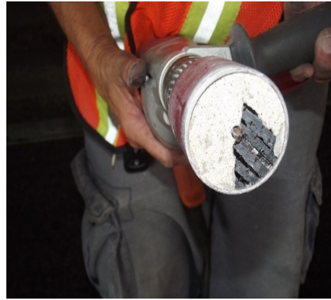
Figure 5-3 Core failure in sample 4 after drilling
