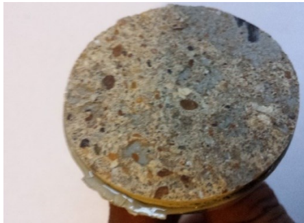
(a) Failure Mode G in sample 1
