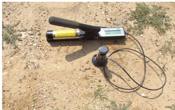
Figure 4-9 Positest pull-off adhesion tester
