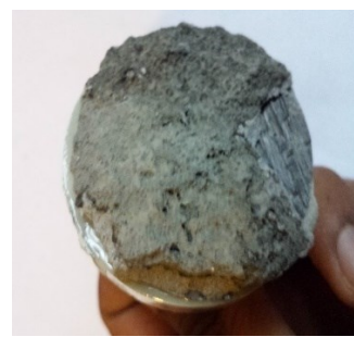
(f) Failure Mode F in sample 6
