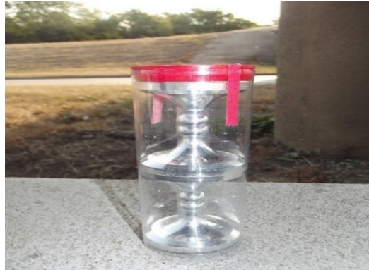
Figure 4-6 Dollies used for pull off test
