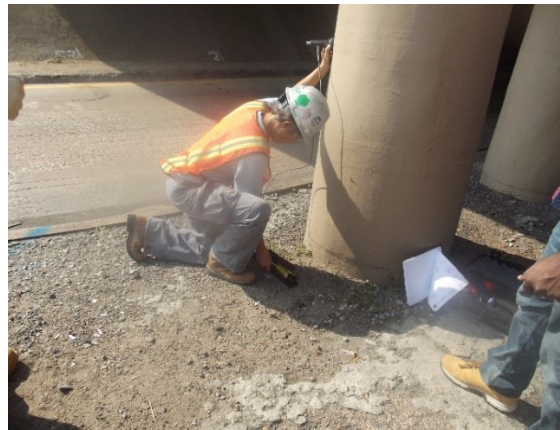
Figure 5-13 Pull-Off test on column 1 (sample 2), Bridge 3
