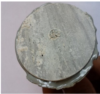
(a) Failure Mode F in sample 1
