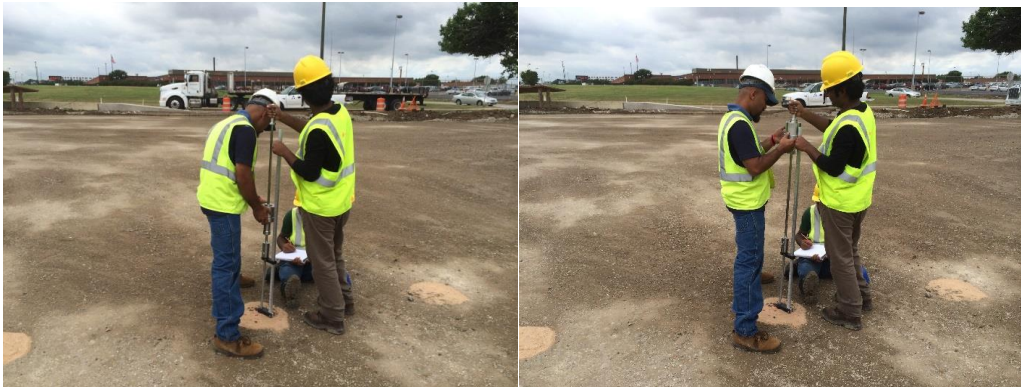
Figure 3.11: Dynamic Cone Penetrometer Test Photos
