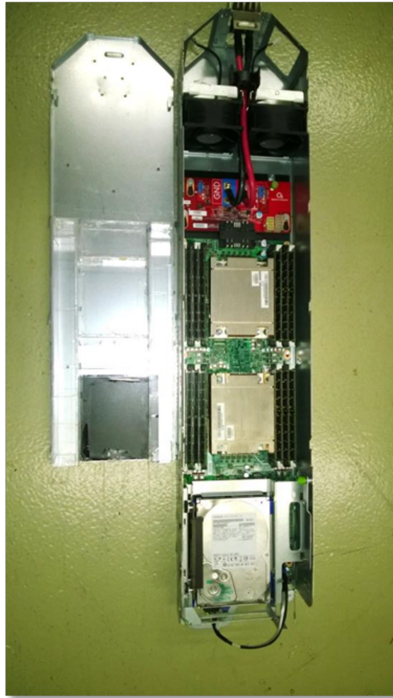
Figure 5.9. Server with improved chassis duct.
