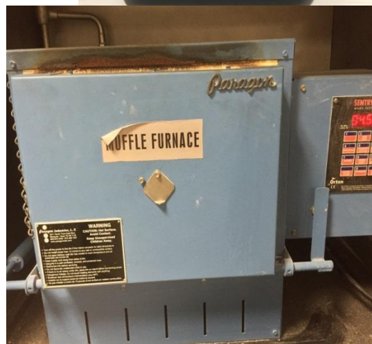
Figure 2-3 the activated carbon used for all the research tasks and the muffle furnace which is used to prepare the GAC-Fe.
