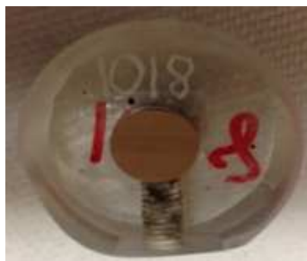
Figure 4-1 Sample as after preparation (with mirror finish)
