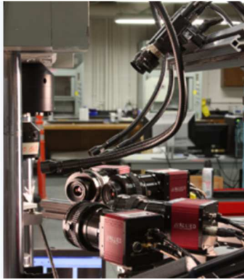
Figure 3-1 Typical DIC camera setup
