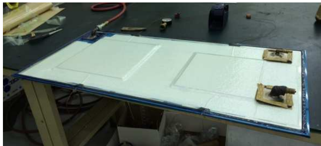
Figure 2-3 Leak check performed on bagged laminate
