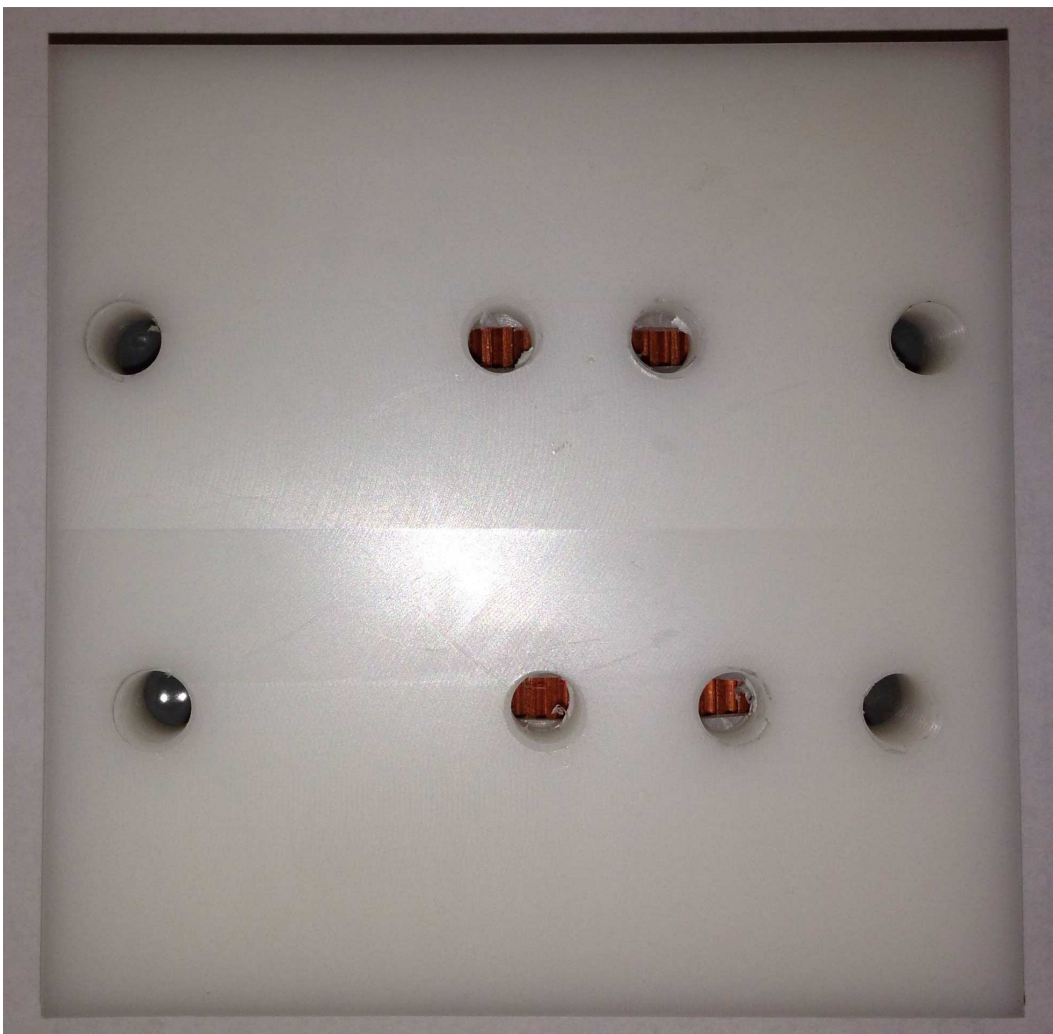
Figure A-1 Fabricated sample of finalized cold plate design
