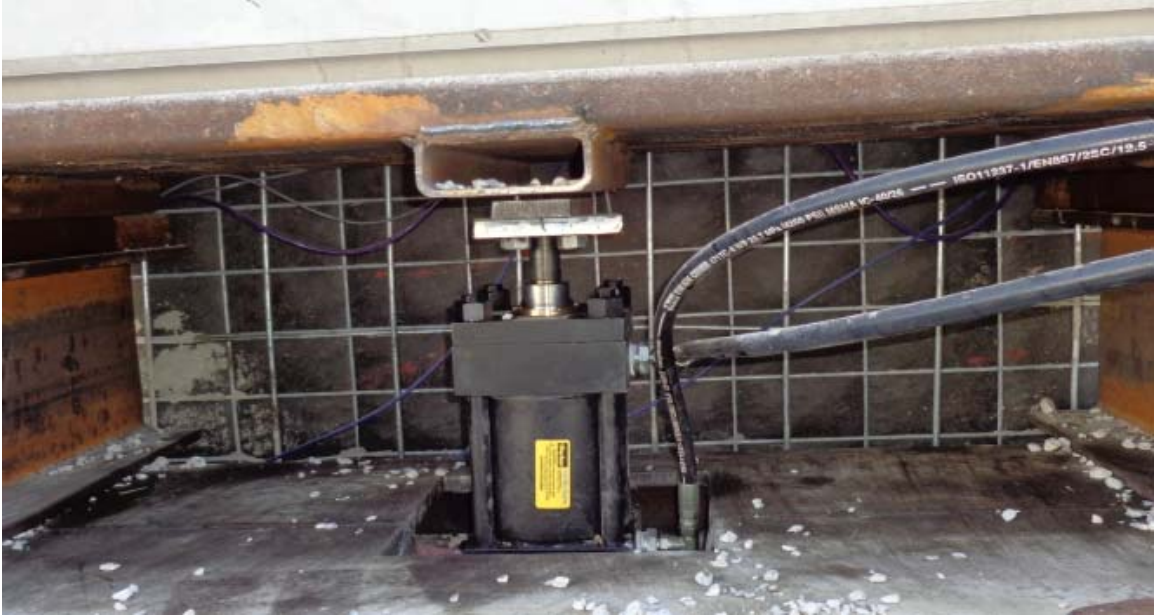
Figure 3-26 Hydraulic actuator to raise and lower platform
