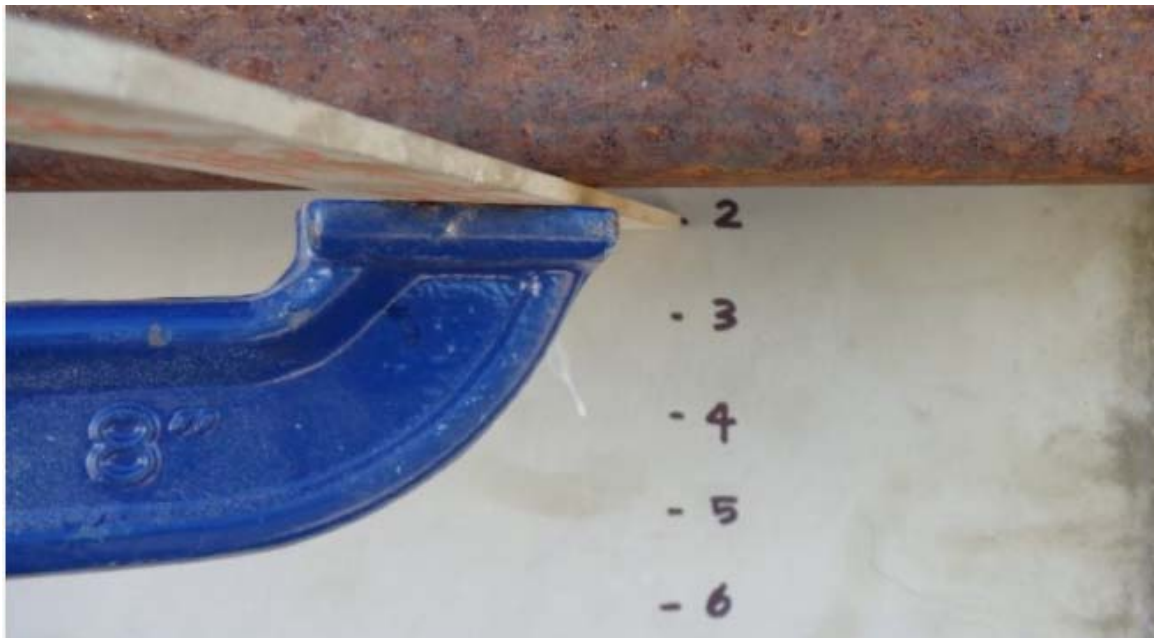
Figure 3-27 Platform raised 50 millimetres
