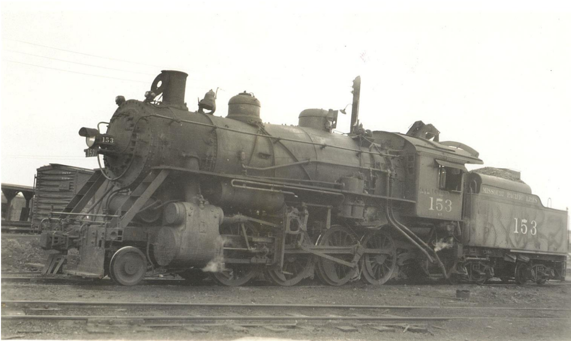
Figure 8 - 2-8-0 Consolidation-type Locomotive - Basis for Cooper's E loading [8]
