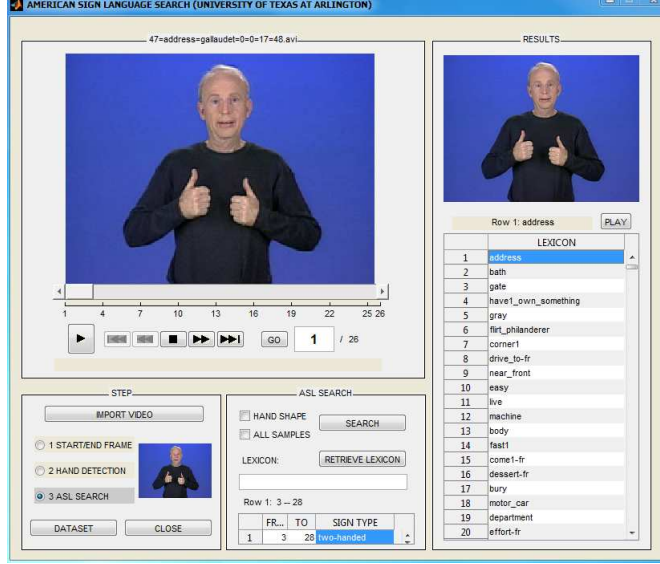
Figure 2.5: The step of matching the query with models in the proposed sign recognition system.
