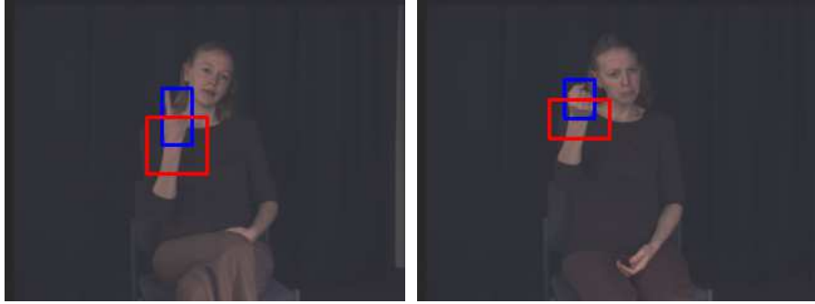
Figure 3.9: Context captured around the hand bounding box. The blue rectangle shows the hand bounding box and the red rectangle shows the extended box used to capture context around the hand. The context is captured over a region having the same height and twice the width as the hand.
