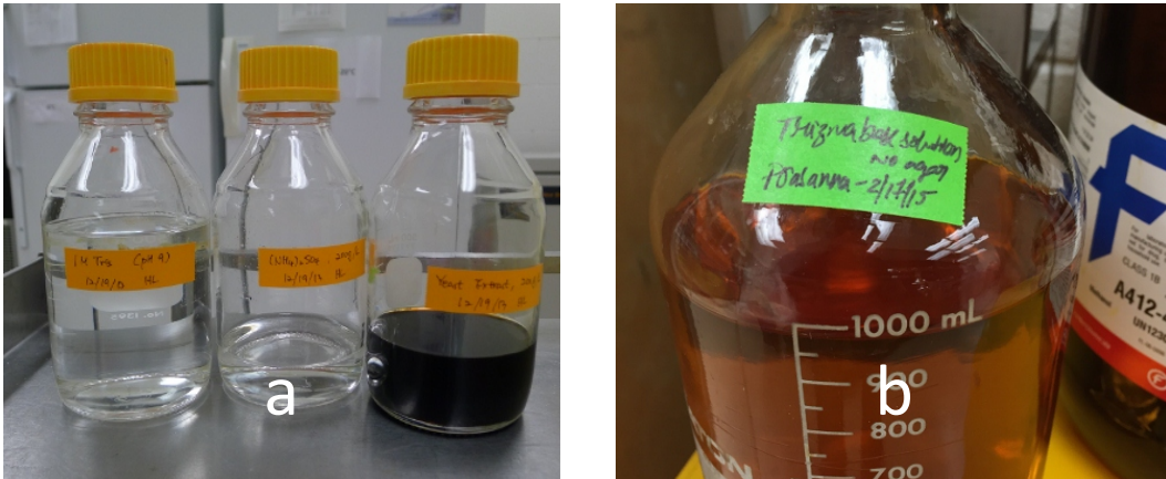
Fig 3-2: Preparation of Tris buffer solution a) Components autoclaved separately b) Solution of mixed components
