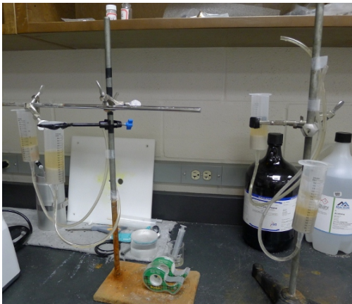
Fig 3-20: Experimental setup Images of calcium concentration influence on bio-cementation
