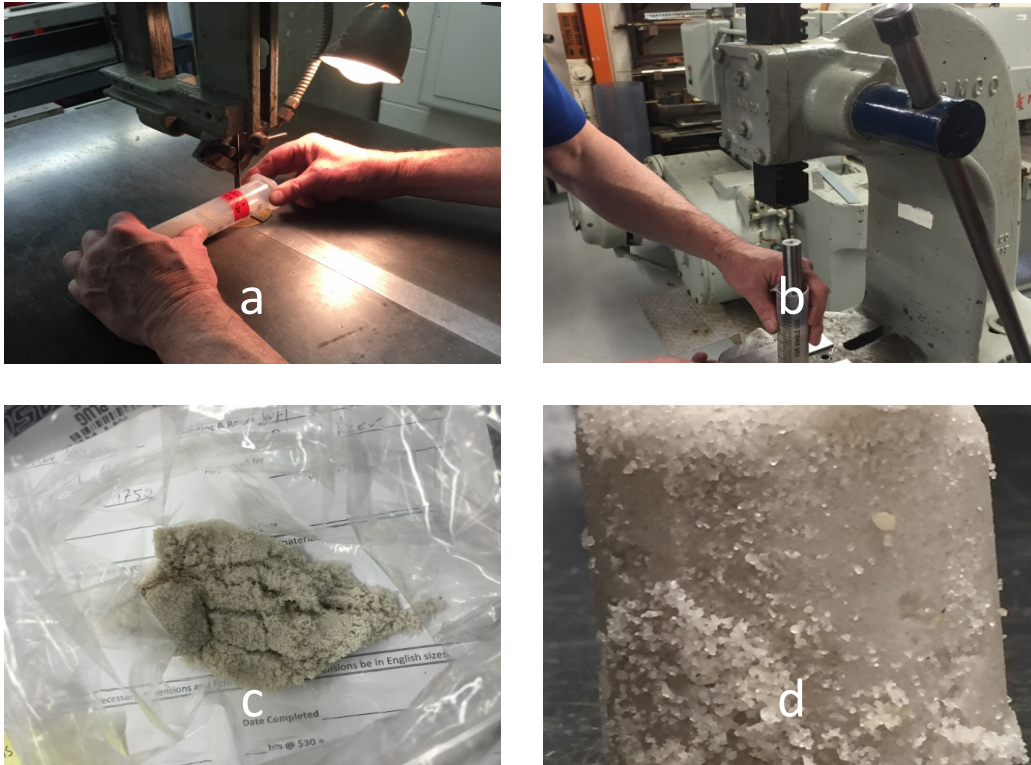
Fig 3-23: Images of sample after curing 16 days: a) Sawing bottom part of syringe, b) Extracting the sample, c) Single bacterial injection, d) Multiple bacterial injections
