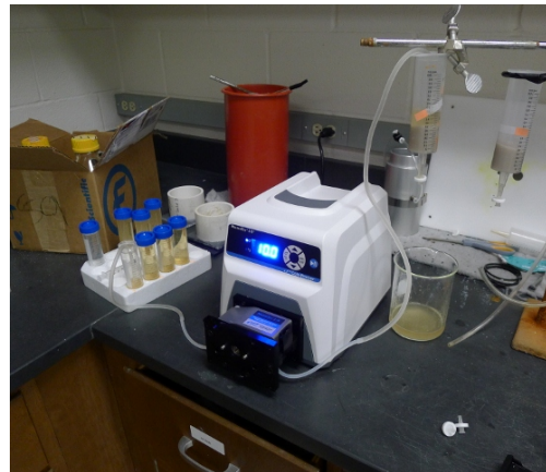
Fig 3-20: Experimental setup Images of calcium concentration influence on bio-cementation
