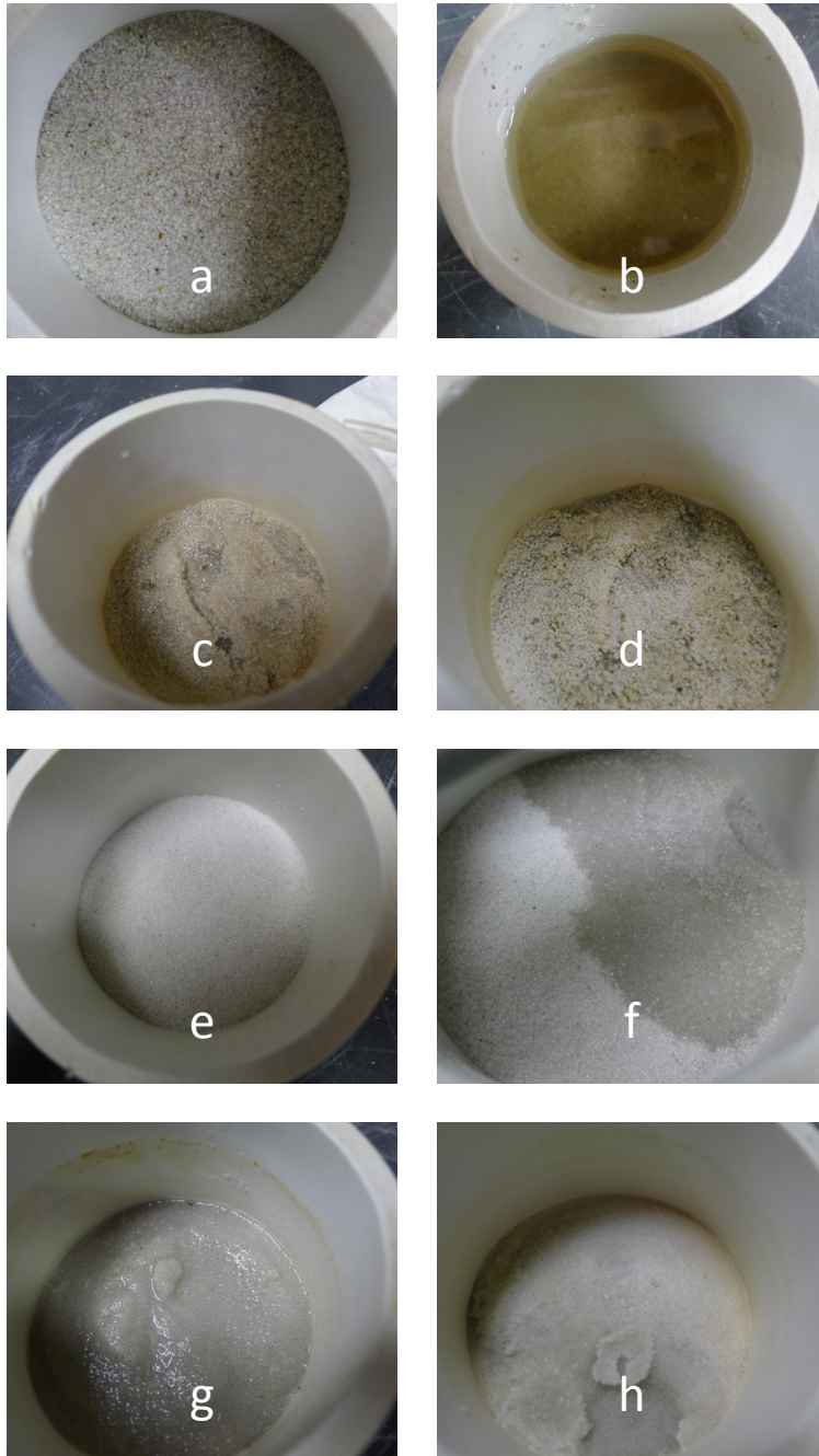
Fig 3-14 Description of particle size experiment: Ottawa sand a) sample of Ottawa sand, b) Sample saturated with bacterial solution, c) During cementation, d) End of test, e) Sample of well-graded sand, f) Application of nutrient solution, g) In between nutrient cycles, h) End of test
