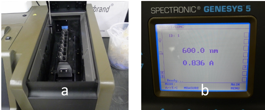
Fig 3-9: Bacteria counting technique: a) Spectra Genesis 5 spectrometer, b) Absorbance at 600 nm wavelength
