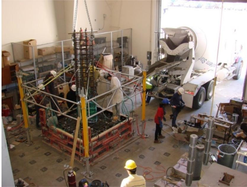
Figure 162. Bottom Block Casting.
