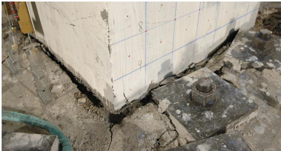
Figure 100. Damage and separation at the column-footing interface
