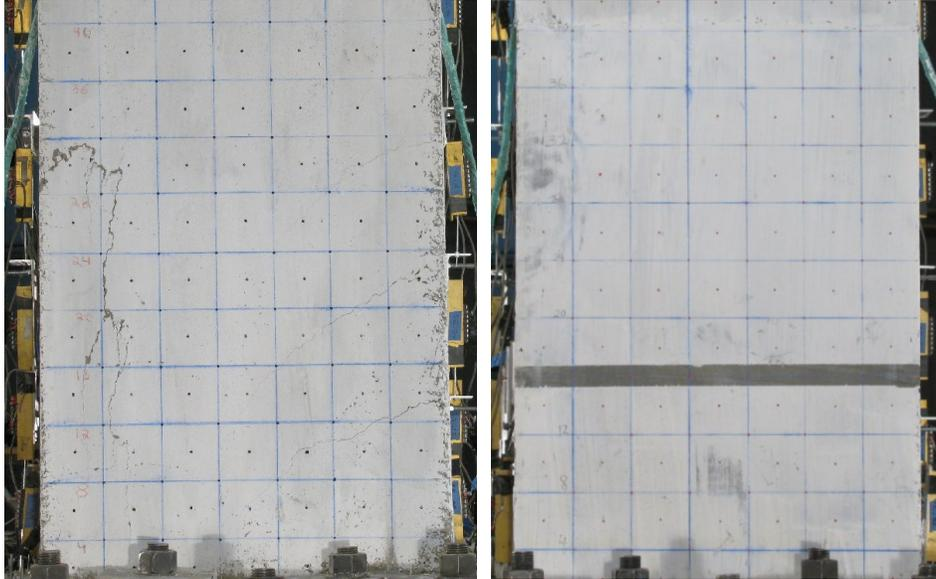
Figure 96. Column specimen SP5 and SP8 at 0.75% drift
