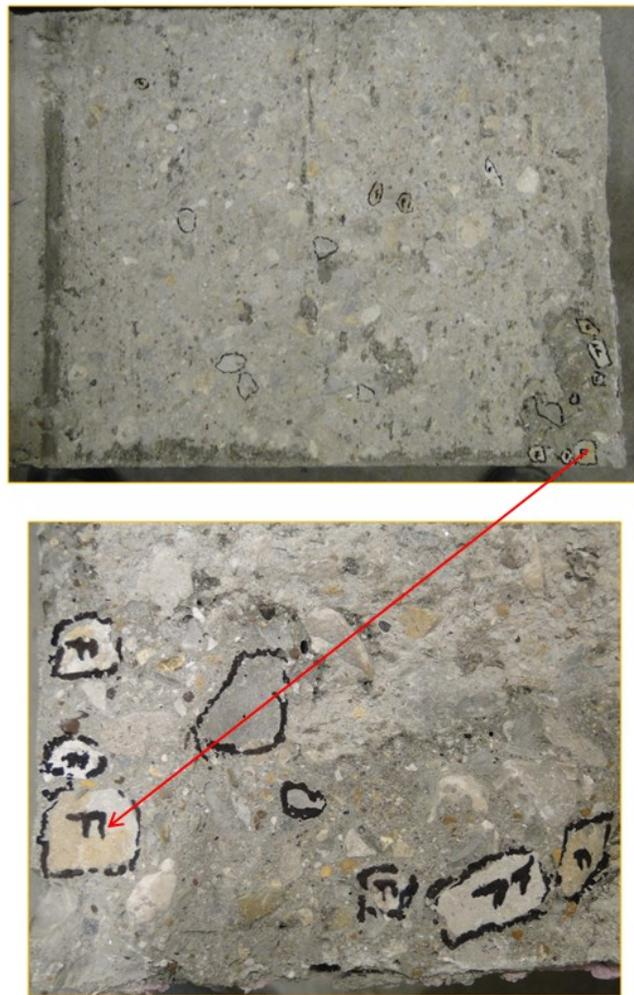
Figure 311. CSP 8 specimen precast failure plane showing dislodged and fractured aggregates
