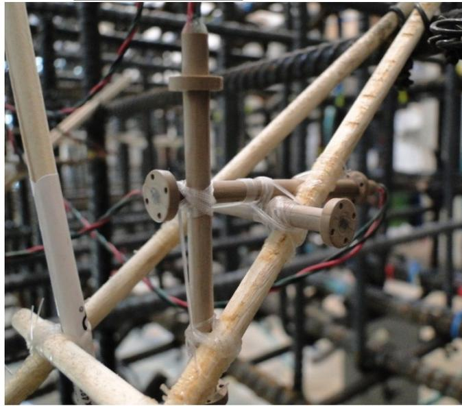
Figure 141. Location of concrete strain gauges for space frame and perimeter frame columns
