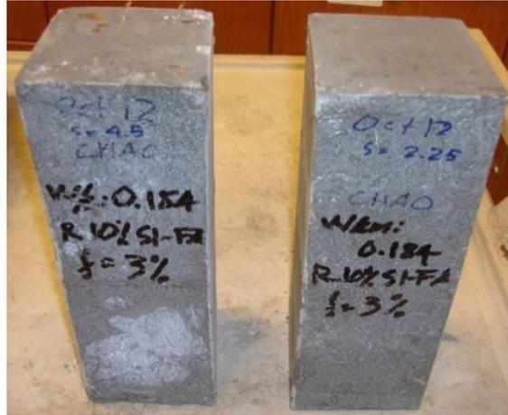
Figure 39. Specimens B2 and B4 after formwork removal and grinding
