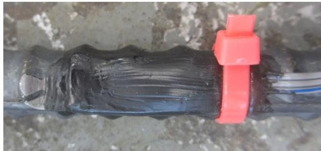
Figure 75. Completed strain gauge installation
