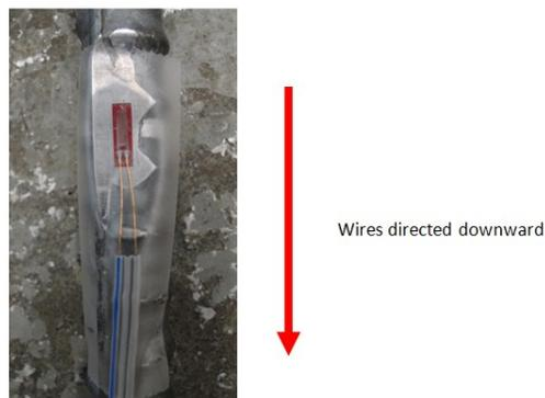
Figure 25. Lining up the gauge crosshairs to the proper location on the rebar
