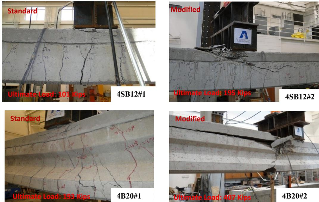
Figure 319. Full-scale beam specimens at failure
