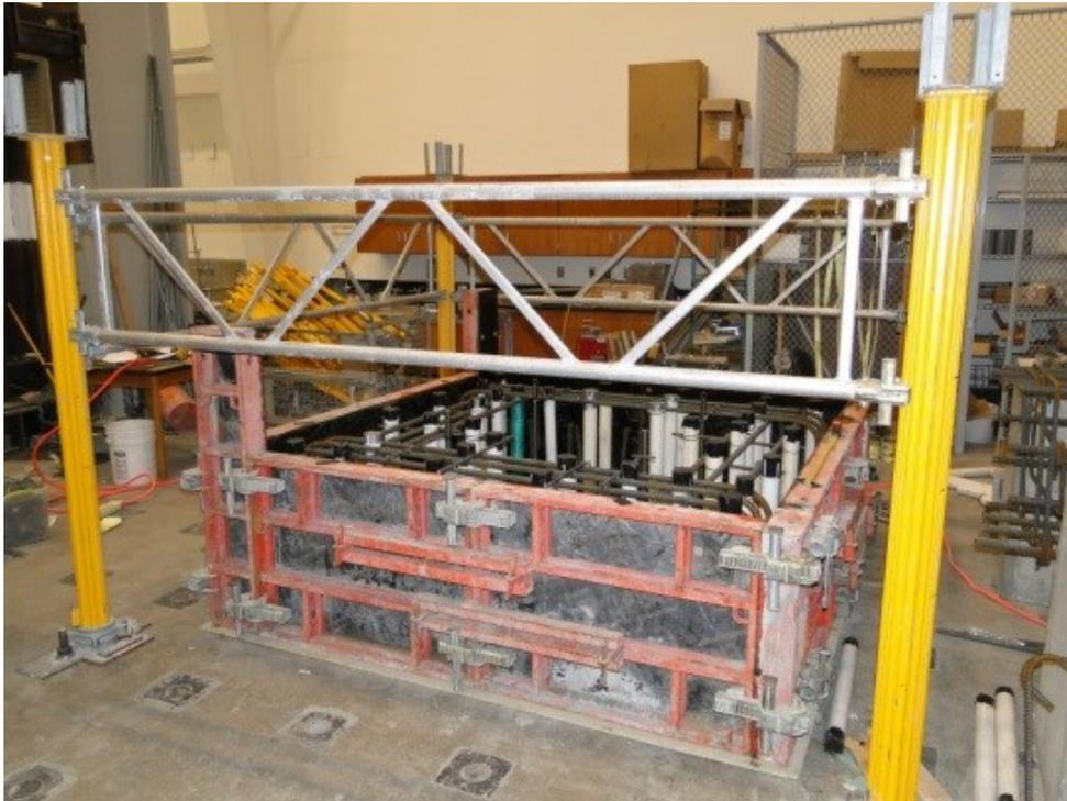
Figure 53. Footing block reinforcement and formwork
