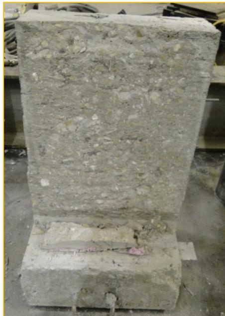
Figure 36: Failure into the CIP at the top notch.
