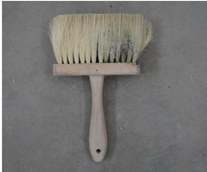
Figure 199. Concrete broom
