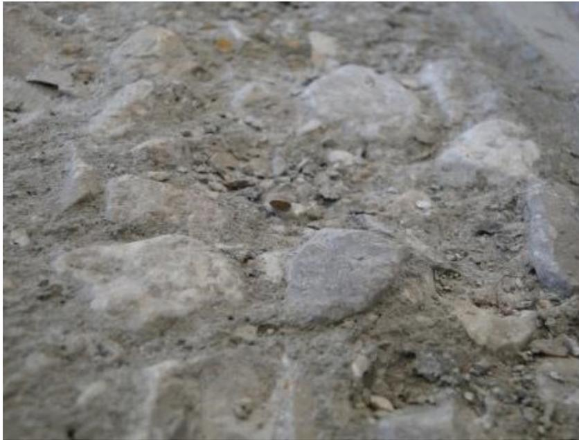
Figure 312. CSP 9 specimen surface profile
