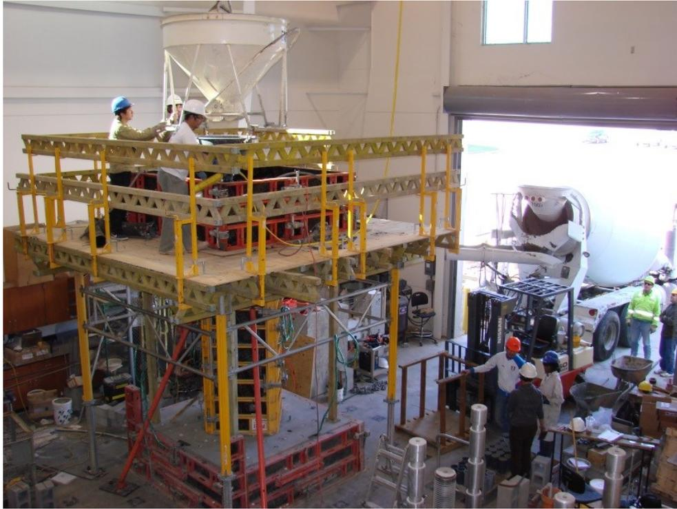
Figure 60. Final column and loading block casting
