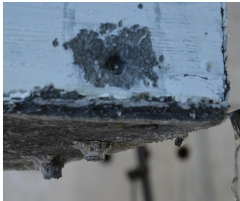
Figure 110. Longitudinal bar pull-out from footing after testing
