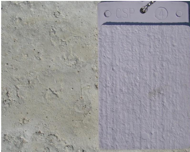
Figure 170. SCC concrete surface compared to CSP 4
