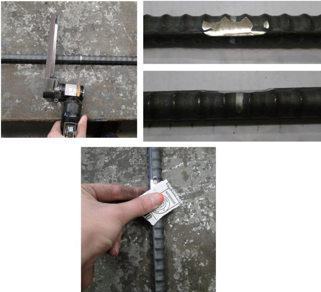
Figure 21. Grinding and sanding of deformed rebars
