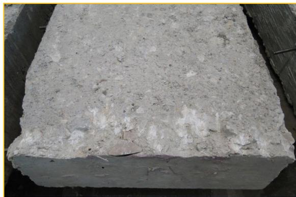
(c) Fracturing of concrete near notch.
