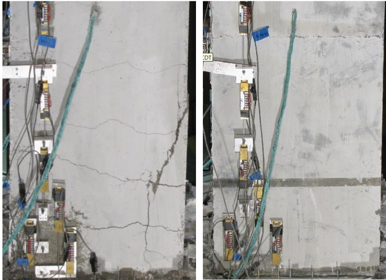
Figure 97. Column specimen SP5 and SP8 at 1.4% drift
