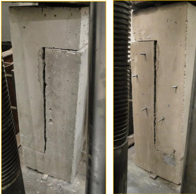
Figure 28. CSP 8 Specimen #1 failure (a) front view (b) back view.
