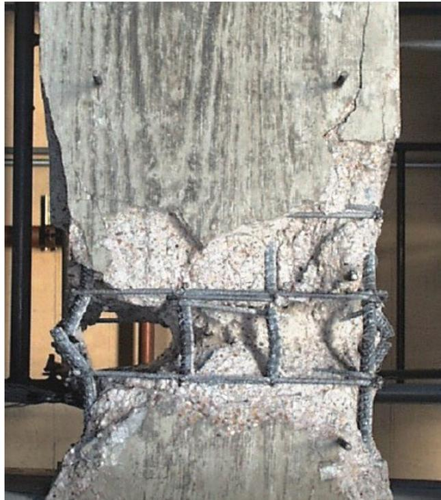
Figure 26. Specimen S24-4UT after failure (Bae, 2005)
