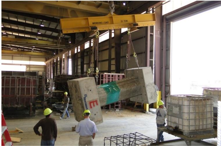
Figure 154. Lifting column horizontally
