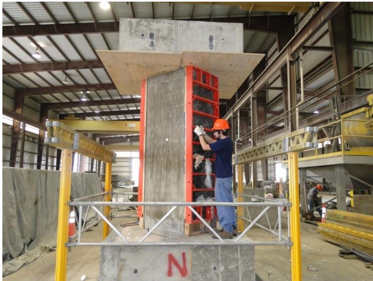
Figure 135. Removing LVDT rods
