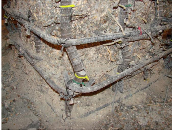
Figure 107. Column SP5 after testing
