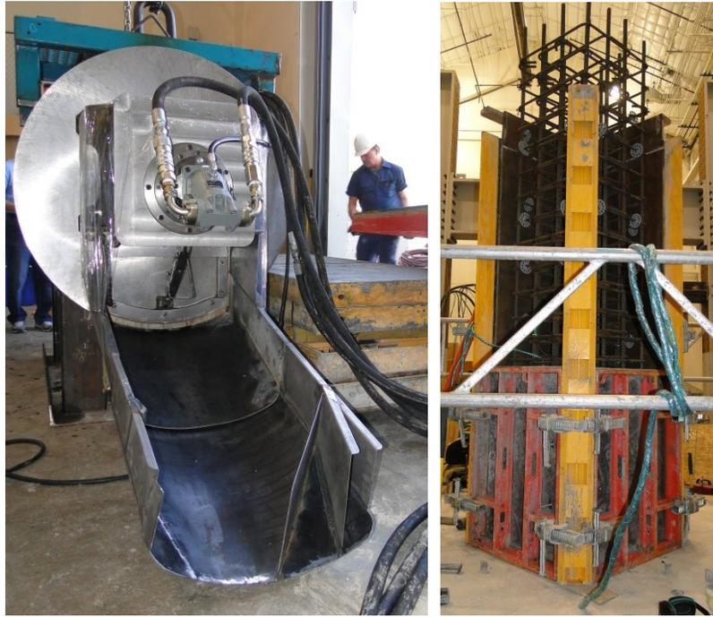
Figure 64. Mixer and formwork for 40 in. UHP-FRC section
