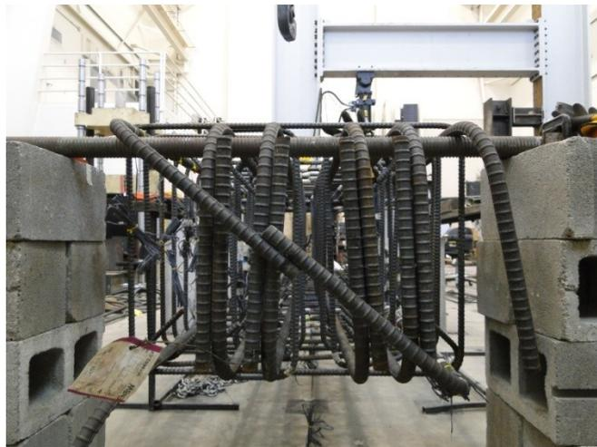
Figure 43. Tied longitudinal bars at the base of the column
