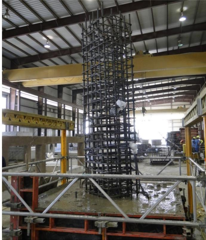
Figure 83. Cast bottom block
