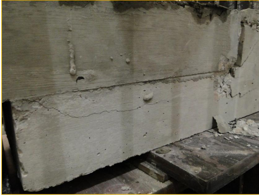
(a) Failure progressing into precast part.
