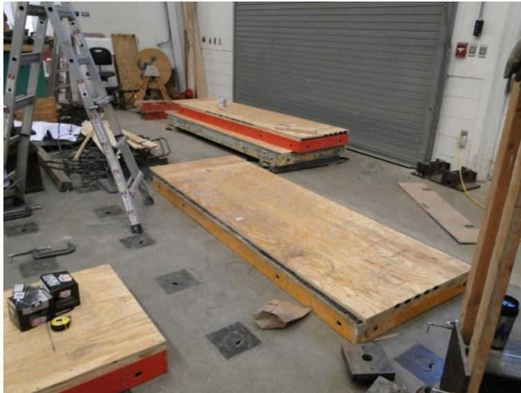
Figure 66. Completed column formwork modification
