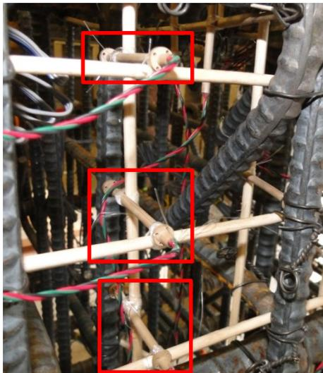
Figure 79. Concrete strain gauges
