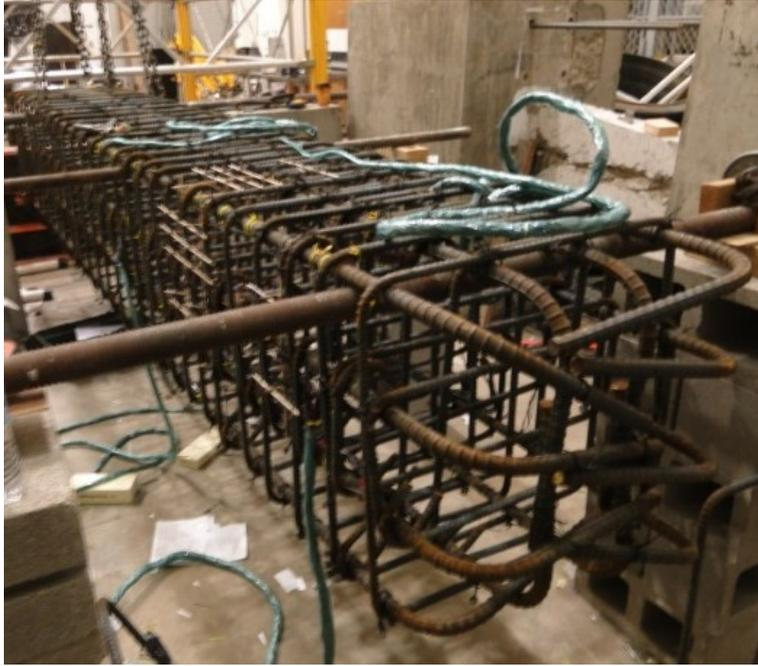
Figure 54. Completed column reinforcement cage
