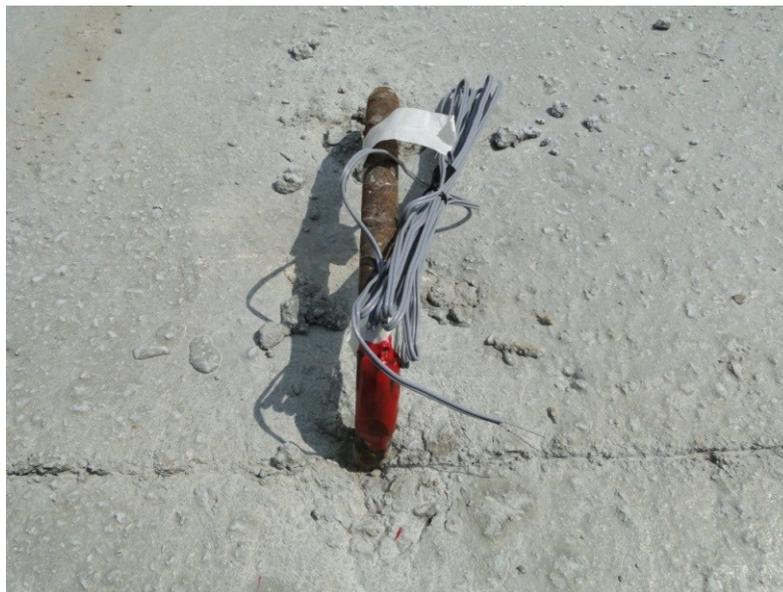
Figure 300. Strain gauges installation on horizontal shear reinforcements
