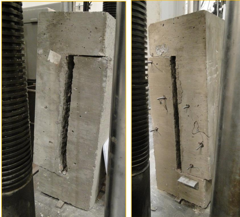
Figure 31. CSP 8 Specimen #2 failure (a) front view (b) back view.
