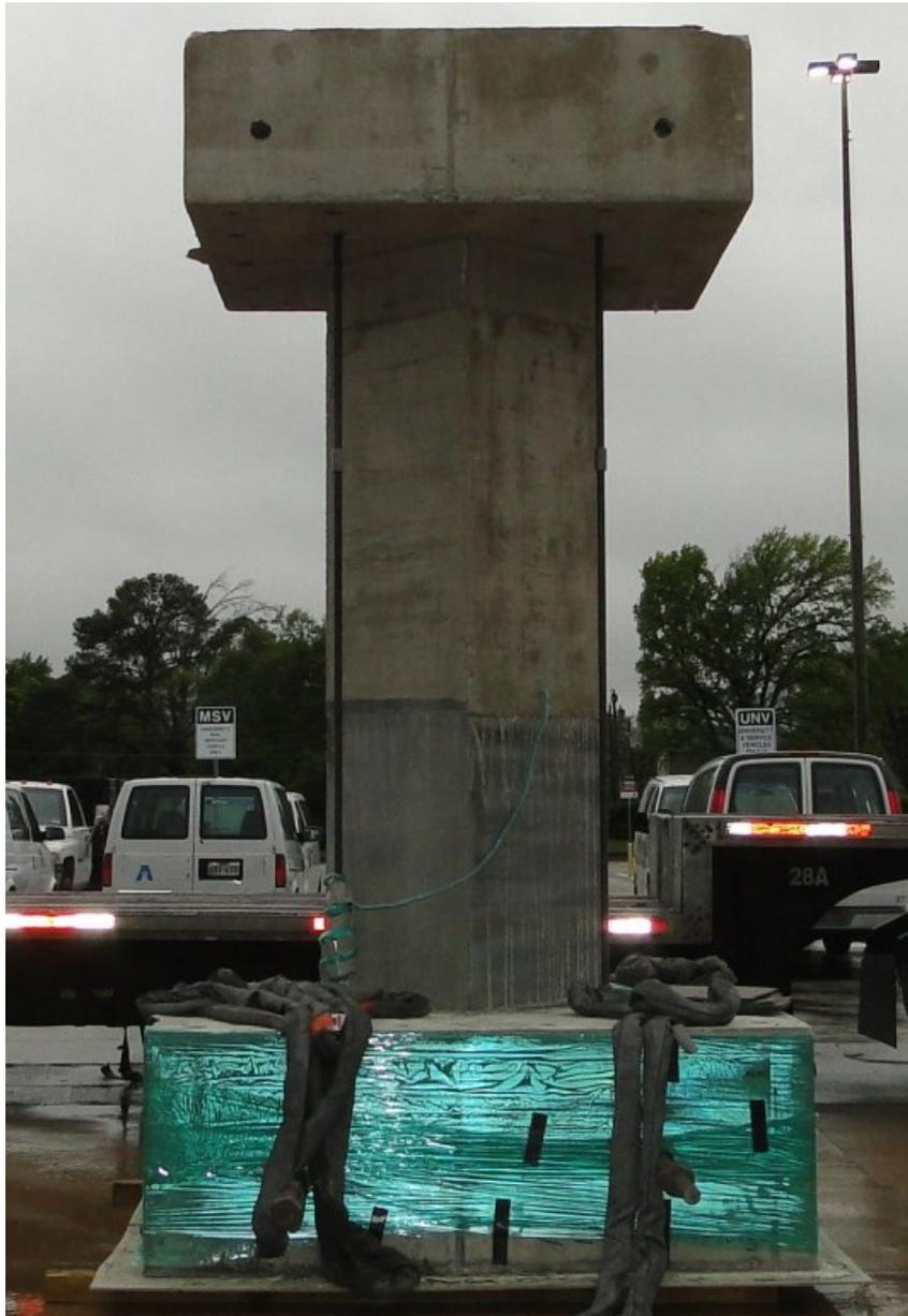
Figure 70. Space frame column specimen SP8
