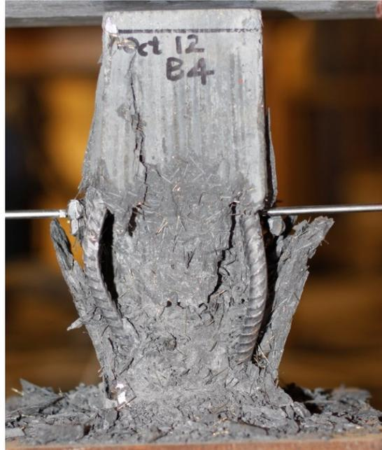
Figure 47. Crushing of specimen B4
