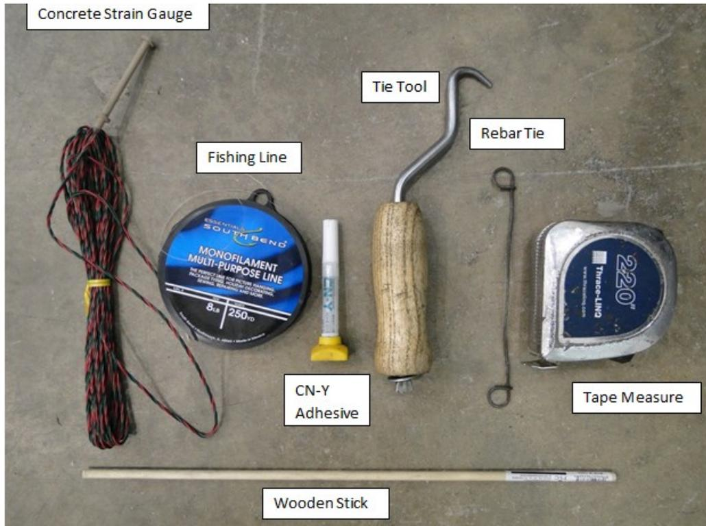
Figure 49. Concrete Strain Gauge Instillation Materials.
