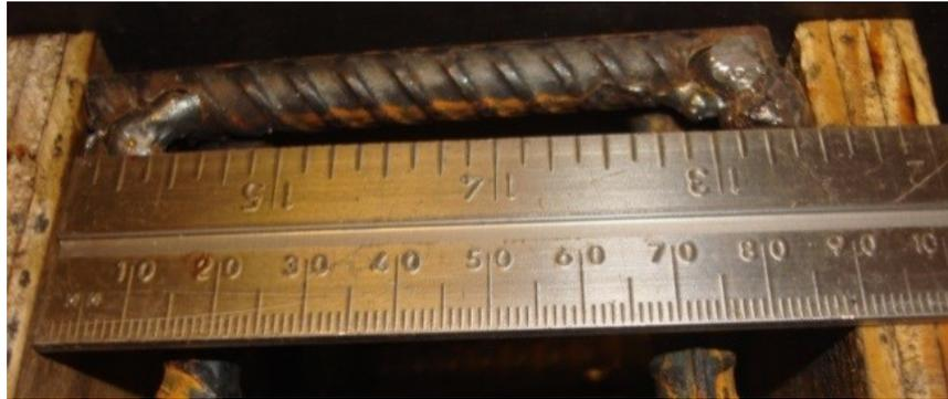
Figure 37. Tolerance checking to make sure the different is less than 1/8 in.
