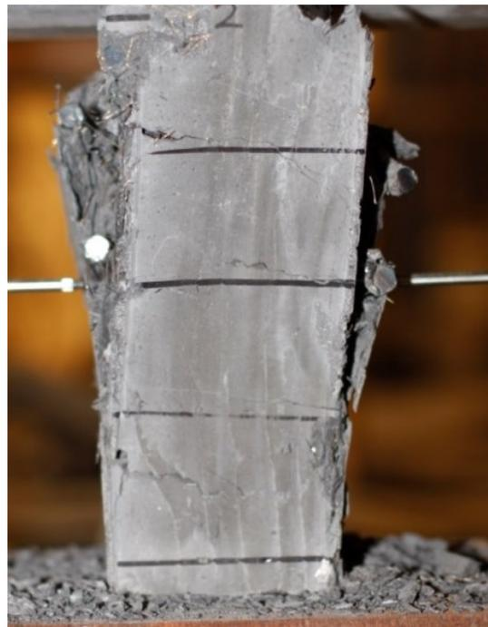
Figure 48. Crushing of specimen B2
