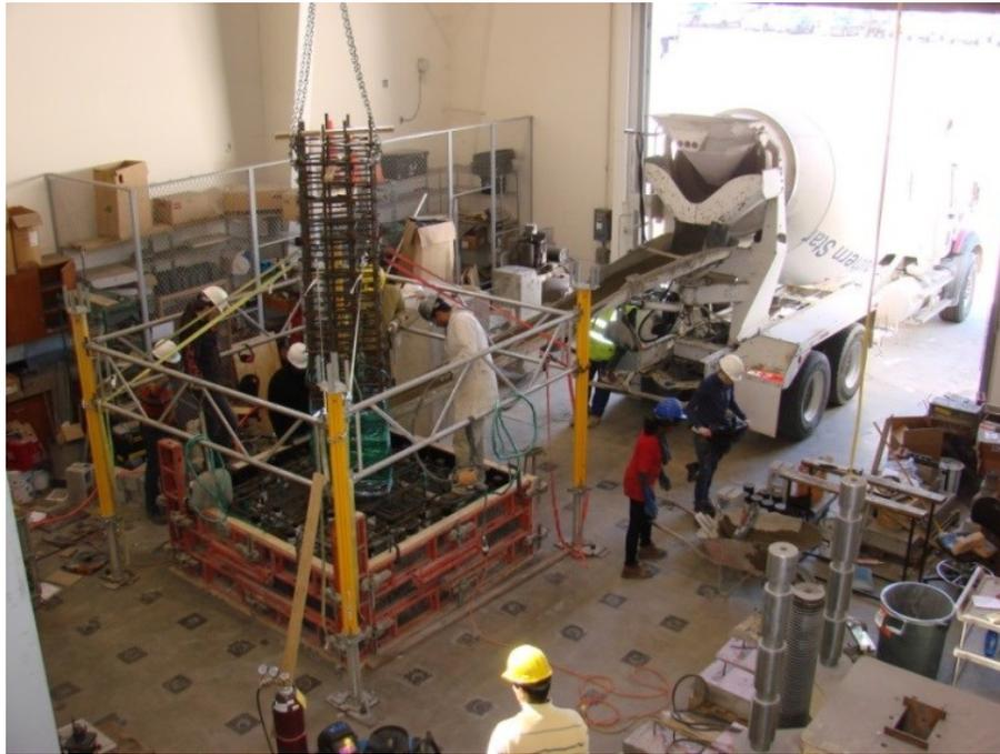
Figure 57. Footing block casting
