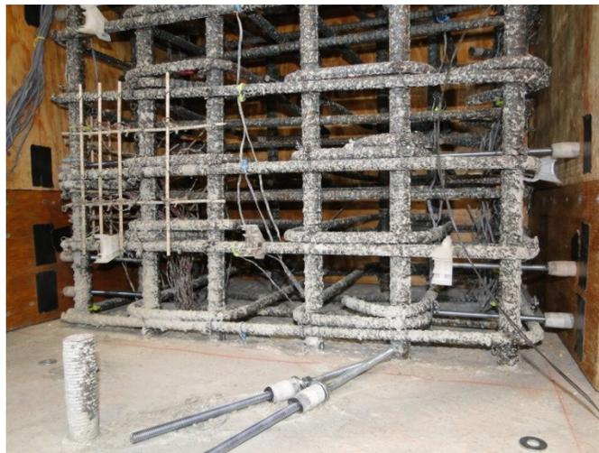
Figure 95. Placing of LVDT rods on both formwork panels
