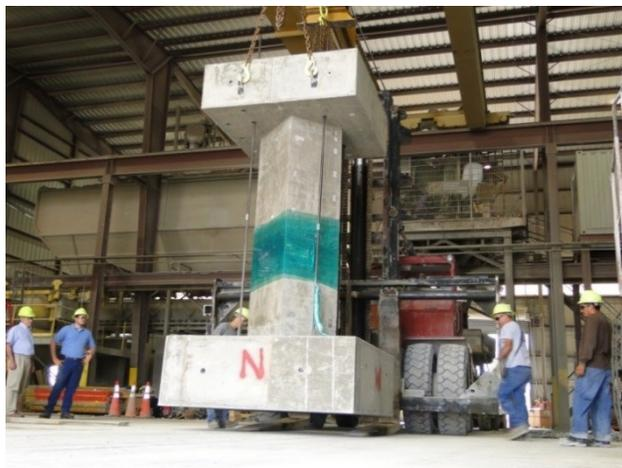
Figure 147. Setting column on forklift
