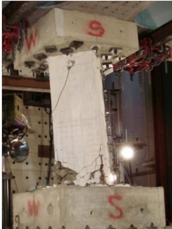
Figure 143. SP3 column subjected to a symmetric cyclic loading protocol
