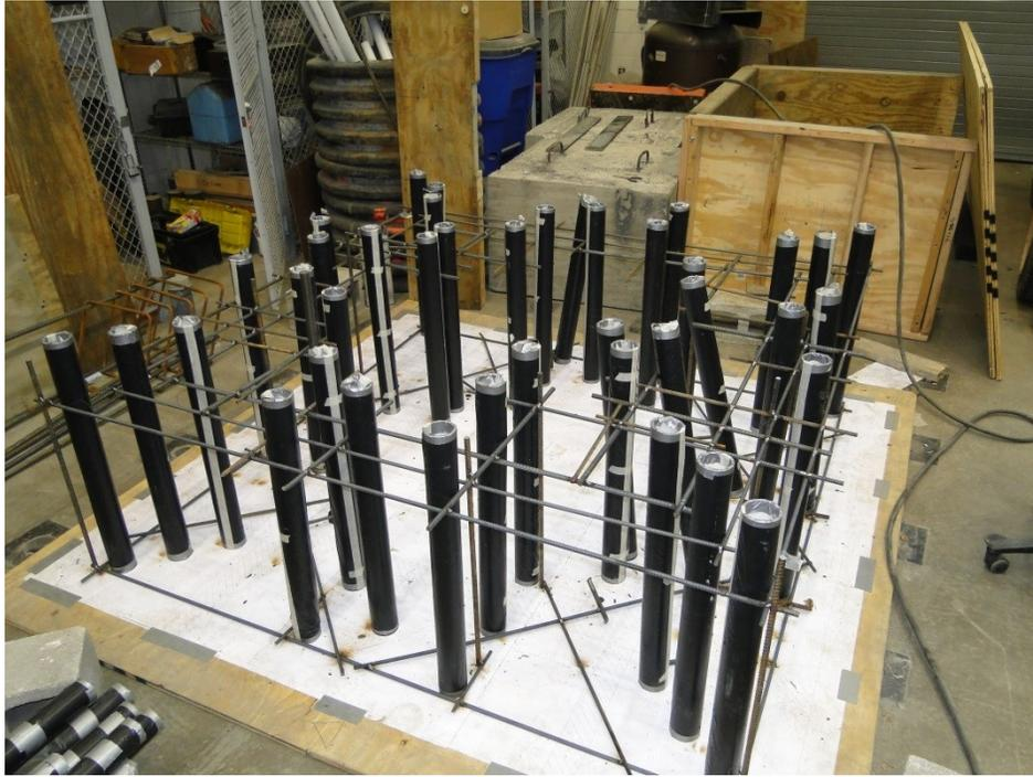
Figure 23. Final bottom block reinforcing bar grid.
