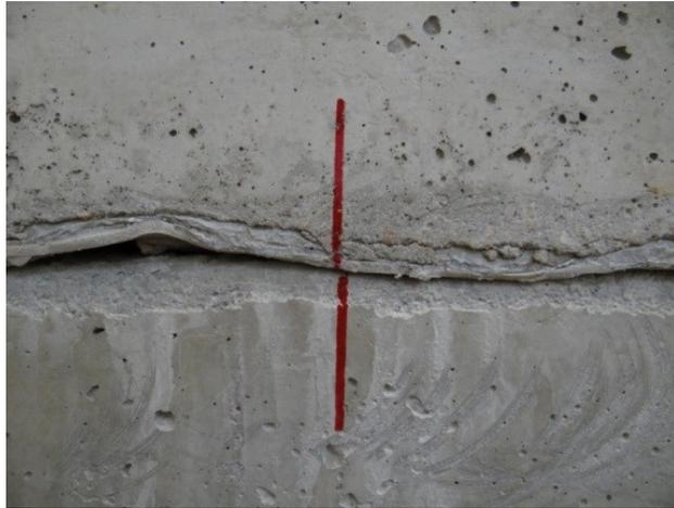
Figure 326. Interface slip at 180 kips
