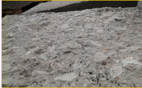
(b) Extremely rough surface showing both fracture and pullout
