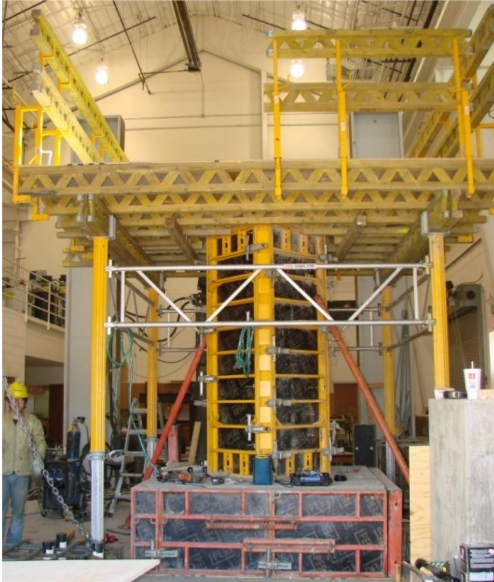
Figure 59. Column formwork and loading block platform
