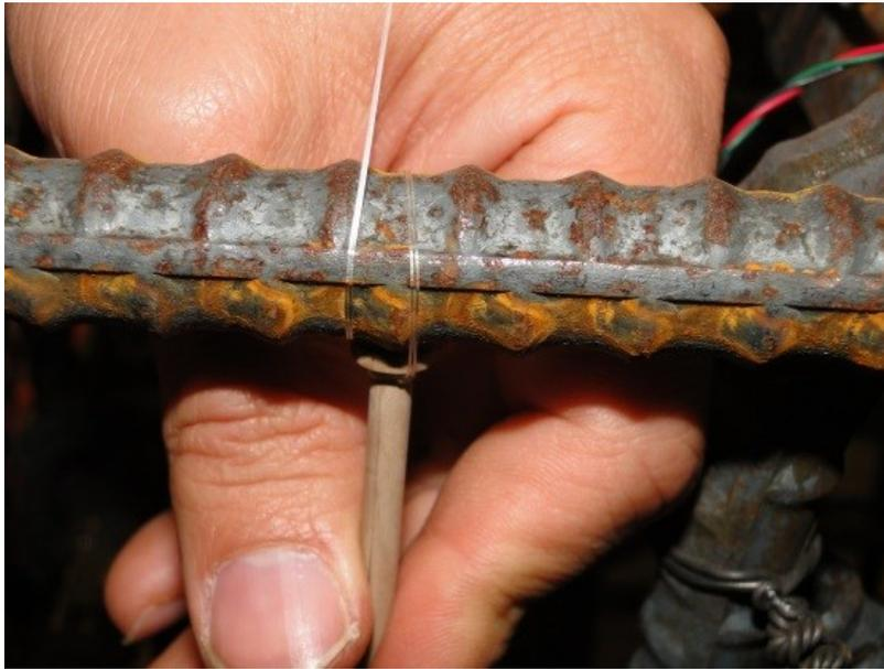
Figure 63. Tying concrete gauge to rebar
