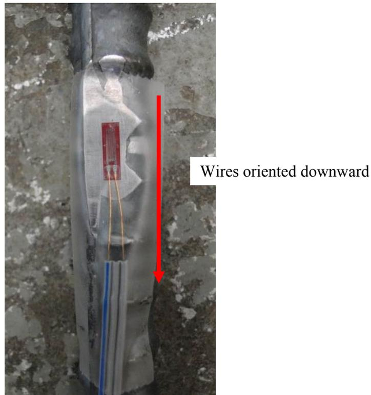
Figure 18. Strain gauge orientation
