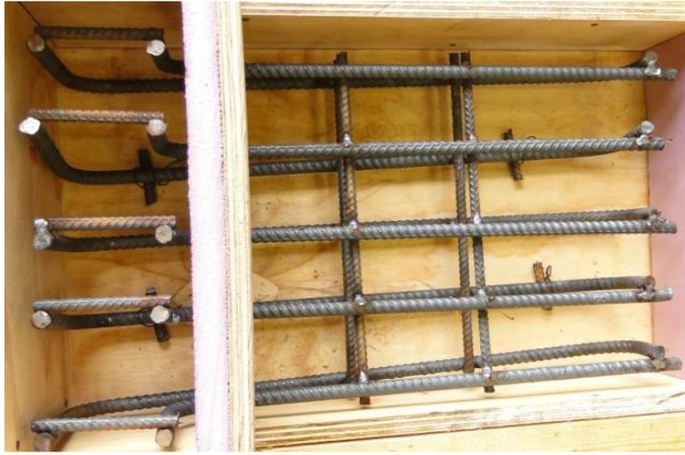
Figure 190. Caging for precast part of specimen
