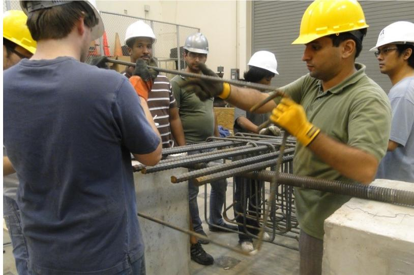
Figure 39. Placement of upper hoop configuration
