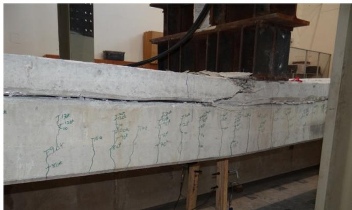
Figure 321. Beam at failure
