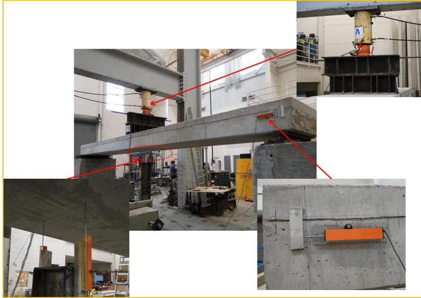
Figure 306. Test setup: LVDT's and loading beams
