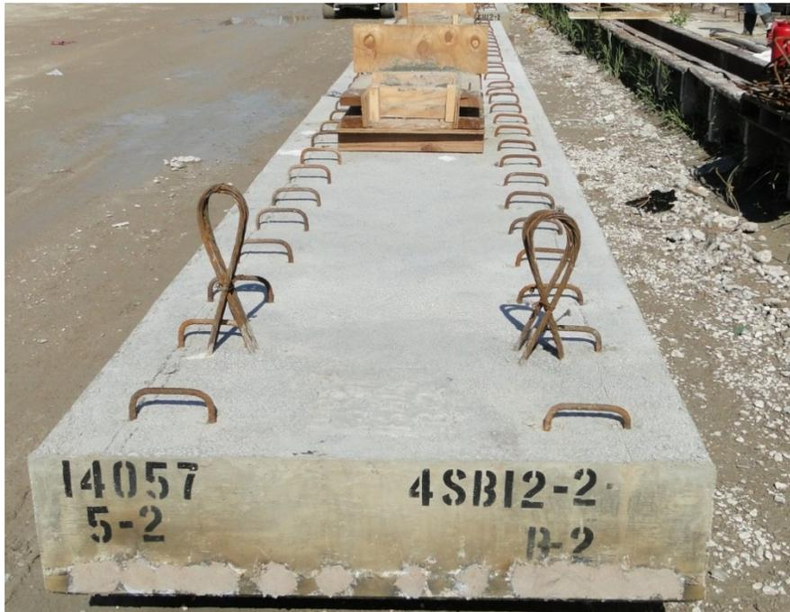
Figure 295. Finished slab beam specimen
