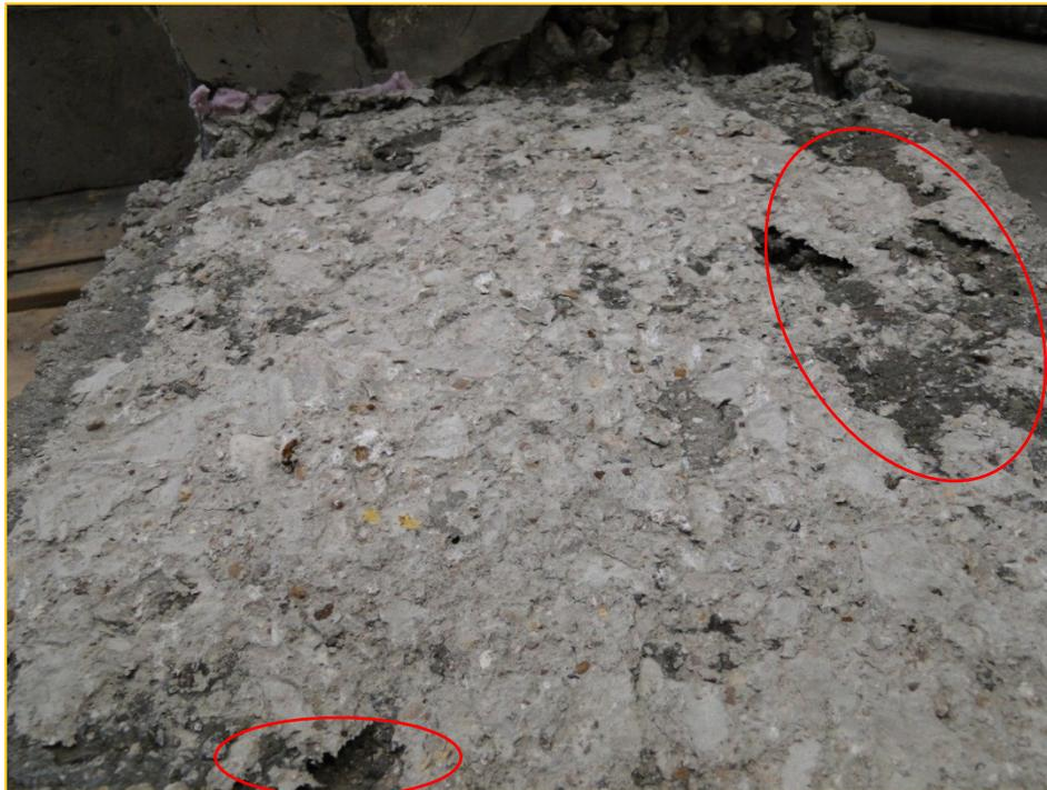
Figure 5. Wood Float Specimen #1 Cast in-place failure plane.
