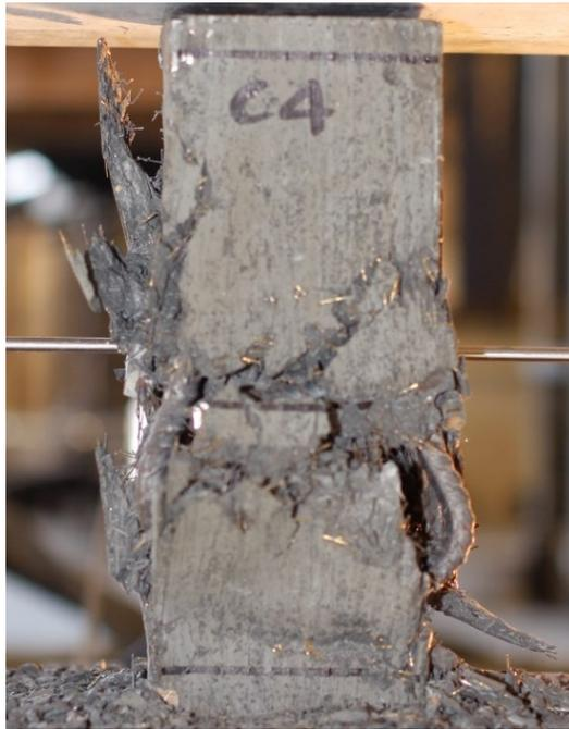
Figure 49. Crushing of specimen C4
