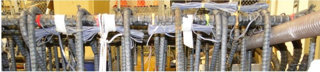
Figure 7. Orientation of strain gauges on longitudinal Bar 3 (on bottom ridge)
