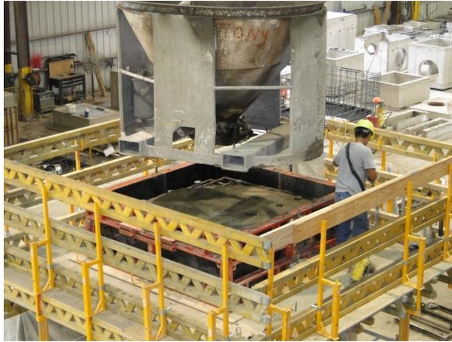
Figure 130. Top block casting.
