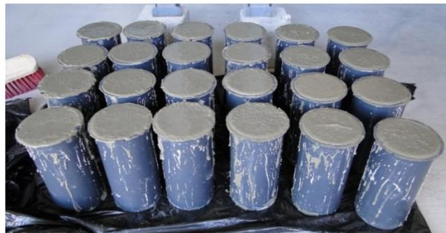
Figure 84. 24 Concrete Cylinders
