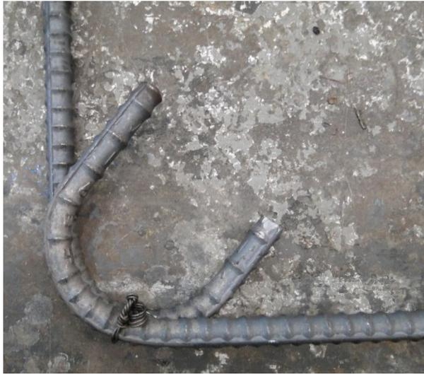
Figure 15. Hoop with hooks tied in place before measuring strain gauge locations
