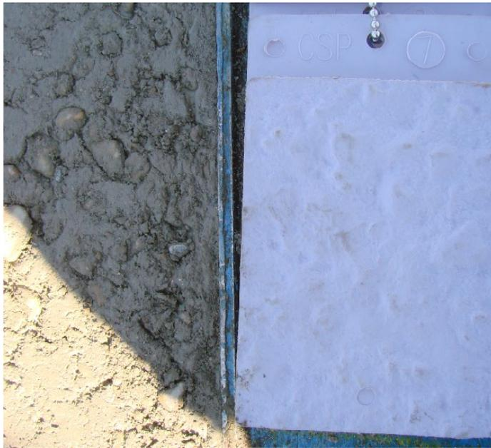
Figure 171. Wood float concrete surface compared to CSP 6 and CSP 7
