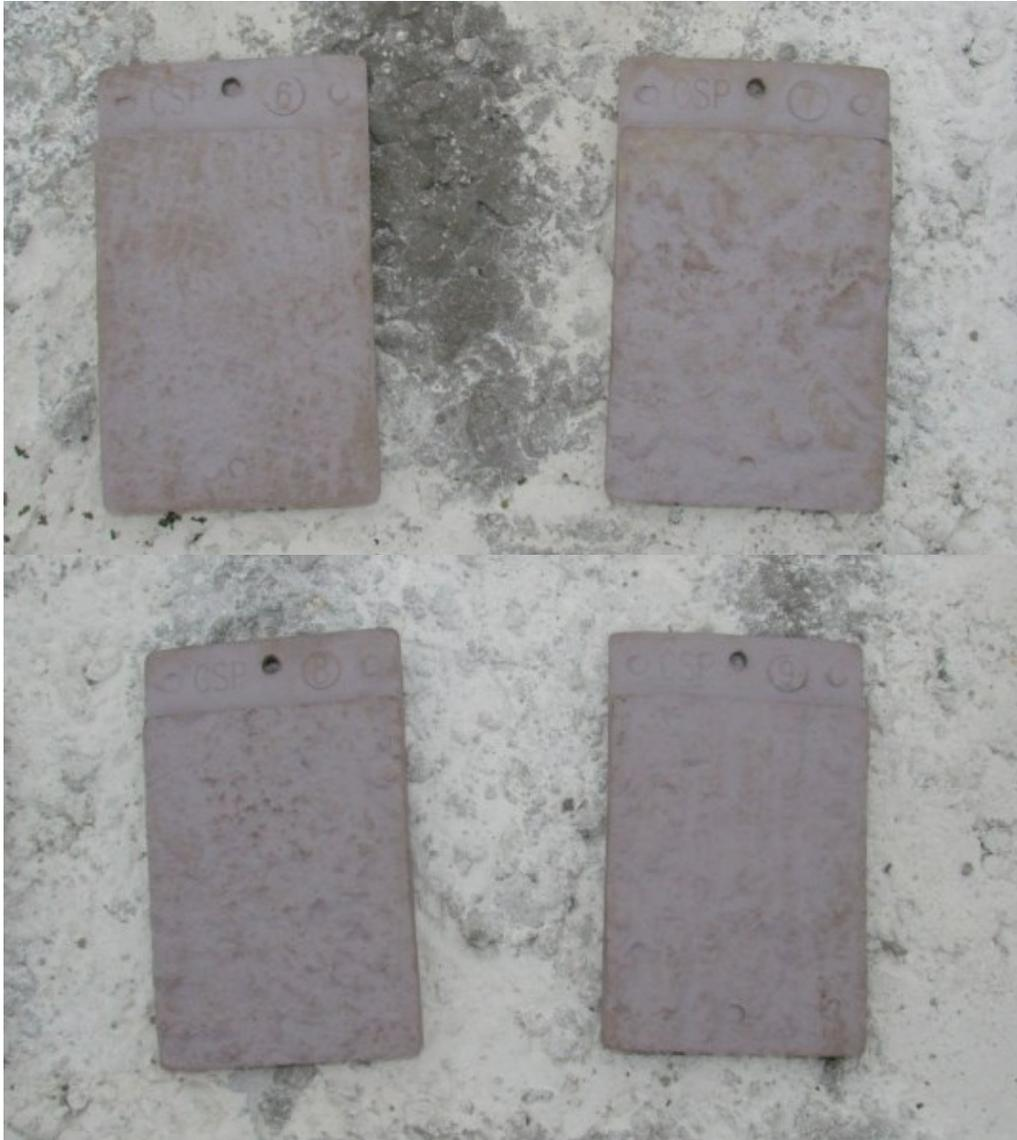
Figure 174. Box beam surface roughness compared to CSPs
