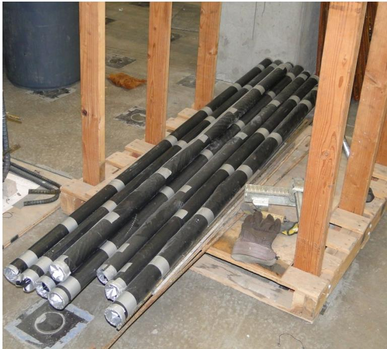
Figure 15. Long Horizontal pvc pipes used for lifting.
