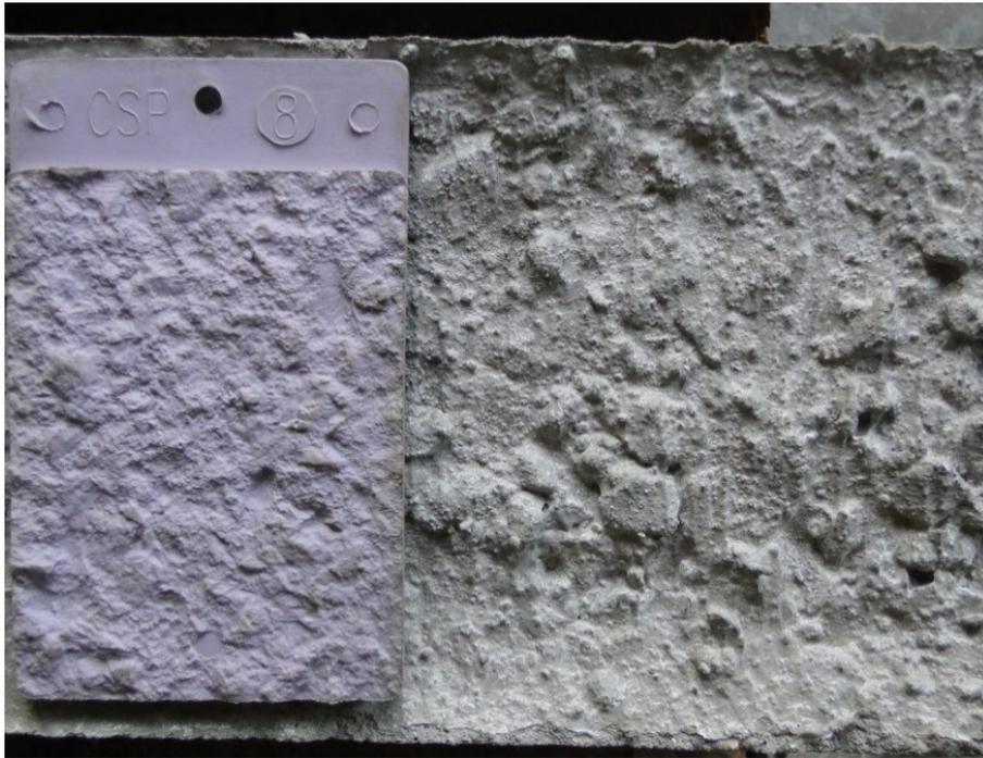
Figure 205. CSP 8 finish using the modified method of preparation
