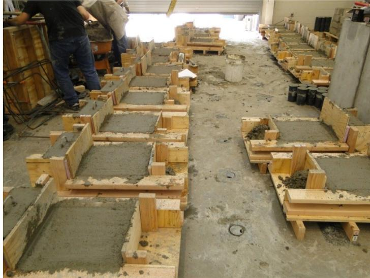
Figure 214. Finished specimens
