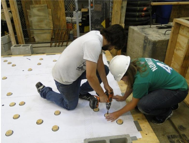
Figure 10. Drilling the wooden discs to the plywood
