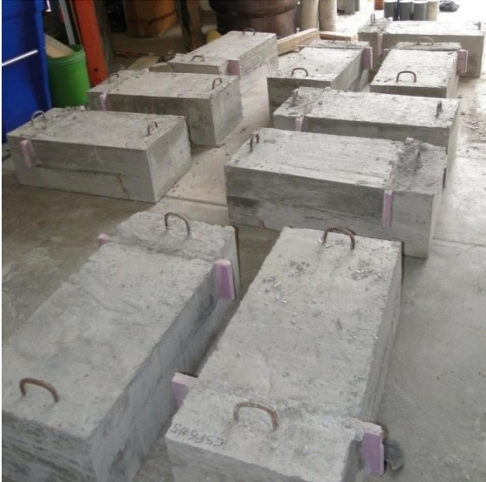
Figure 218. Demolded specimens
