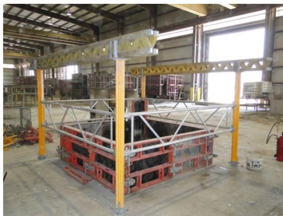
Figure 68. Bottom block and frame setup
