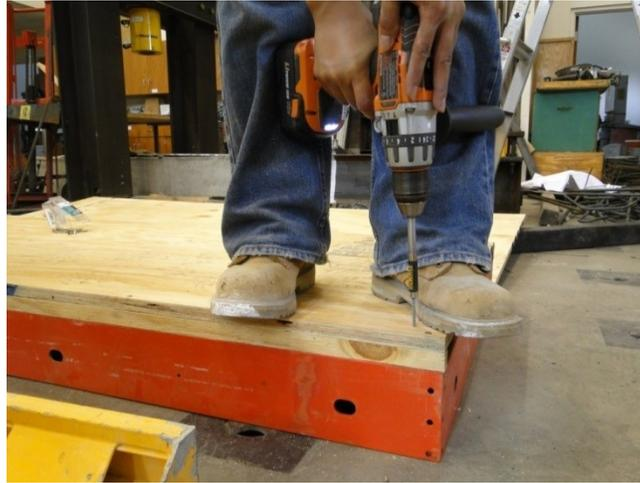
Figure 65. Drilling plywood to the edge strips
