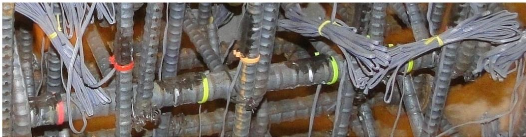
Figure 8. Orientation of strain gauges on longitudinal Bar 4 (on top ridge)
