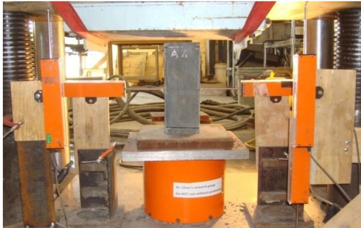
Figure 41. Test setup with LVDTs and load cell
