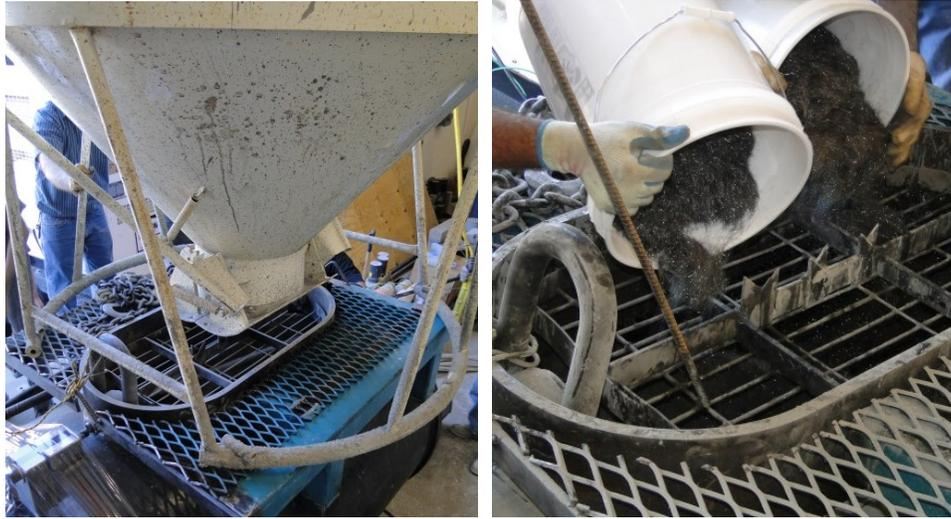
Figure 66. Pouring dry material and addition of micro-fibers
