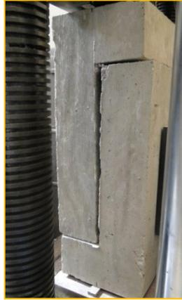
Figure 45. CSP 9 Specimen #3 failure front view
