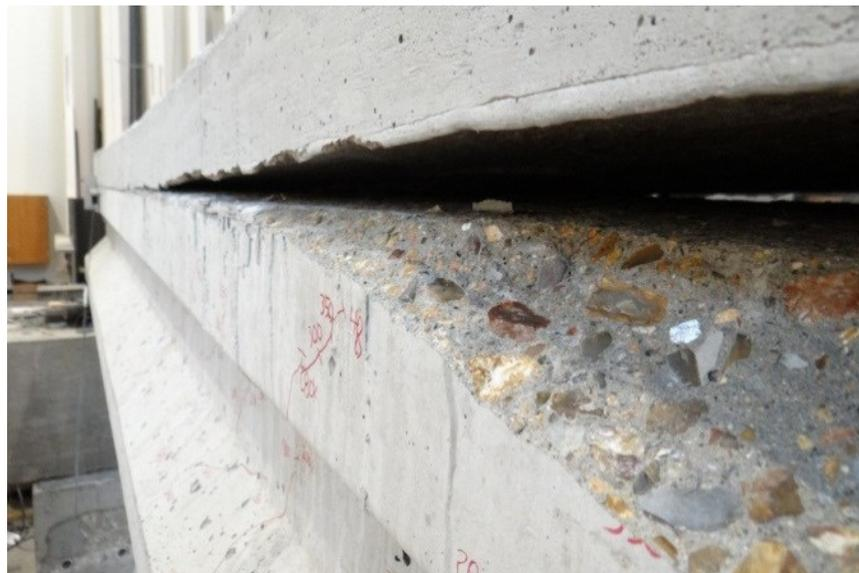
Figure 318. Flexural/ horizontal shear failure near midspan
