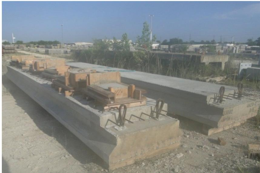
Figure 249. Finished box beam specimens
