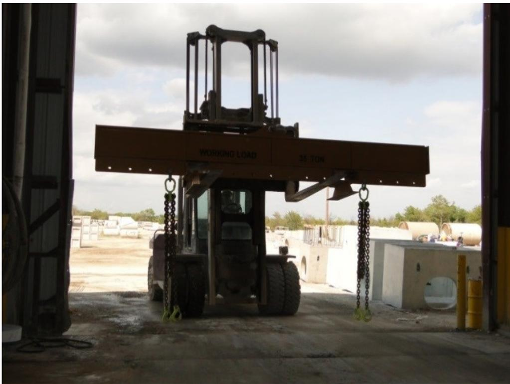
Figure 145. Spreader beam
