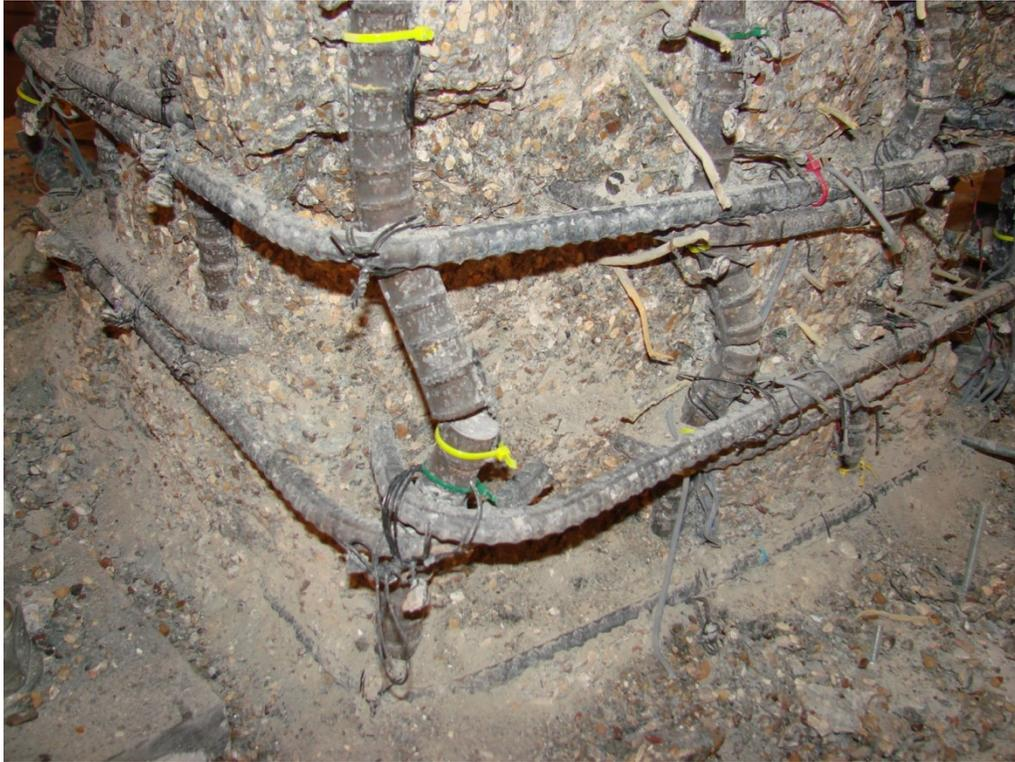
Figure 136. SP5 bar buckling and rupture
