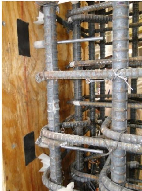
Figure 91. Inserting LVDT rods through the column formwork
