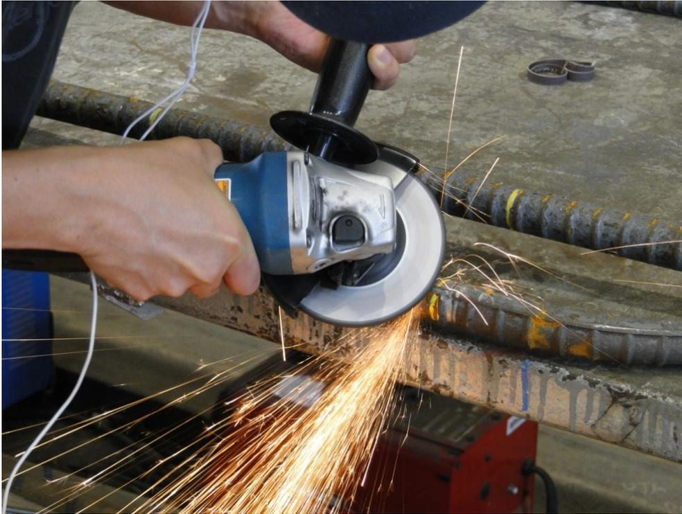
Figure 72. Grinding of the reinforcing bars
