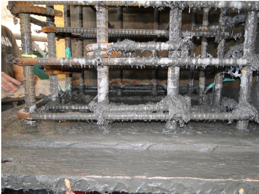
Figure 69. UHP-FRC section after casting
