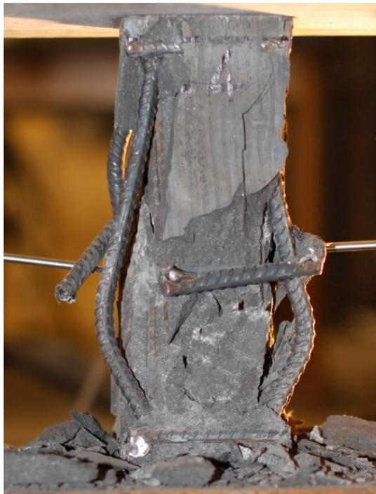
Figure 44. Crushing of specimen A4
