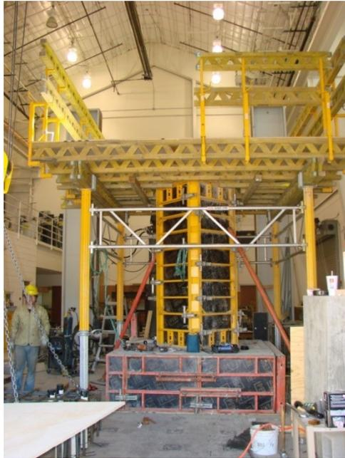
Figure 164. Column Formwork and Loading Block Platform
