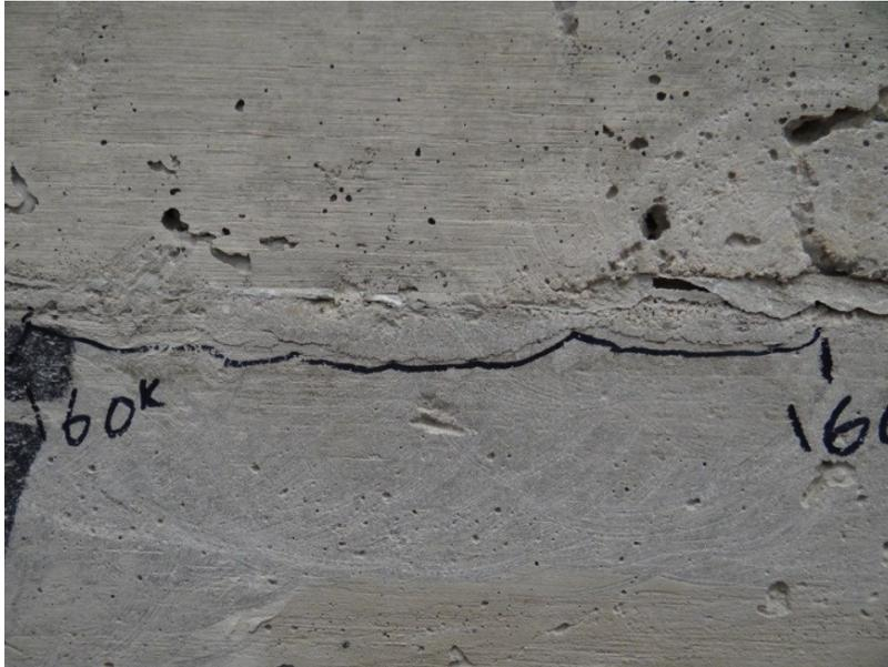
(a) Crack on the East-end of beam
