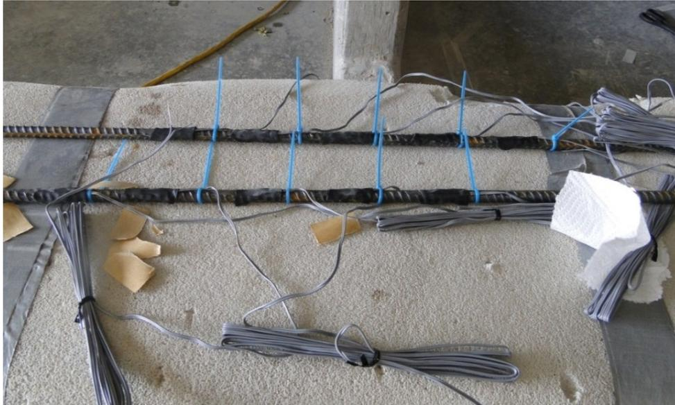
Figure 234. Strain gauges on longitudinal reinforcement
