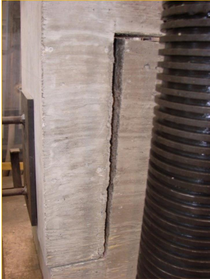
Figure 39. CSP 9 Specimen #1 failure
