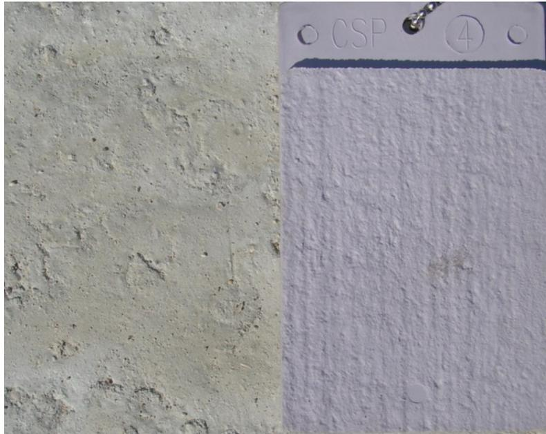
Figure 283. Surface finish on SCC slab beams comparable to CSP 4
