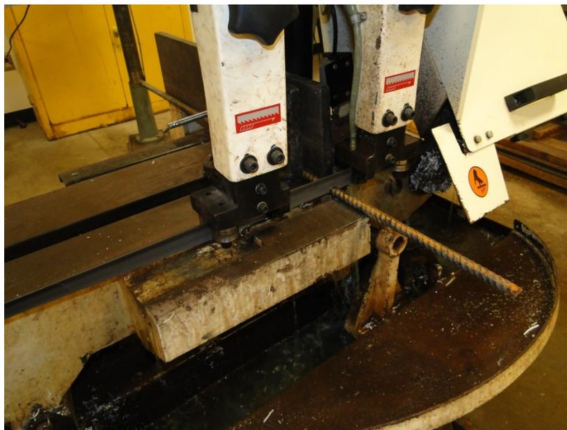
Figure 13. Cutting reinforcing bars for bottom block grid
