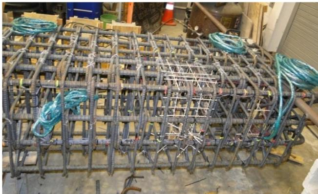
Figure 69. Completed gauge instillation
