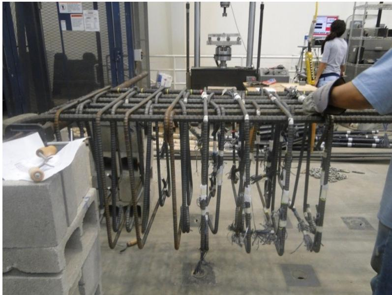
Figure 38. Transverse reinforcement with strain gauges
