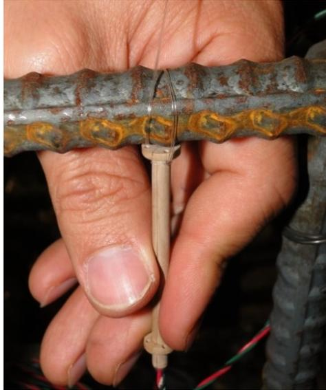
Figure 61. Placing of concrete gauge
