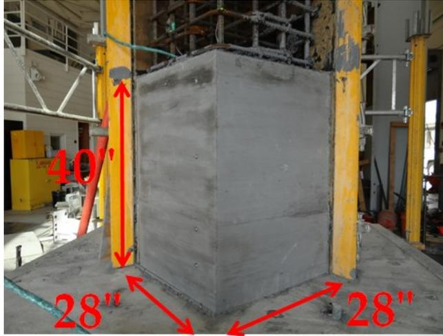
Figure 182. 40" UHP-FRC Section After demolding
