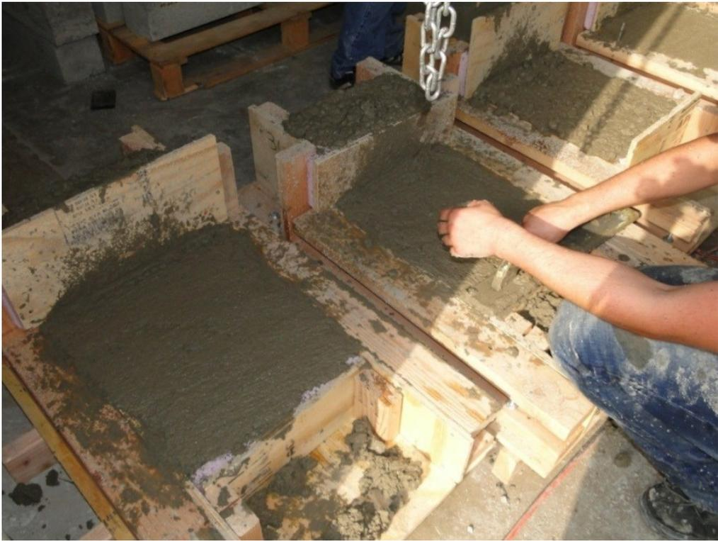
Figure 208. Wood float finish on all specimens
