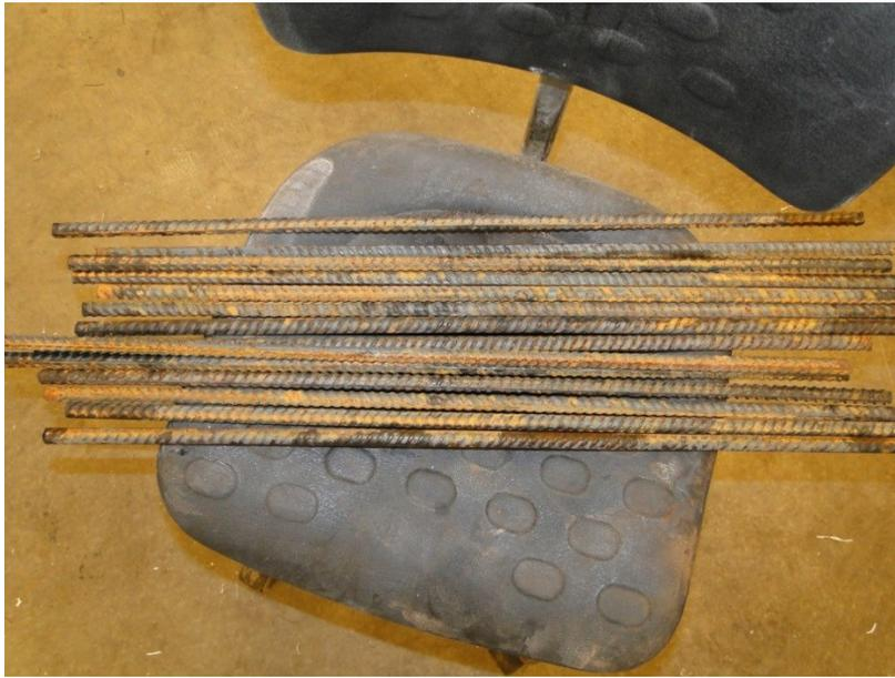
Figure 14. Cut reinforcing bars for bottom block grid
