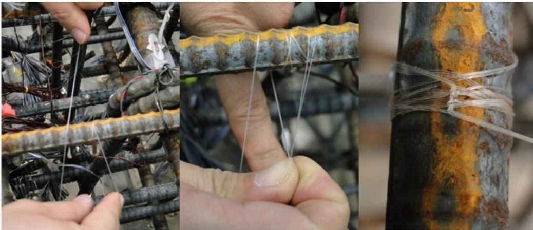
Figure 64. Securing gauge to bar
