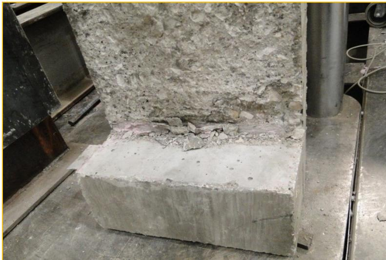
Figure 32: Failure into the CIP at the notch.
