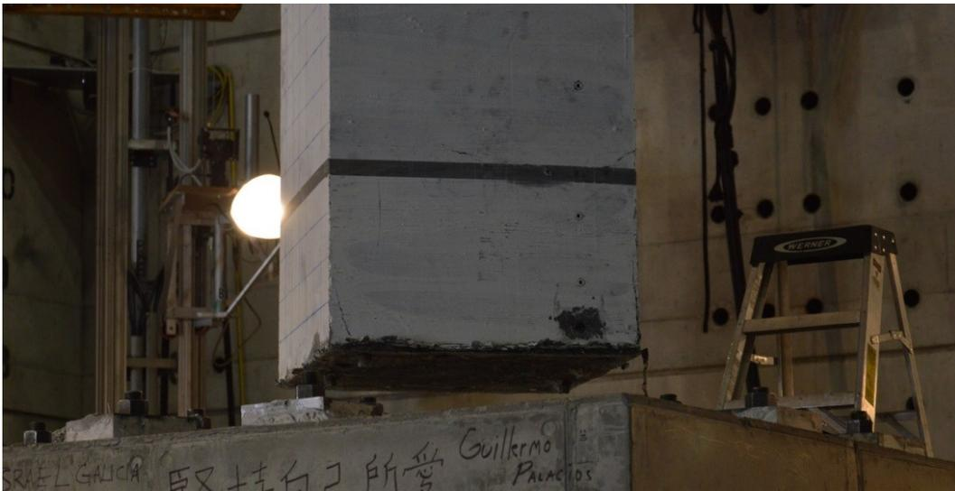
Figure 101. SP8 column specimen after testing
