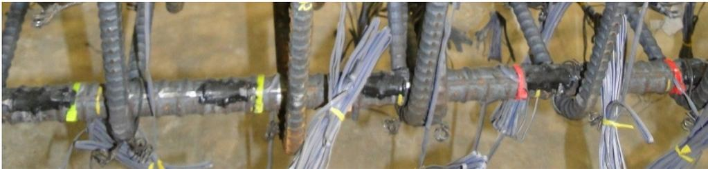
Figure 5. Orientation of strain gauges on longitudinal Bar 1 (on top ridge)
