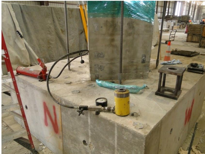
Figure 140. Post tensioning equipment
