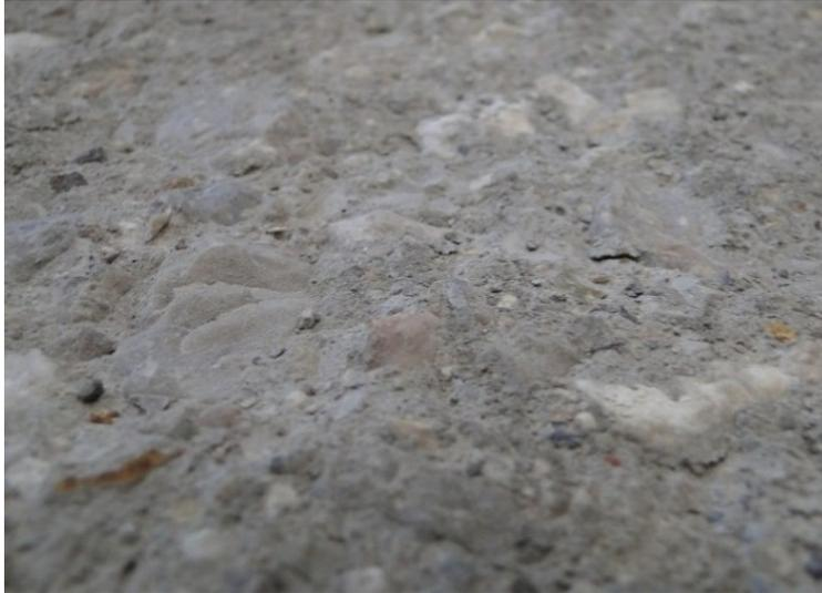
Figure 310. CSP 6 Specimen precast surface profile
