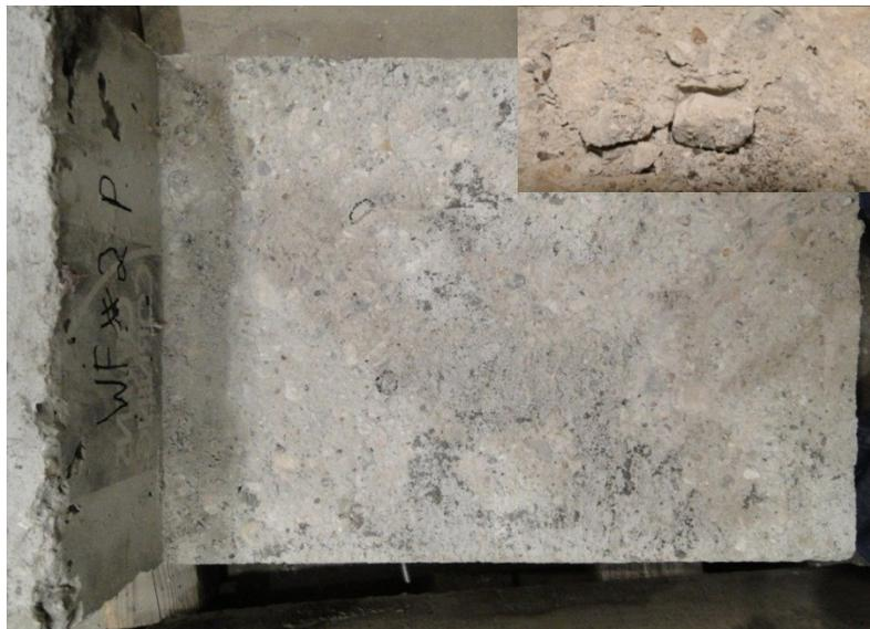
Figure 309. Precast failure plane showing dislodged aggregate
