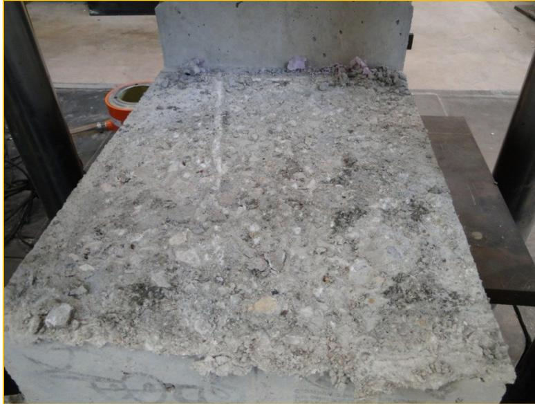
Figure 4. Wood float specimen # 1 precast failure plane showing aggregate pullout.
