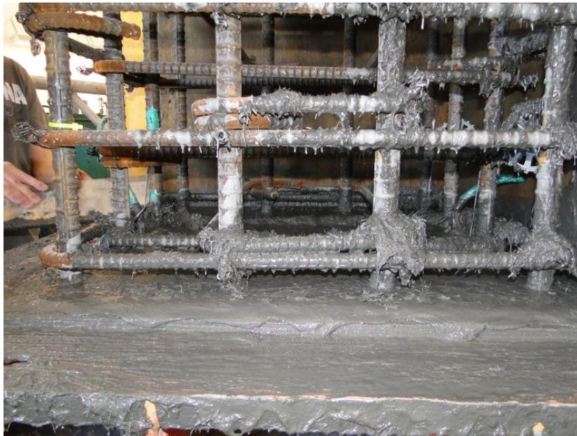
Figure 181. UHP-FRC Section after Casting
