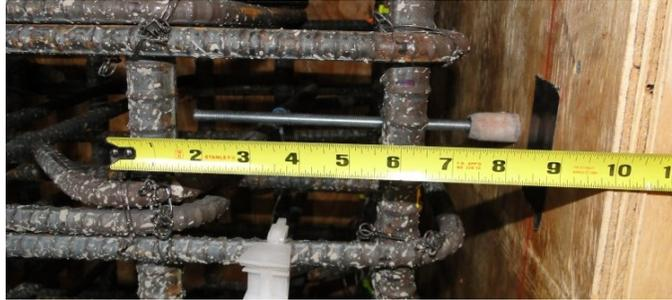
Figure 96. 10" embedment of LVDT rods
