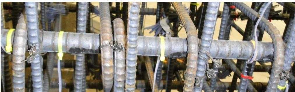
Figure 6. Orientation of strain gauges on longitudinal Bar 2 (on bottom ridge)
