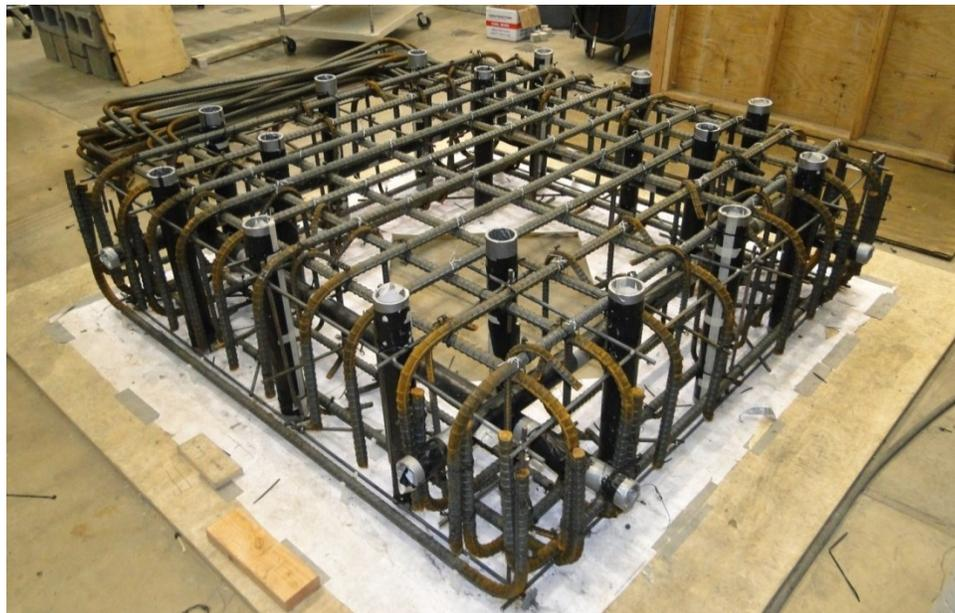
Figure 62. Completed top block cage
