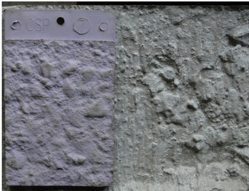
Figure 204. CSP 7 finish using the modified method of preparation
