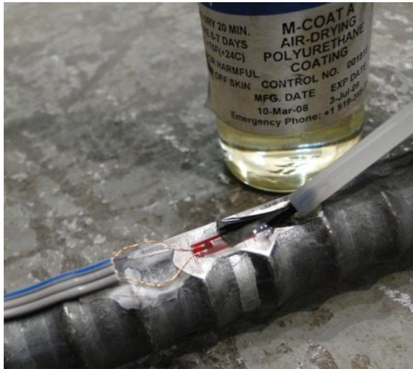
Figure 74. Application of coat A
