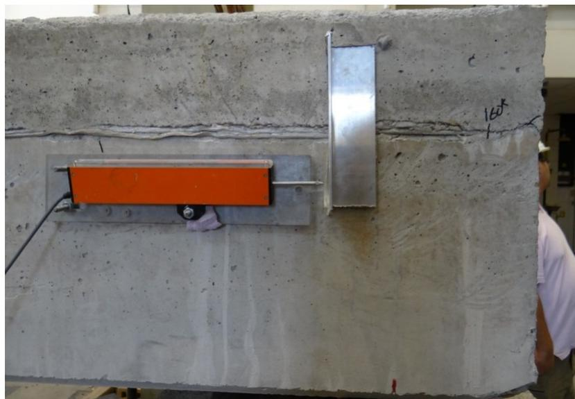
(b) Crack on the East-edge of beam
