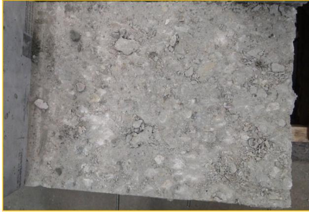
(a) Dislodged concrete and aggregates.
