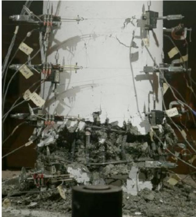
Figure 31. Specimen S1 after 10.7% drift ratio (Aviram et al., 2010).
