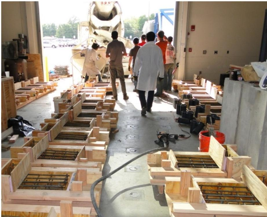
Figure 207. Specimen formwork
