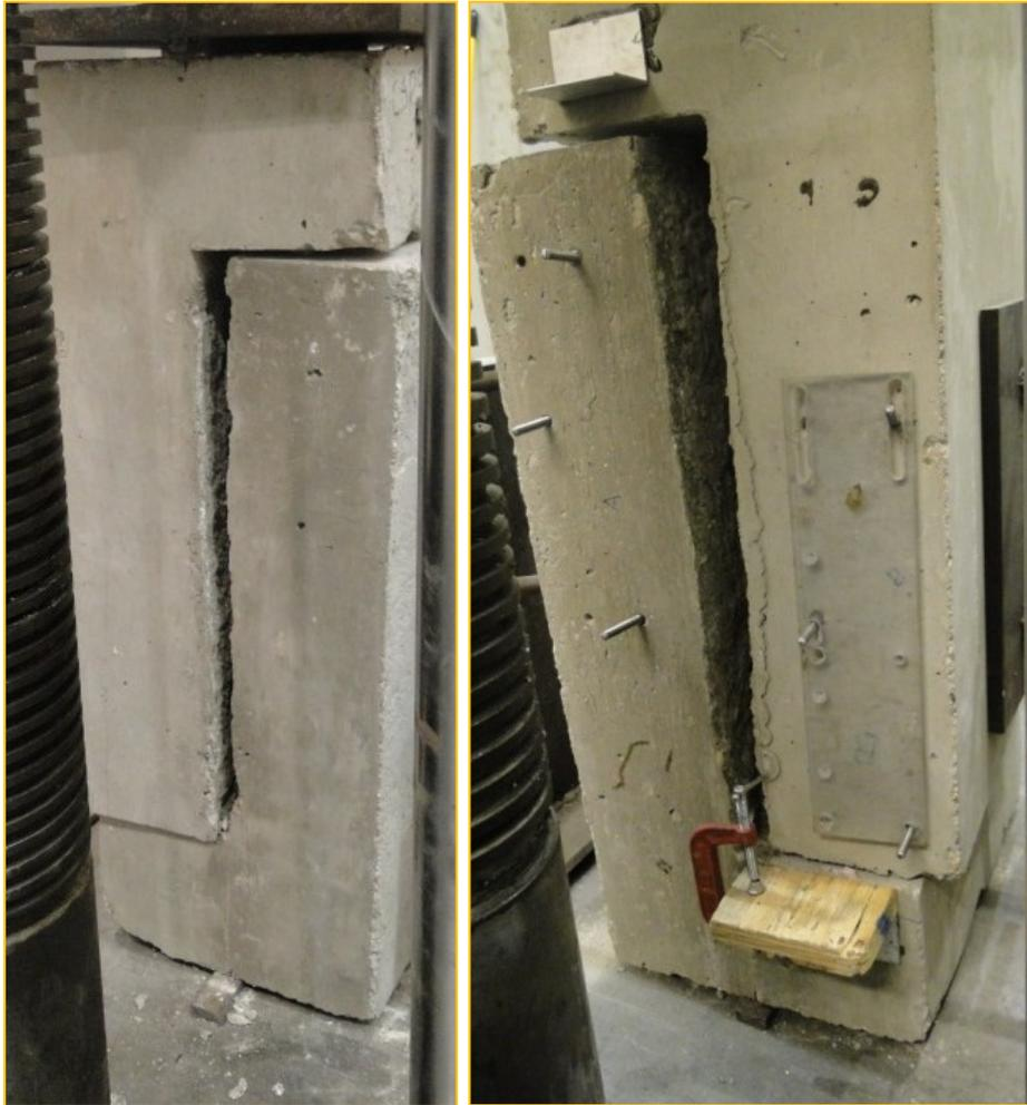
Figure 42. CSP 9 Specimen #2 failure (a) front view (b) back view.
