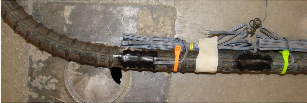
Figure 2. Location of strain gauge on longitudinal rebars
