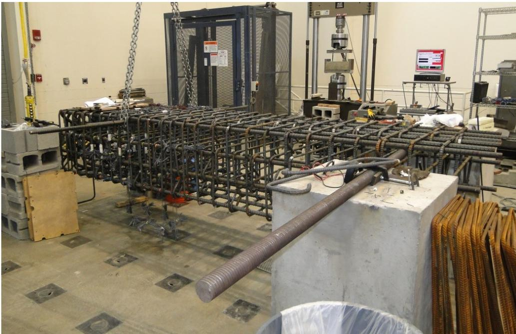
Figure 52. Side view of the completed tied column cage
