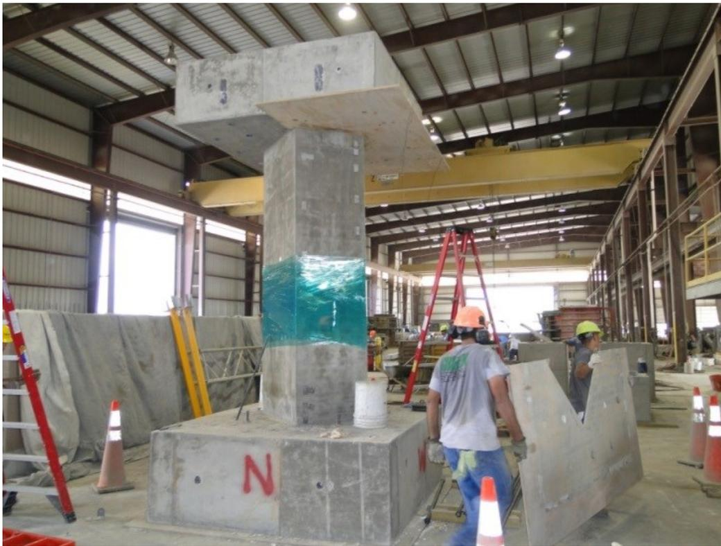
Figure 136. Wrapping wires to column section
