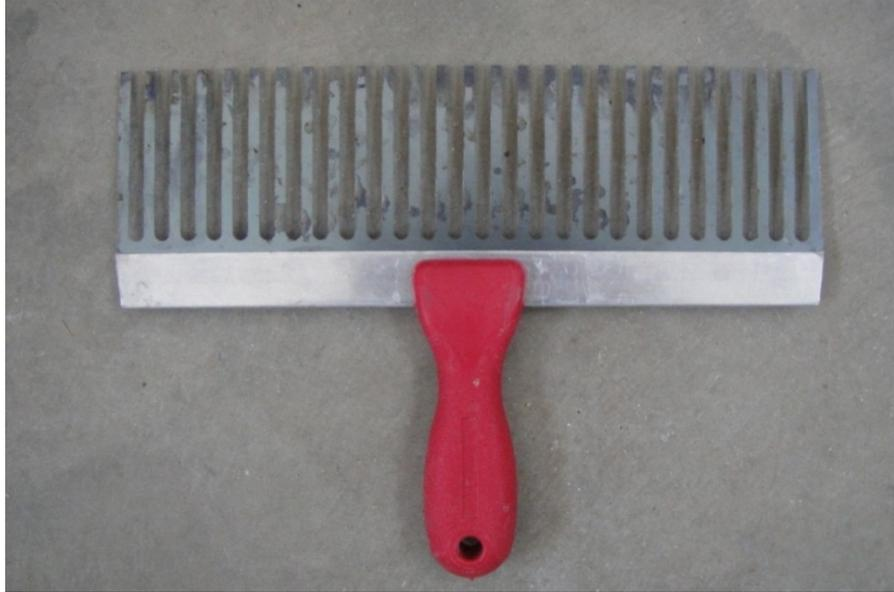
Figure 198. Concrete rake
