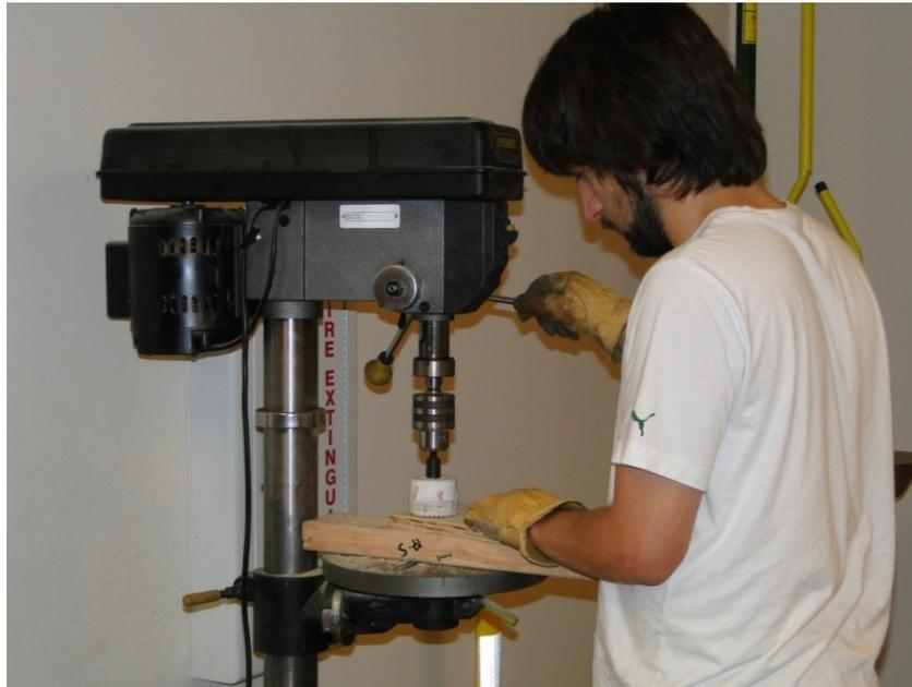
Figure 7. Cutting the wooden discs
