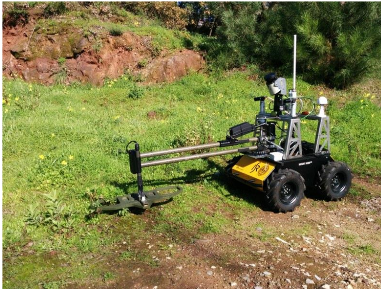
Figure 3-2 (a) The Vallon VMP3 metal detector (b) The VMP3 installed on the Husky robot [26]
