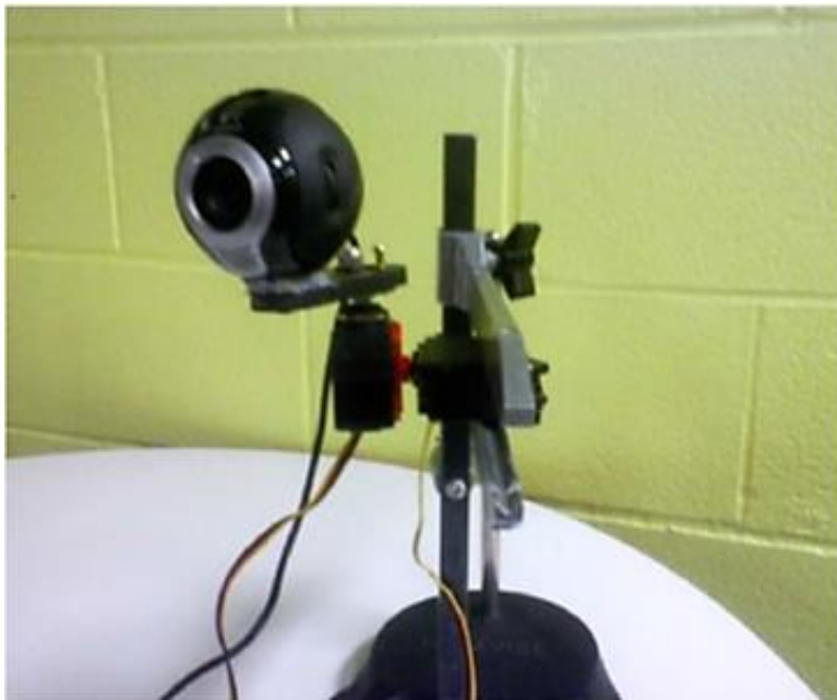
Figure 2-4 Pan and tilt servoing using visual based target tracking [6]
