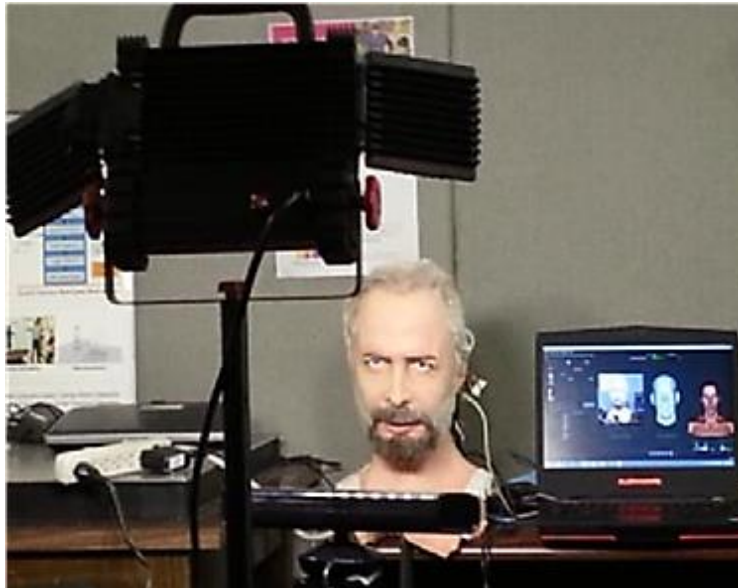
Figure 4-5 Experimental setup used for data collection in which lighting and Kinect sensor position relative to PKD are carefully controlled
