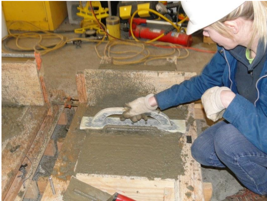
Figure 4-26 Wood float finish on all specimens
