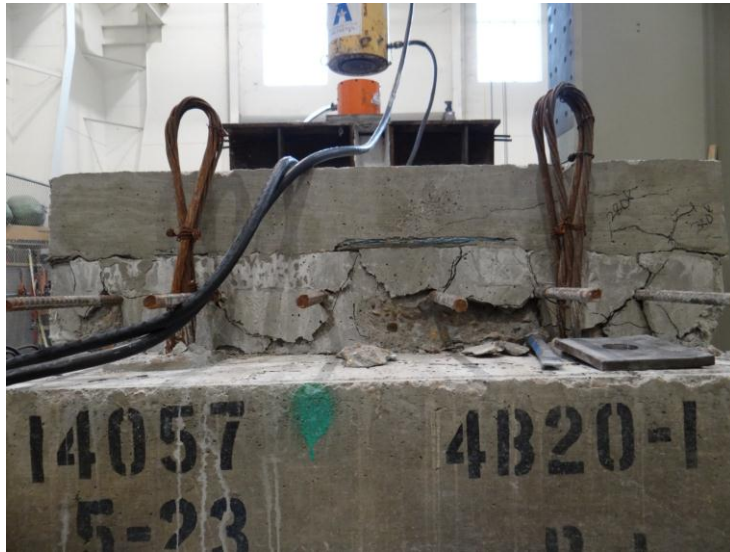
Figure 5-55 Fracture of concrete at East-end
