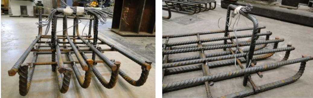
Figure 4-21 Caging for precast part of specimen
