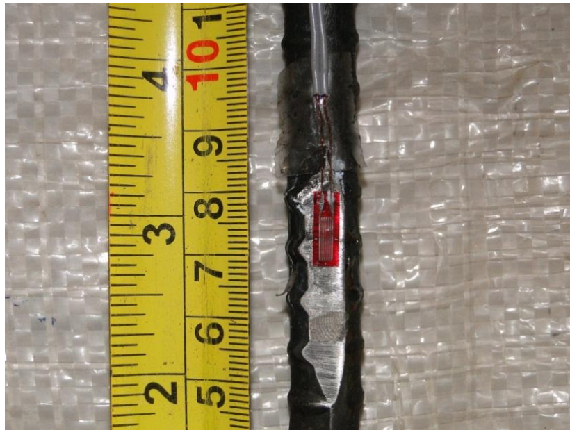
Figure 4-31 Mounted strain gauge
