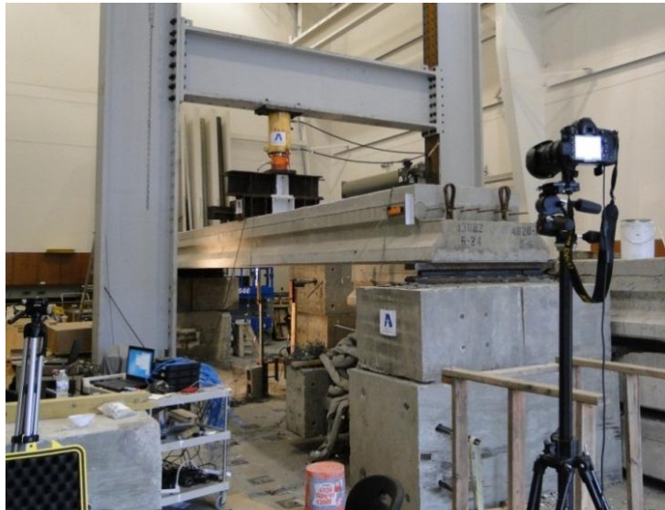
Figure 5-21 21 Box beam (4B20#1) elevation view of test set-up
