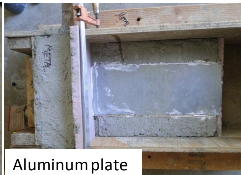
Figure 4-91 Push-off specimen with foam tape, aluminum strip and Styrofoam to reduce interface area
