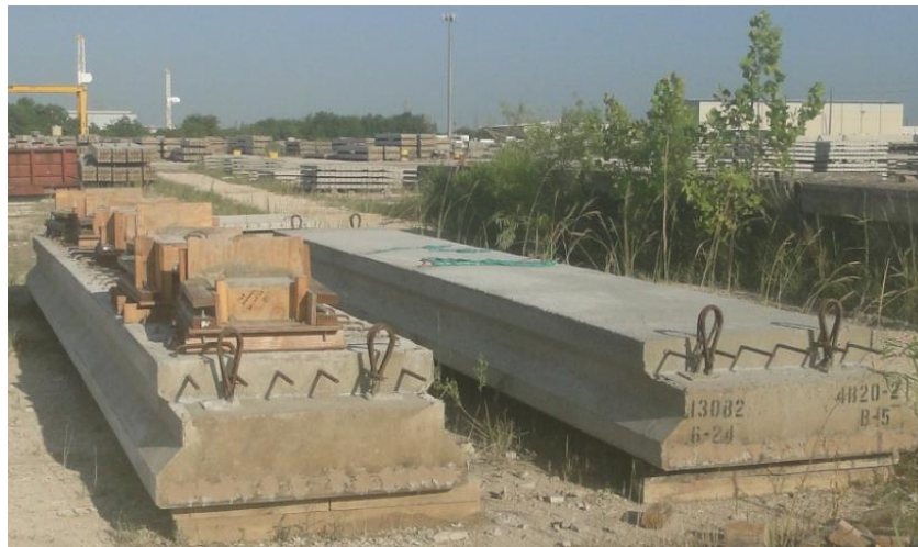
Figure 4-49 Finished box beam specimens
