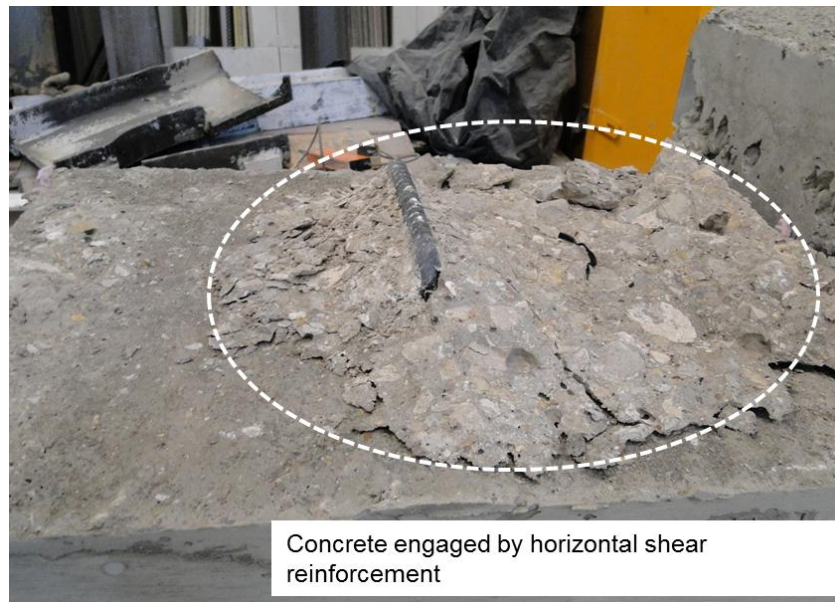
Figure 6-1 Typical failure mode of push-off specimens with 2-in. embedment
