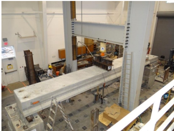
Figure 5-27 Overall test setup of specimen (top view)
