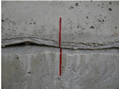
Figure 5-43 Interface slip at 180 kips
