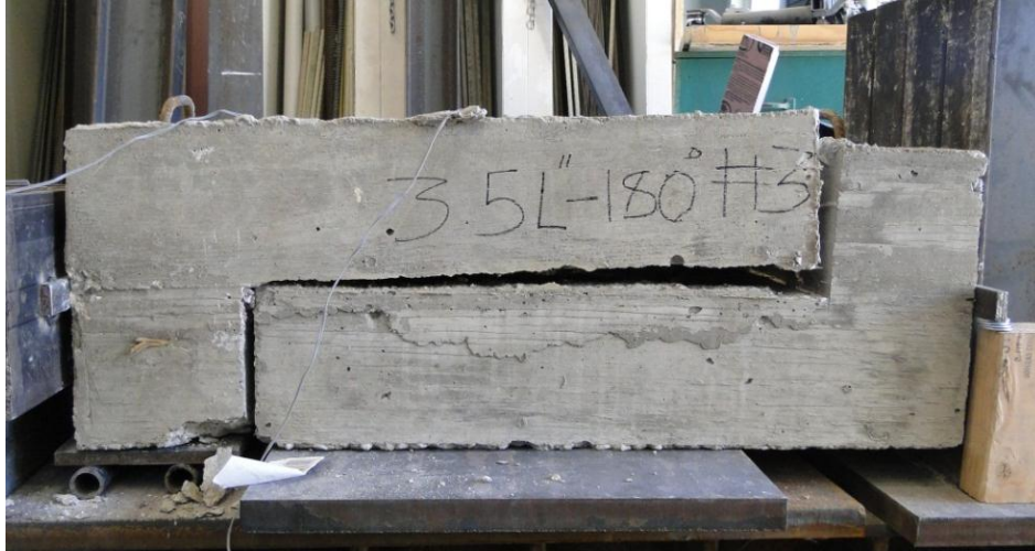
Figure 5-1 Typical failure mode of push-off specimen failure with a 2-in. embedment; bar pulled out from the CIP slab
