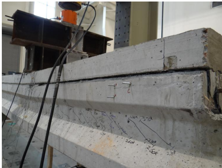
Figure 5-56 Separation between the CIP slab and precast beam
