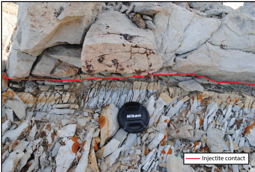
Figure 12 – Red alteration halos along the systematic Mowry joint sets and parallel injectite contact at Injectite #1. The staining is more pronounced near the injectites. Sub-vertical closely-spaced fractures terminating against the injectite are along sedimentary laminations in the Mowry formation.
