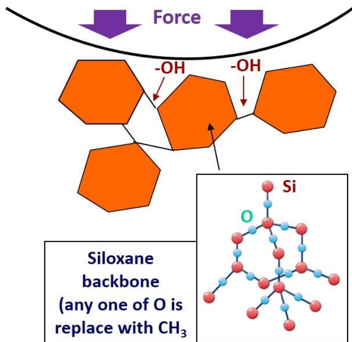
Fig. 3.4 Schematic illustration of a chain of weak links in the backbone network
