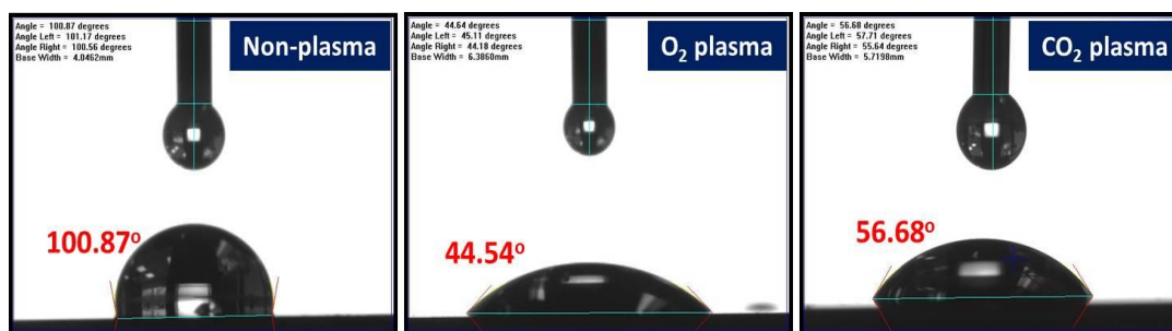
Fig. 3.3 Variation of contact angle depending on plasma exposure
