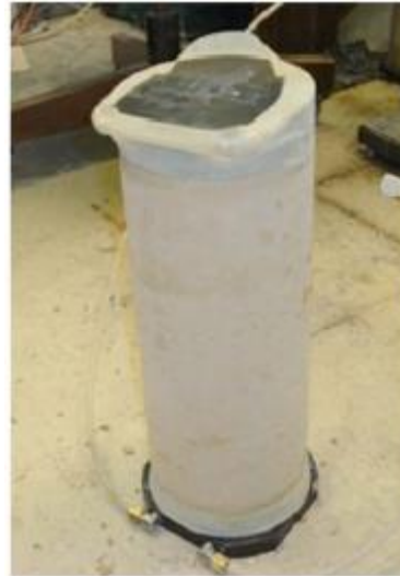
Figure 2-32 Geogrid reinforced triaxial sample (Abu-Farsakh et al. 2012)
