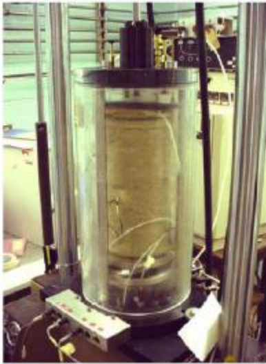
Figure 2-31 Triaxial testing set up of geogrid reinforced sample (Abu-Farsakh et al. 2012)
