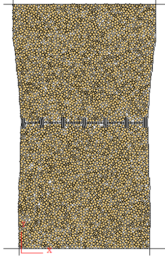
Figure 4-40 Reinforced sample at 5 % axial strain loaded at 0.005 m/s
