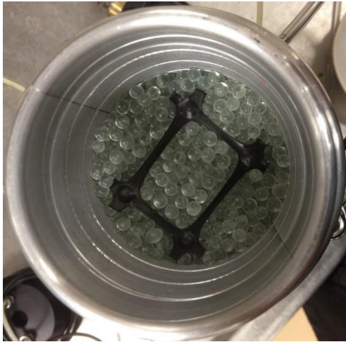
Figure 3-6 Position of geogrid in the sample
