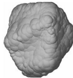
Figure 2-42 Clump particle representing realistic aggregate shape (Ferrellec and McDowell 2010)
