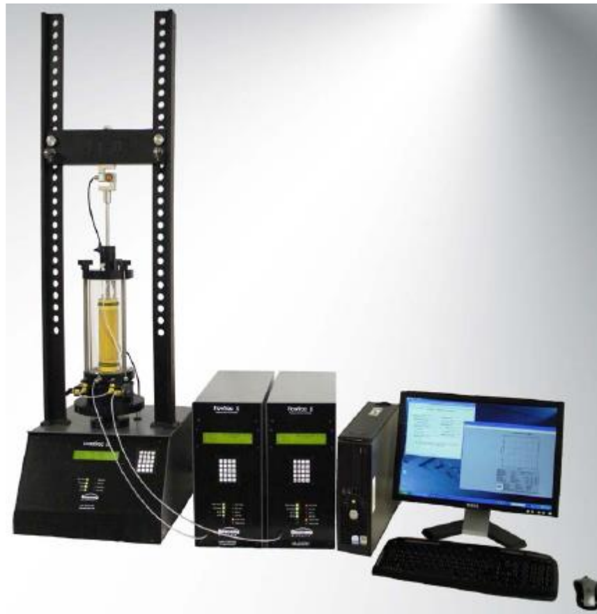
Figure 3-5 Triaxial testing equipment FlowTrac II from Geocomp
