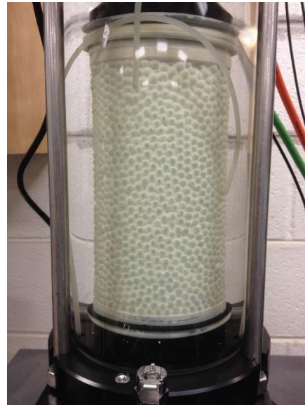
Figure 3-9 A triaxial sample of glass beads in a triaxial cell
