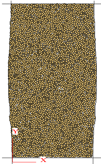
Figure 4-25 Unreinforced circular biaxial sample at 5 % axial strain with flexible boundary loaded at 0.005 m/s
