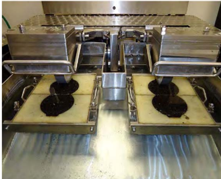
Figure 2-14 Hamburg Wheel rut tracking
