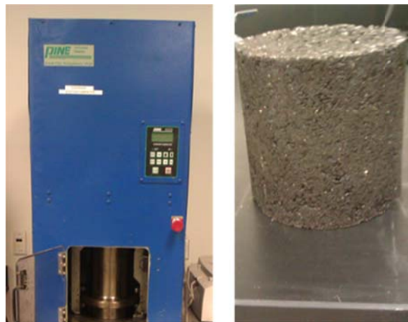
Figure 4-1 Compaction of HMA specimen using Super-pave Gyrotory Compactor
