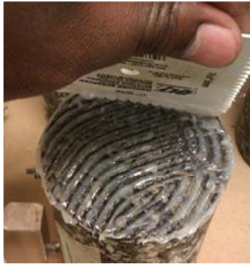
Figure 4-14 Uniform spreading of epoxy glue on sample surface
