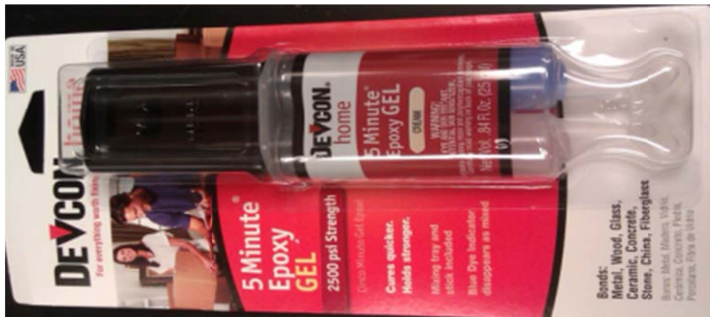
Figure 4-13 High strength epoxy glue used in the tension test
