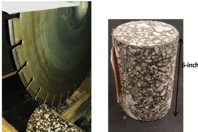
Figure 4-3 Trimming of HMA specimen ends using circular saw
