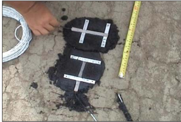
Figure 3-8 Texas Measurement Gauges Model PML-120-2L
