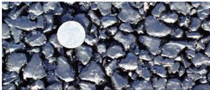
Figure 2.7 Close-up view of Perpetual Pavement wearing course with OGF mix
