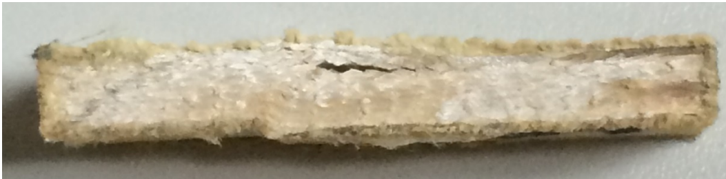
Figure 4-4: Kevlar Test Specimen from Compression Tests
