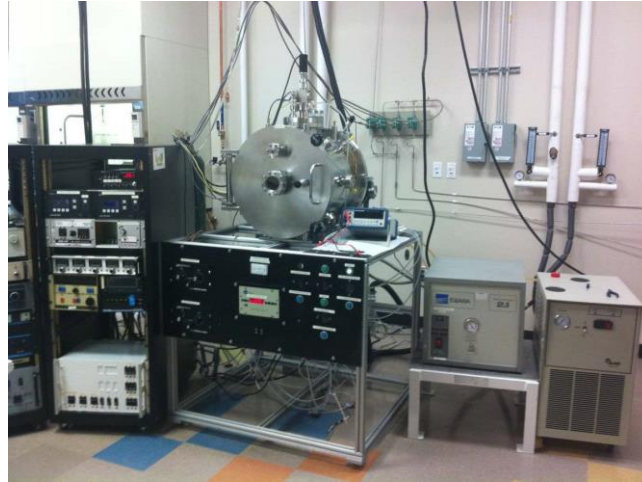
Figure 3.2 Lab-Built PVD reactive magnetron sputtering system in Surface and Nano Engineering Laboratory
