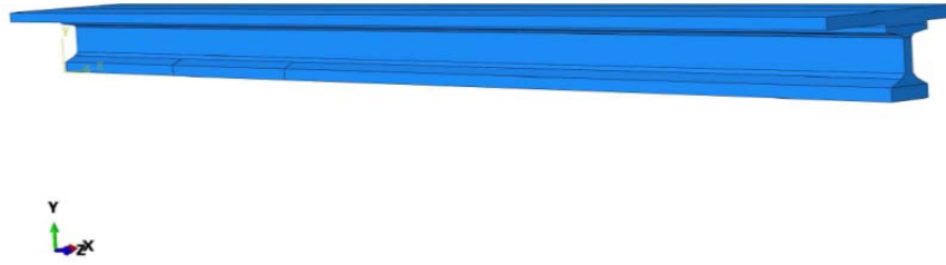
Figure 5-27 ABAQUS Concrete Repaired Section
