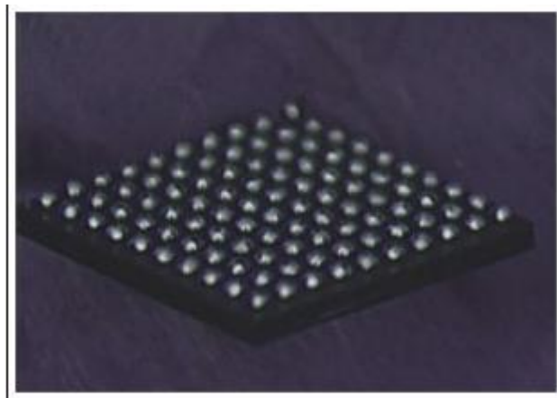
Figure 1-6 10 x 10 WLP with circuit side view
