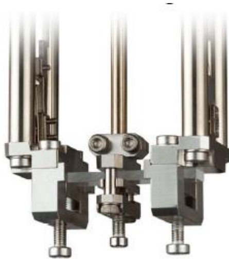
Figure 3-11 Bending Fixture for DMA
