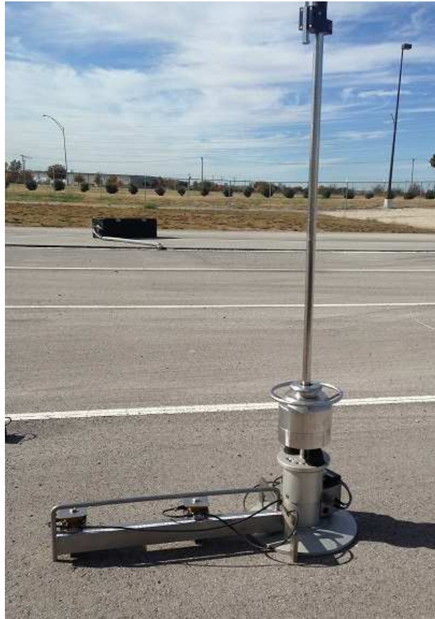
Figure 2-5 PRIMA100 With Two Additional Geophones
