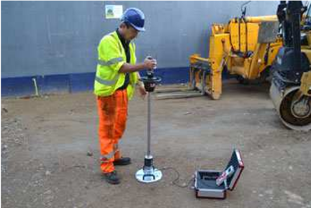
Figure 2-4 Light Weight Deflectometer With a Single Geophone
