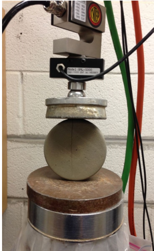
Figure 3-58. Indirect tensile strength test (IDT) on dry soil specimen
