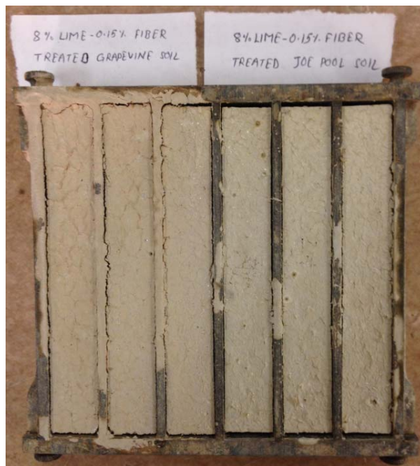
Figure 5-42 Linear shrinkage bar test on the lime+fiber treated soils
