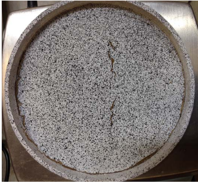
Figure 3-21 Cracking of 8% lime treated Grapevine soil at the end of the test
