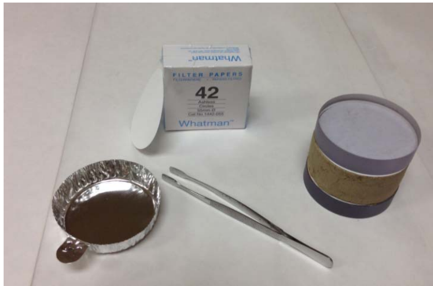
Figure 3-42 Filter paper technique for measuring matric suction
