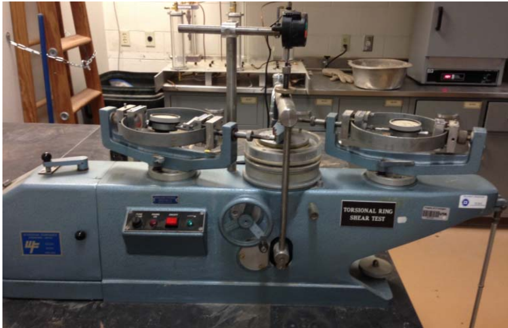
Figure 3-9 Bromhead ring shear device and test setup
