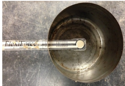
Figure 3-63 Horizontal orientation of the sensor inside the moisture can
