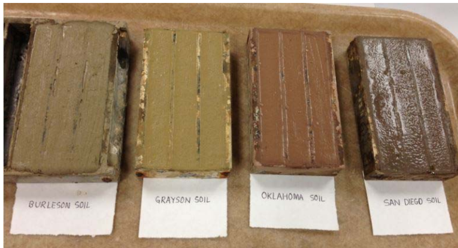
Figure 3-89 Soil specimens kept in the mold for linear shrinkage bar test
