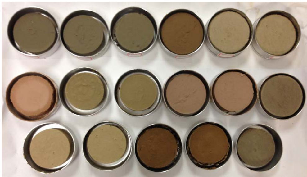
Figure 3-57 Slurry soil specimens dried in air and made ready for testing
