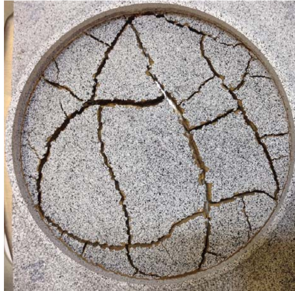
Figure 3-19 Cracking of the Grapevine soil at the end of the test
