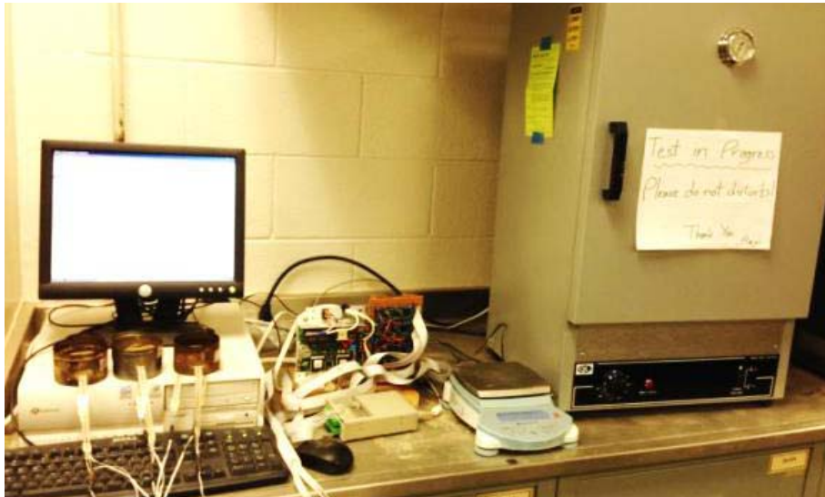
Figure 3-65 SIP test setup for the oven drying method
