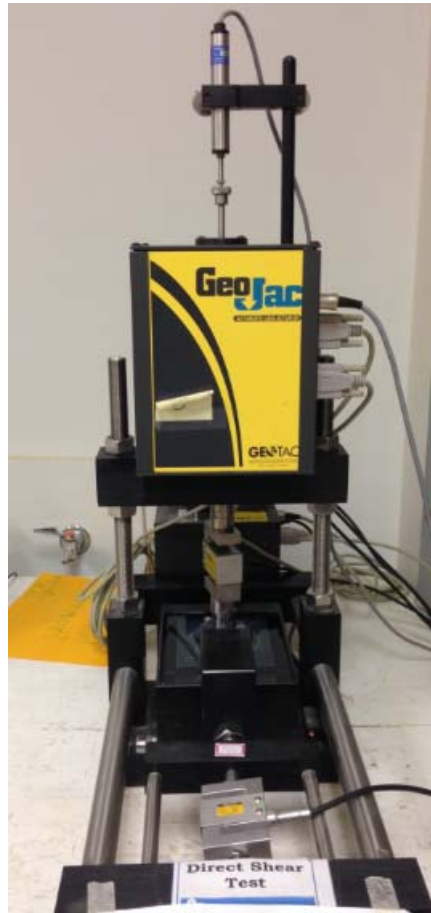
Figure 3-7 Direct shear test apparatus used in this study
