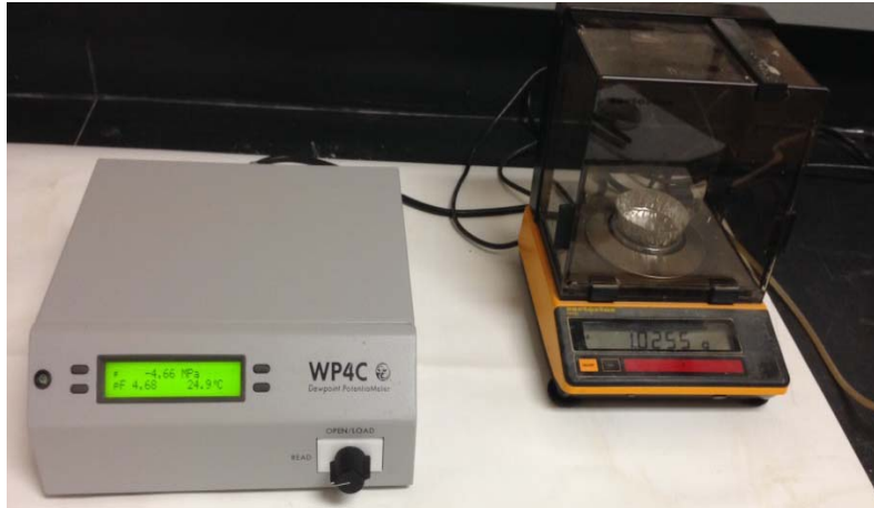
Figure 3-45 WP4C Potentiometer and precision balance used in the measurement of soil suction
