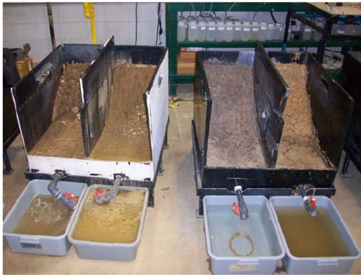
Figure 2-7 Experimental set up to study the erosion of the slope with and without the biopolymer treatment (Larson et al., 2012)
