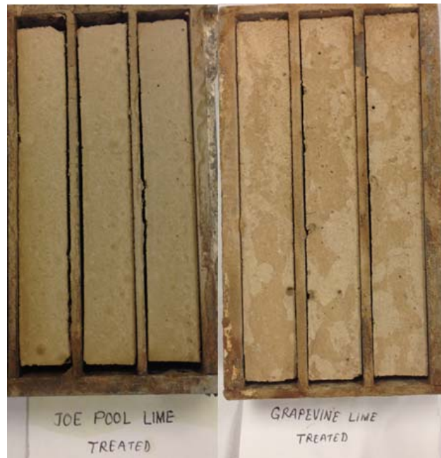
Figure 5-41 Linear shrinkage bar test on lime treated soils
