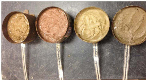
Figure 3-64 Sensors inserted into the soil matrix through the opening on the side wall of the moisture can
