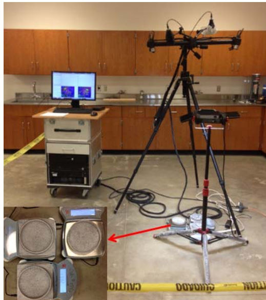
Figure 3-17 3D DIC experimental setup for 3 specimens
