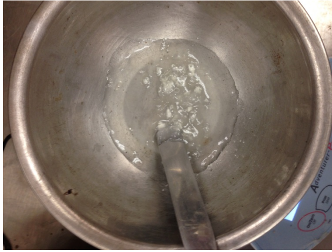
Figure 5-15 Swelling of biopolymer upon adding water
