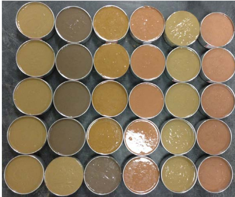
Figure 3-56 Slurry soil specimens molded for IDT
