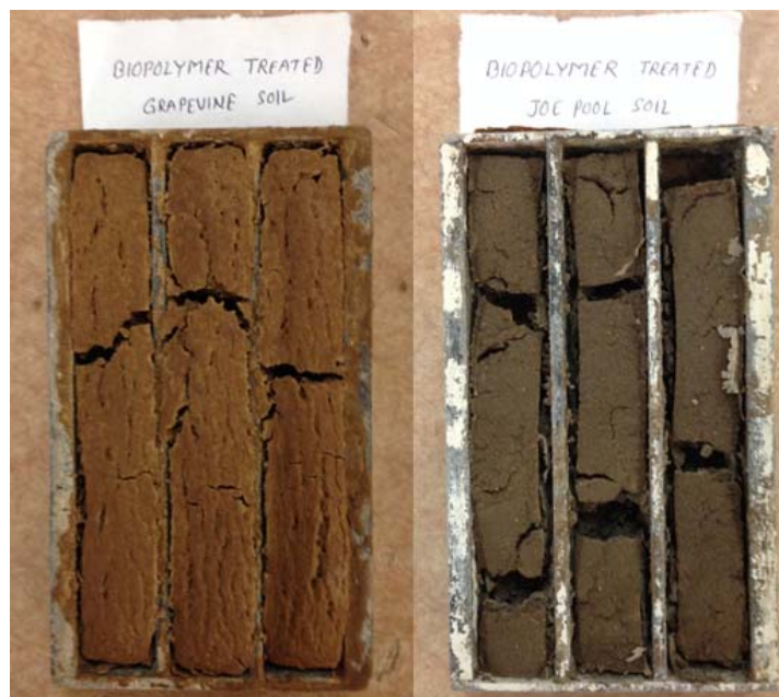
Figure 5-40 Linear shrinkage bar test on the biopolymer treated soils
