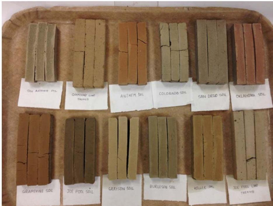
Figure 3-90 Soil specimens after drying in the oven
