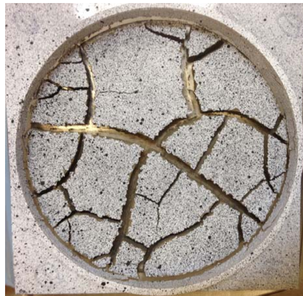
Figure 3-20 Cracking of the Joe Pool soil at the end of the test
