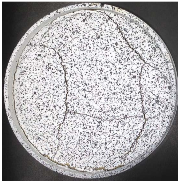
Figure 3-22 Cracking of the 8% lime treated Joe pool soil at the end of the test
