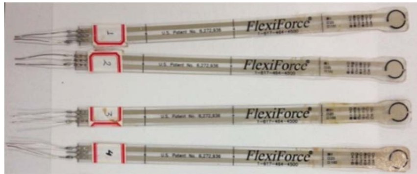
Figure 3-60 The force sensors used in the SIP tests
