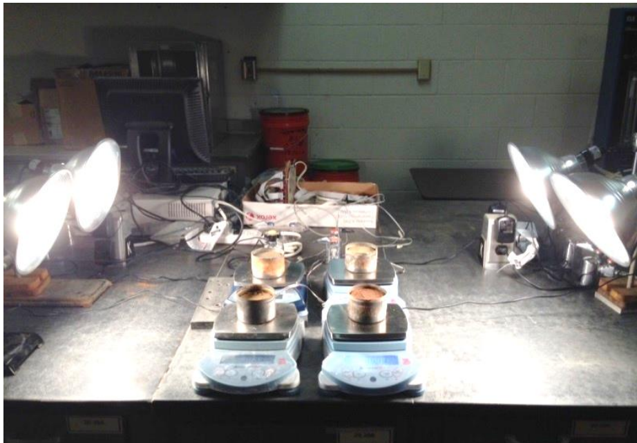
Figure 3-66 SIP test setup by using the heating lamps
