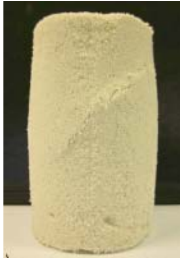
Figure 2-12 Failure mode of a biopolymer treated sand specimen (Khatami and O’Kelly 2013)
