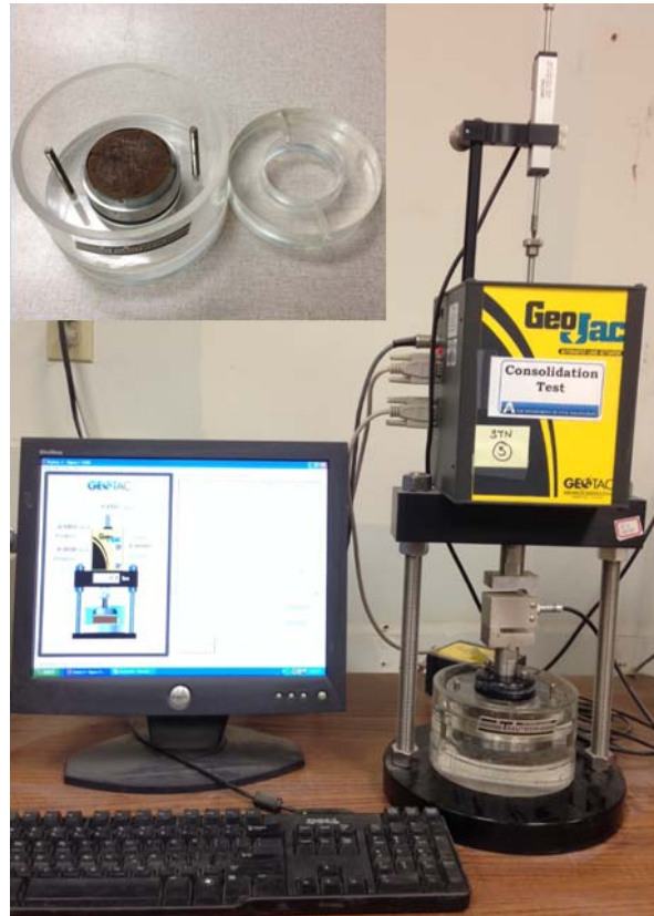
Figure 5-16 Experimental setup for the swell pressure tests
