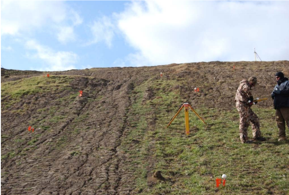
Figure 2-10 Comparison of surface rutting and vegetative growth after 6 months of weathering between control and biopolymer treated section (Larson et al., 2013)
