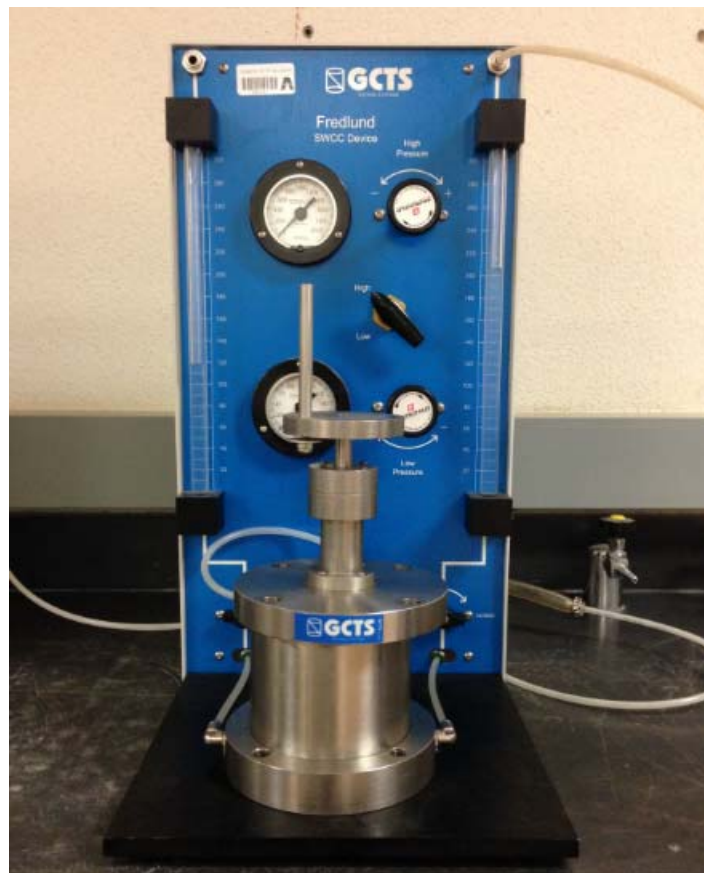
Figure 3-44 Pressure cell apparatus used in the current study
