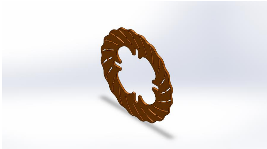
Figure 2-2 Solidworks model of the disk used in simulation
