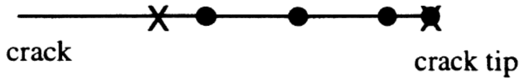
Figure 3.3 Discontinuous crack tip element. Yang, B., and K. Ravi-Chandar.
