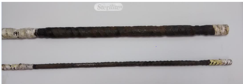
(b) Rebars after cleaning
