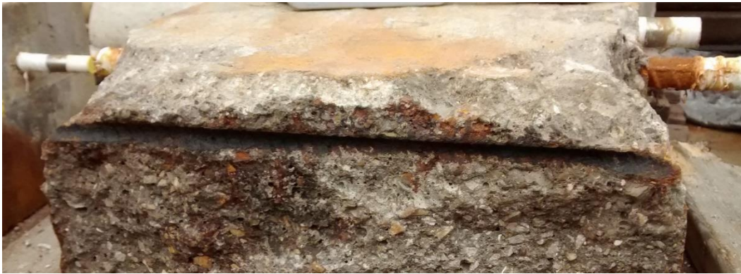
Figure 4-1: Dispersion of corrosion products around rebar
