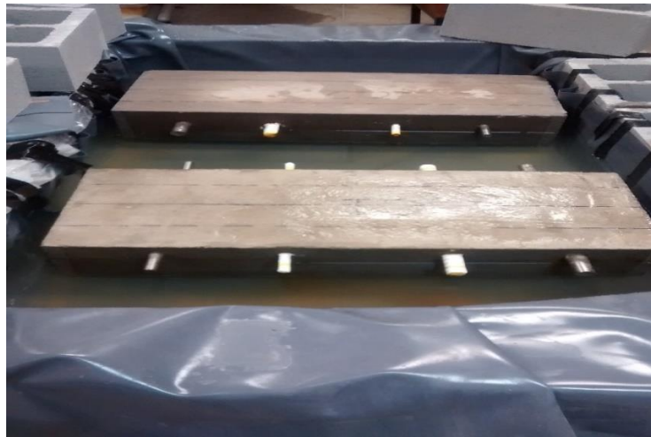
(b) When water level was lowered below rebar level
