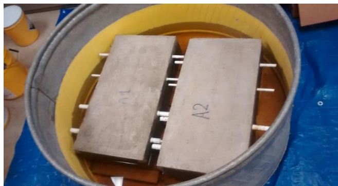
(c) After water level was lowered below rebar level
