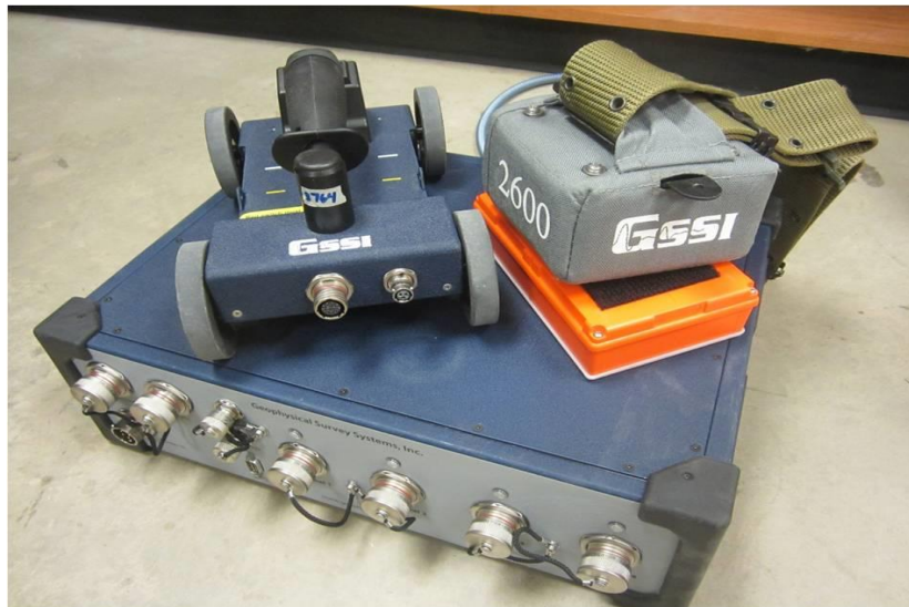
Figure 3-2: GPR equipment (Hasan, 2015)
