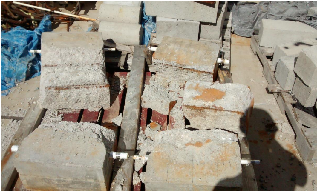
Figure 3-18: Extraction of rebars from the specimens
