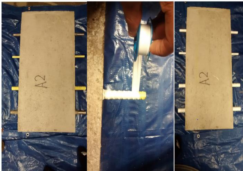
Figure 3-9: Wrapping of rebar ends with Teflon tape
