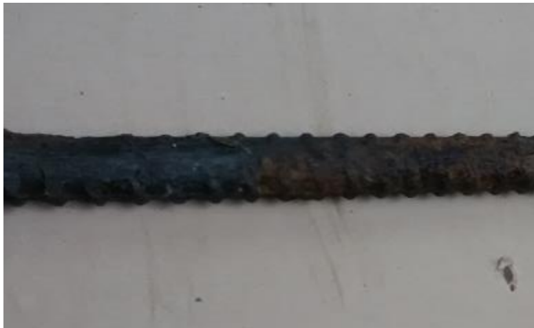
(b) Rebar after cleaning
