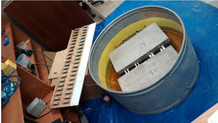
(a) Accelerated corrosion setup
