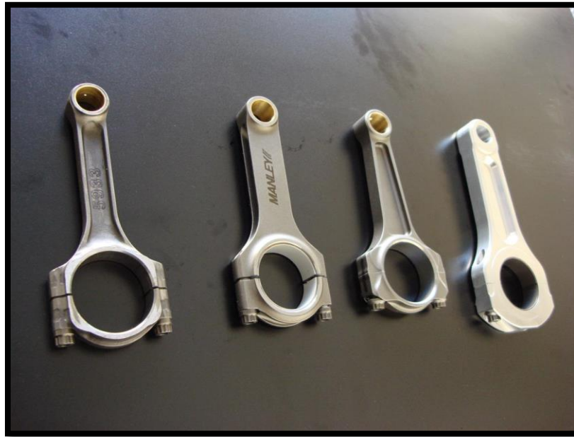
Figure 2.4 Forged steel and Aluminum 7075 as a connecting rod material [9].
