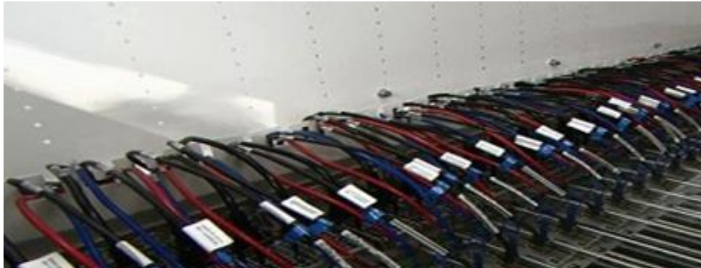
Figure 1-1 Submerging supercomputers into vats of liquid [29]
