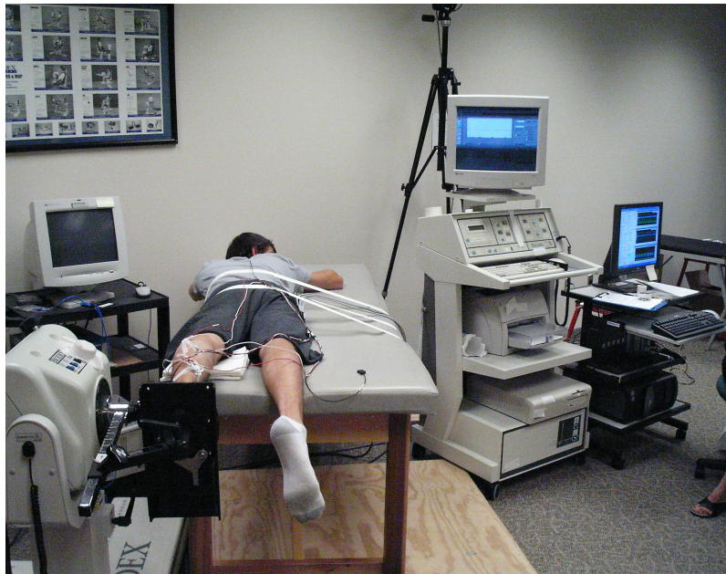
Figure 3.2: Subject secured to plinth. Left ankle secured to the dorsiflexion/plantar flexion biodex® footplate and the subject secured to the plinth with 1.5-in white athletic tape.
