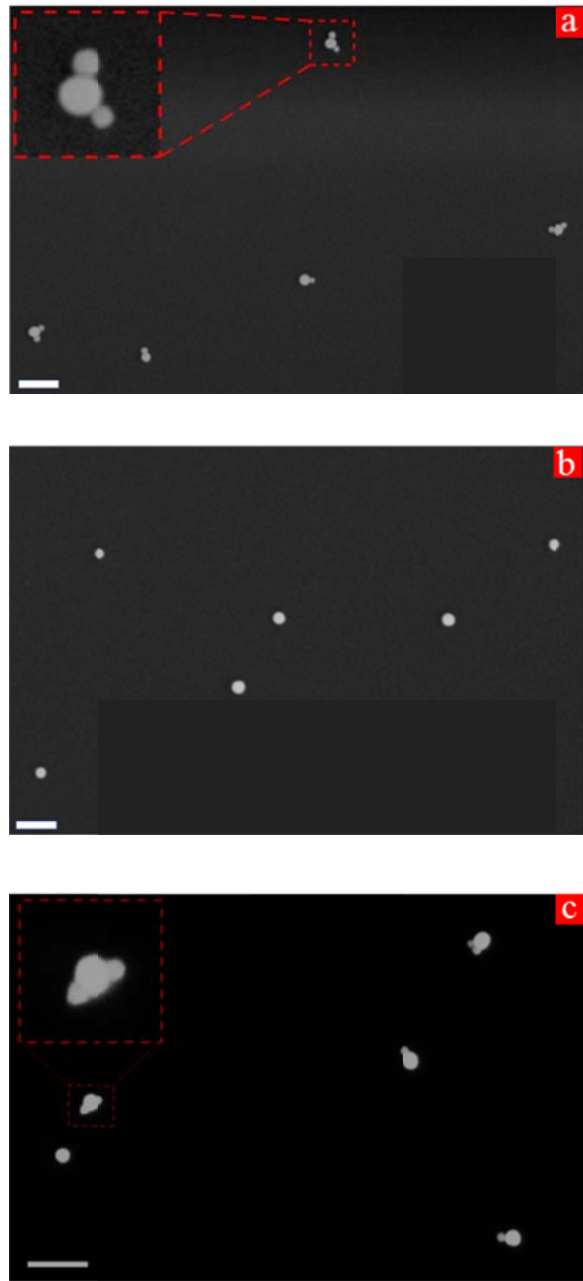
Figure 5-12 Formation of nanoparticle satellite conjugates onto silicon dioxide surface for 50 fM complementary (a) 50 fM 1-base pair mismatched (b), and 100 aM complementary (c) T-DNA (scale bars: 200nm)
