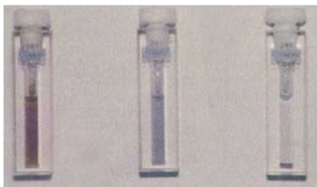
Figure 2-9 Red color DNA-AuNPs at 80 °C in unhybridized state (left), blue color at room temperature before DNA-AuNPs settlement to the bottom (center), and transparent at room temperature after settlement (right) [60].
