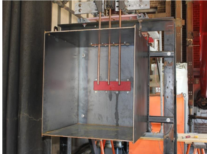
Figure 3- 6 Vertical electrodes in cubic enclosure arc flash tests
