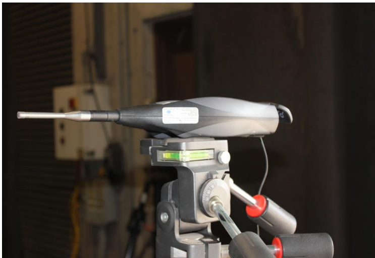
Figure 5- 37 Sound meter utilized in arc flash test
