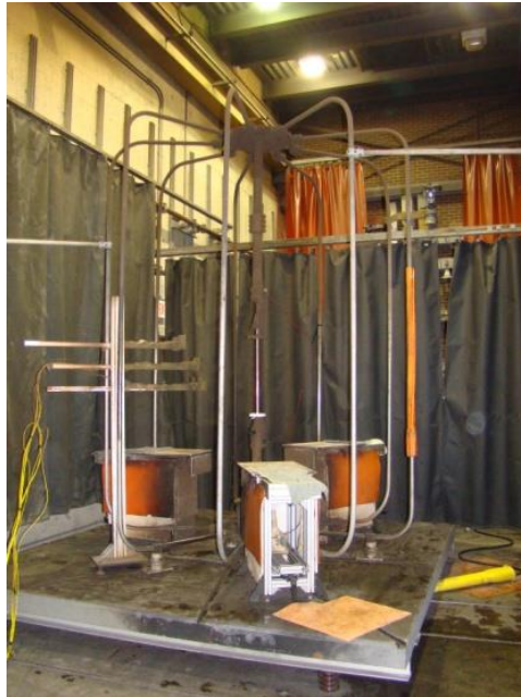
Figure 3- 1 Single phase arc flash test in Faraday Cage
