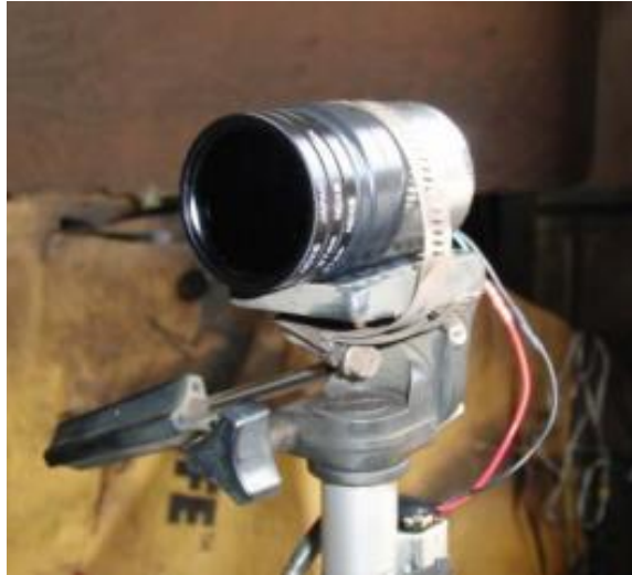
Figure 5- 12 Light measurement device with ND filter
