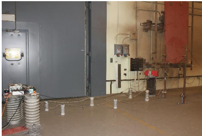
Figure 3- 20 Integrated measurement system with all protections (Top: Whole DAQ system with grounding and isolation design; Bottom: Isolated signal transmission bus)
