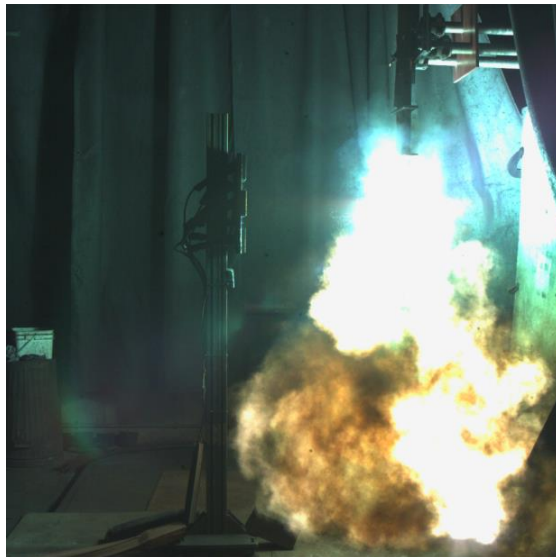
Figure 4- 13 Ejected arc plasma on vertical electrodes in open air
