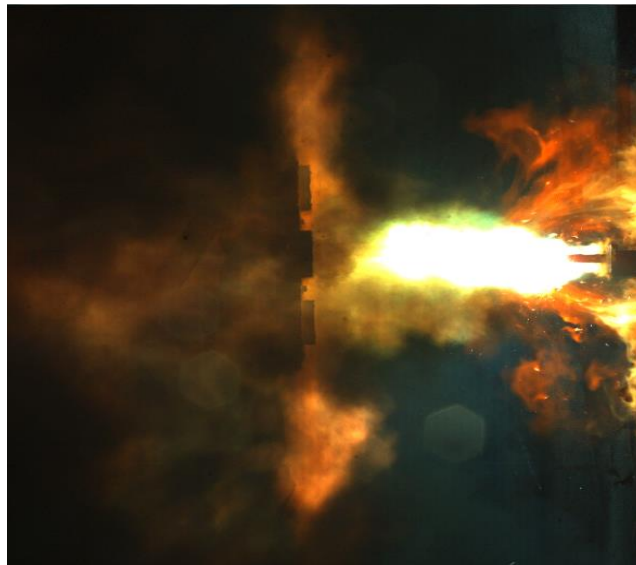
Figure 5- 19 Snap shot of arc flash from high speed video
