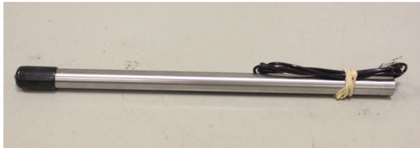
Figure 5- 28 LVDT working mechanism (upper) and typical LVDT device used in industry (lower).
