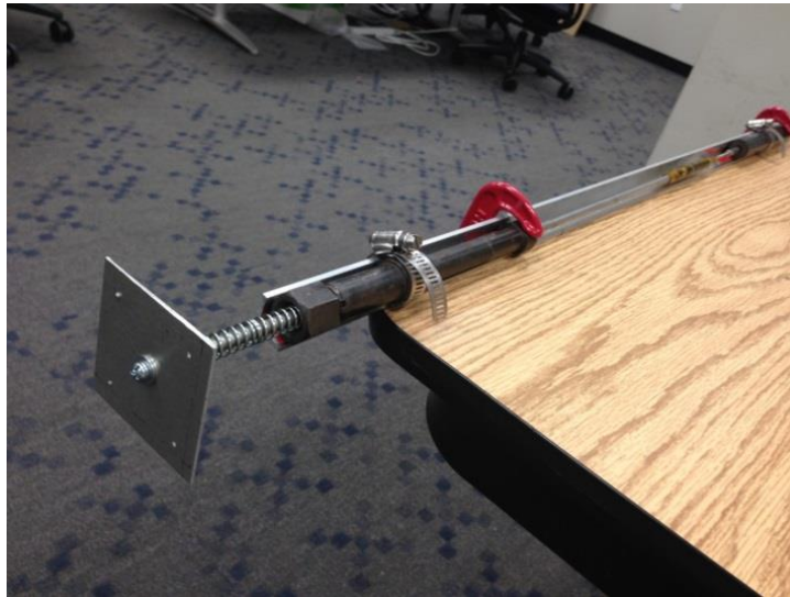
Figure 5- 30 LVDT pressure measurement system for arc flash test
