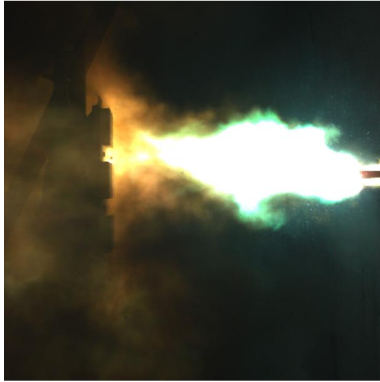
Figure 4- 12 Ejected arc plasma on horizontal electrodes in open air
