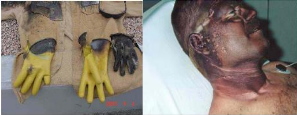
Figure 1- 2 Arc flash burning on equipment and personnel [3]
