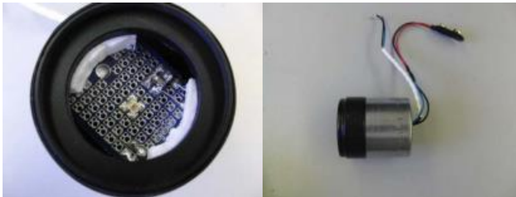
Figure 5- 13 Light measurement device without ND filter
