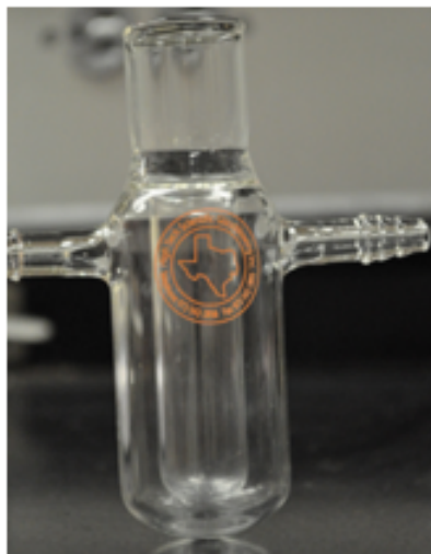
Figure 2.2: Custom Pyrex ® glass cell built by High Tech Scientific Glassblowing Inc. The inner glass tube (8 mm) was joined to an outer tube (48 mm) which allows for cooling of the reaction mixture. This glass cell filters UV light < 320 nm.
