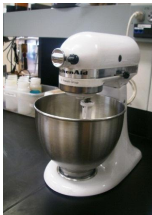
Fig 3.1 Kitchen aid mixer used for blending of greases in the TLCL lab at UTA
