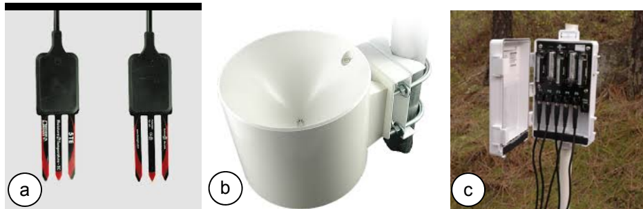
Figure 3. 13: 5TM Temp/moist. sensor, 100ECRN rain gauge and Em-50G data logger
