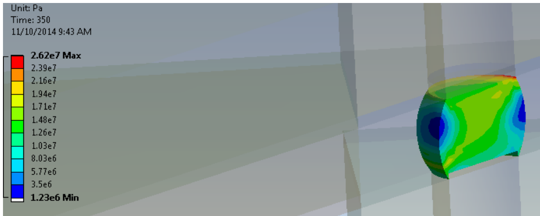
Figure 3-34 Compact model - von-Mises stress (mold E = 5GPa)
