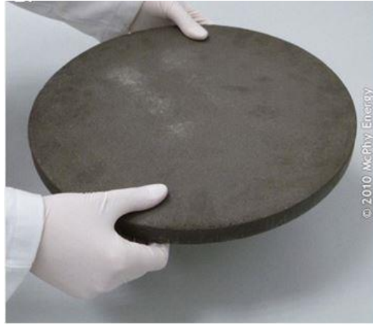
Figure 1.4 McPhy composite (based on magnesium hydride)
