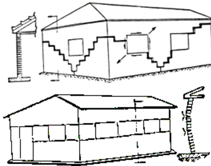
Figure 2-4 Damages in building due to subsoil movement (Kalantari, 2012)
