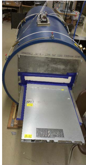
Figure 3-14 HP SE1102 mounted on an airflow bench
