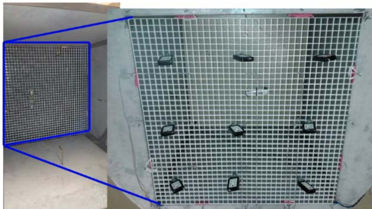
Figure 3-17 Humidity-temperature sensors mounted on a plastic egg crate light diffuser in the upstream duct (Figure adapted, with permission, [54] © 2015 IEEE)
