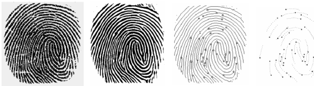
Figure 2-19 Fingerprint image thinning and minutiae extraction process [8]
