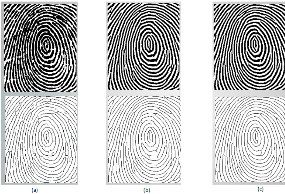
Figure 5-21 Thinning operation on (a) Original FVC2004DB2 101 fingerprint image (b) State of the art enhancement (c) Multi-stage enhancement
