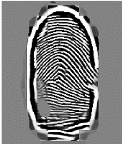
Figure 5-7 Proposed LPD based two-stage scheme enhancement of the bad image
