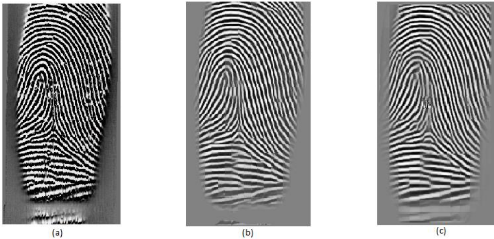
Figure 5-19 (a) Original FVC2004DB3 105 fingerprint image (b) State of the art enhancement (c) Multi-stage enhancement
