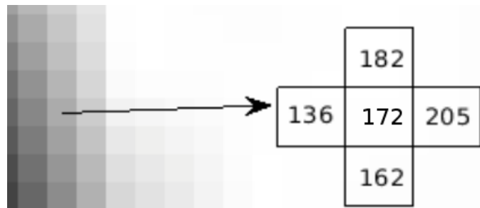
Figure 3.9. An example of pixels that contribute in the value of a specific pixel gradients.
