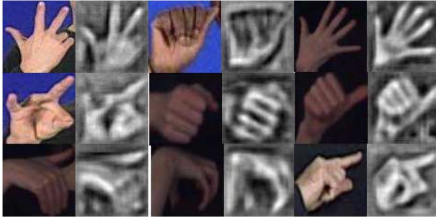
Figure 2.1: Hand shape sample images from the ASL data set. The color images are the annotated hand regions in the color frame. The grayscale images are the corresponding visualizations of extracted HoG features using inverse HoG [27].
