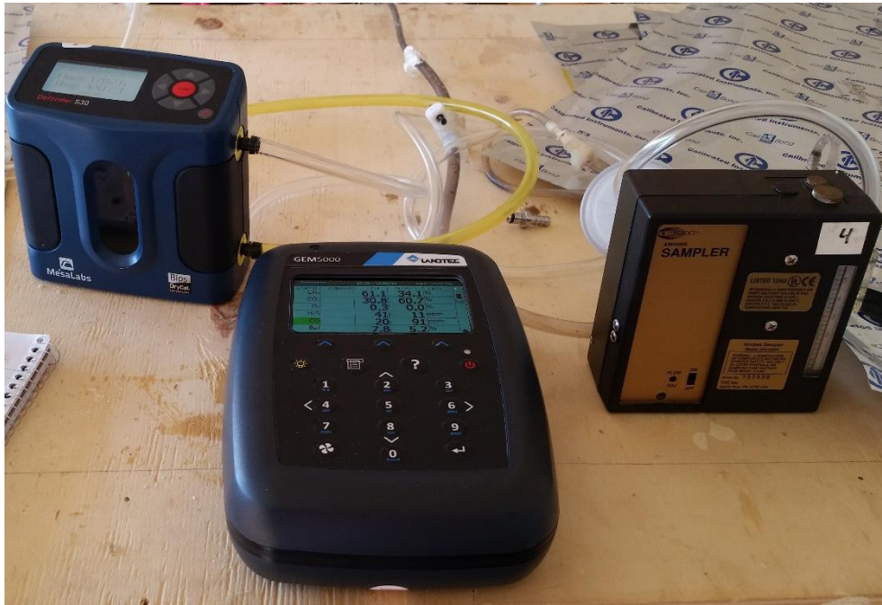
Figure 3-13 Gas composition measurement instrument Landtec GEM 5000 (middle) and volume measurement instruments, Calibrator (Left) & SKC Sampler (Right)
