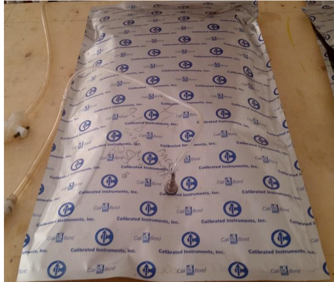
Figure 3-3 Gas-bag used to collect the generated biogas
