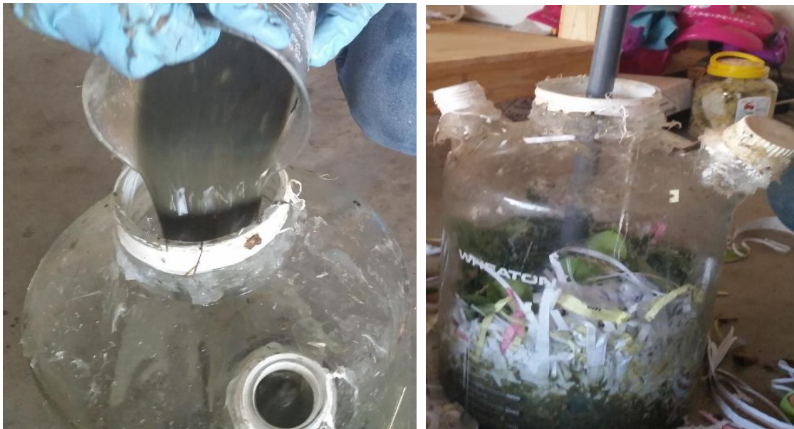
Figure 3- 10 (a) Reactor inoculated with microbe's seed (b) loading of selected waste mixture
