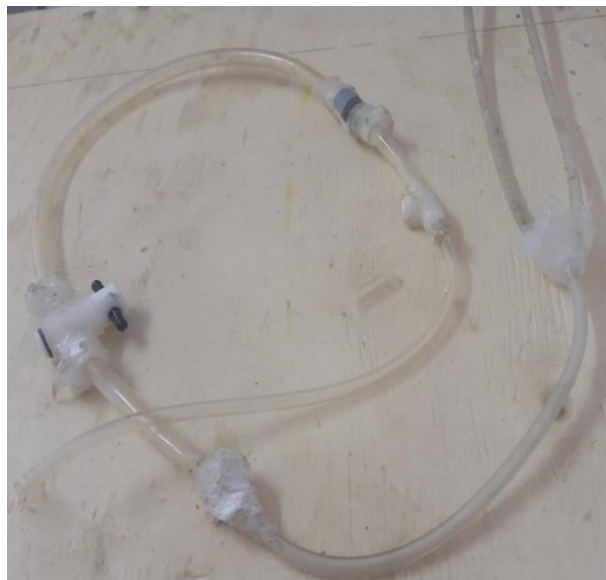
Figure 3-2 Tygon tubes with two-way valve
