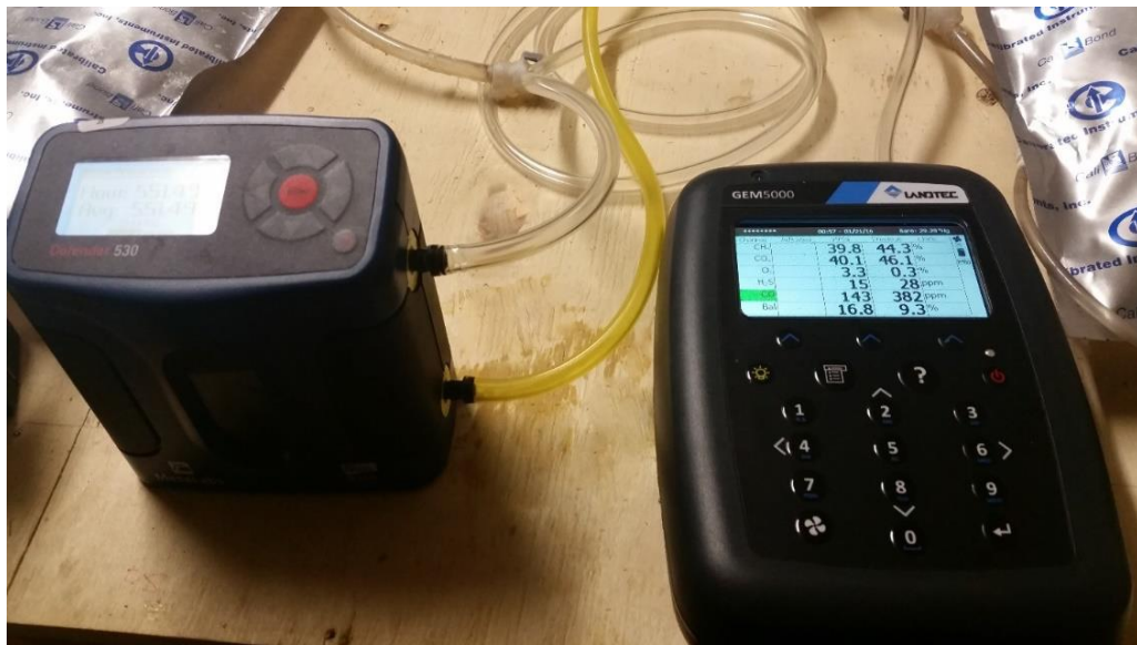
Figure 3-15 Gas flow measurement while measuring the gas composition
