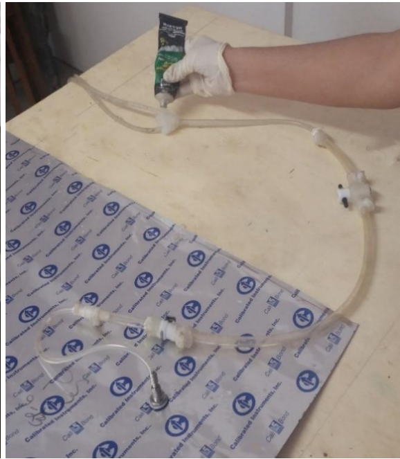
(c) Using sealant at the T-joint of a delivery tube
