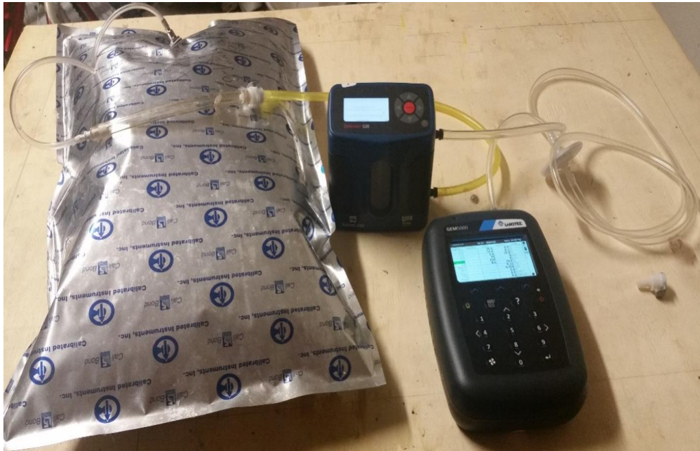
Figure 3- 14 Process of measuring gas composition
