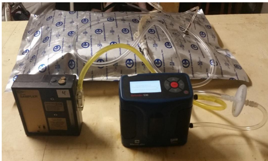
Figure 3- 18 Volume of gas is measured by using SKC sampler and calibrator
