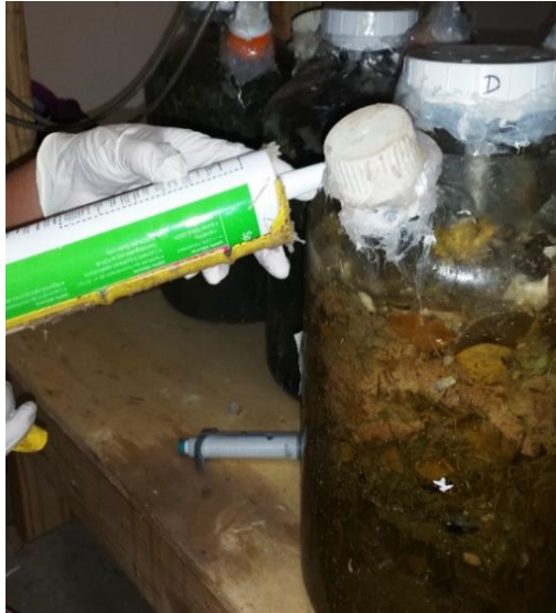
(c) Resealing the cap of reactor
