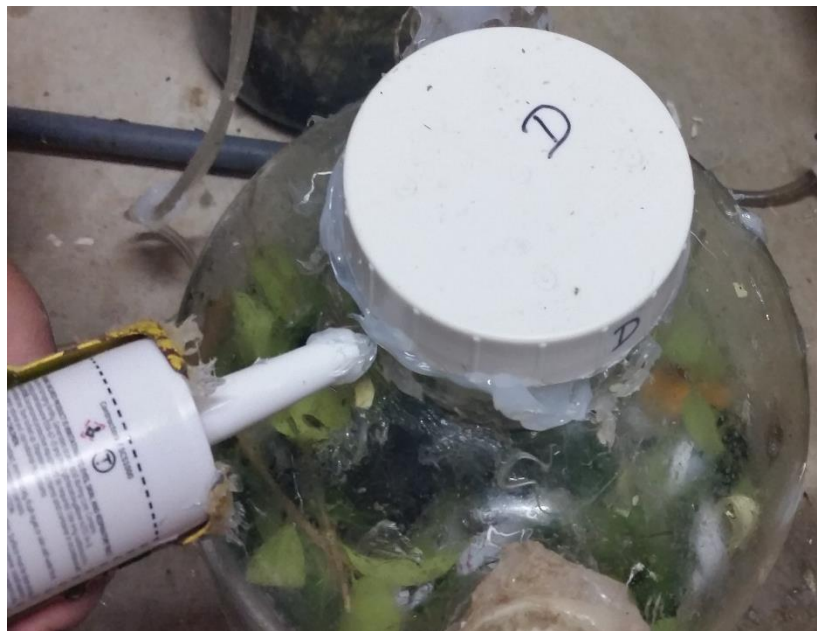
Figure 3- 11 (a) Applying transparent sealant to the reactors
