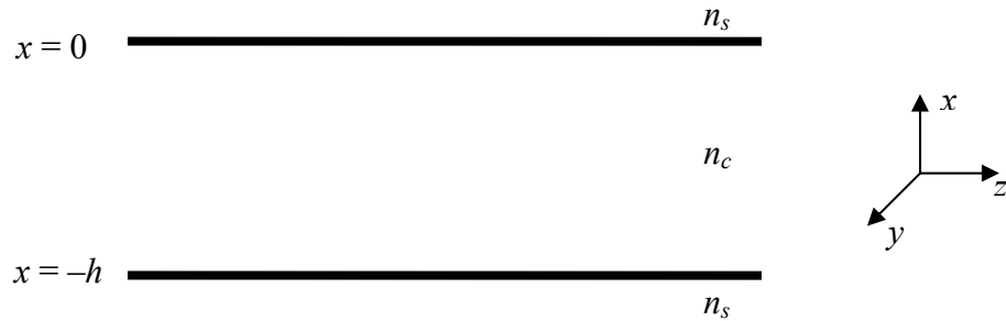
Figure 2-1. A side cross-section of a simple slab waveguide, where a higher refractive index material n_c is surrounded by two lower refractive indices of n_s .
